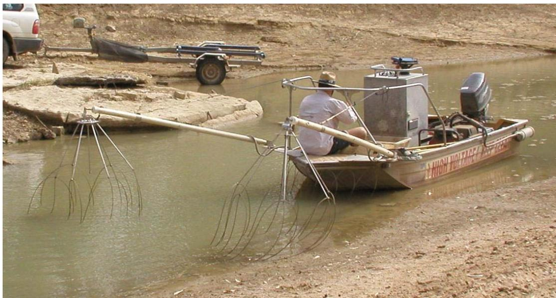
**Plate 1** Boat electrofisher in operational mode, with anodes extended.
