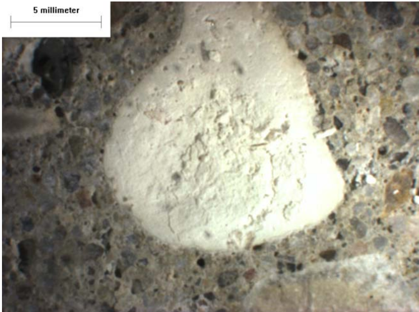
Figure 34. A 10-mm aggregate particle showing first signs of damage after soaking in potassium acetate and then exposure to eight cycles of freezing and thawing in water.
