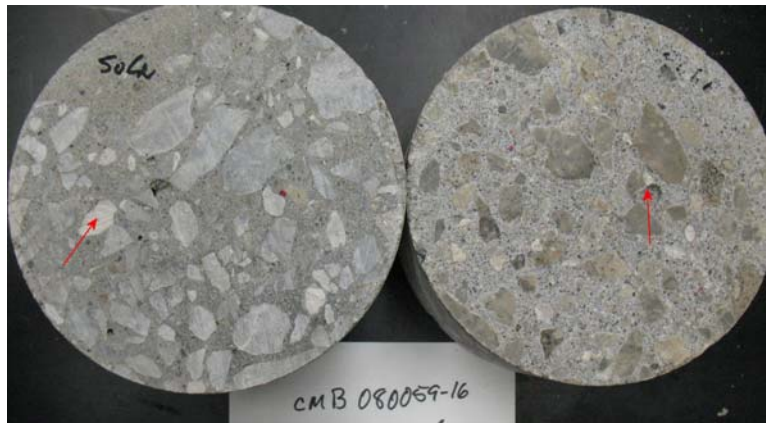
Figure 41. Sample from Core 16. Control is on the left, KAc-exposed is on the right. Red arrows indicate a damaged aggregate particle.
