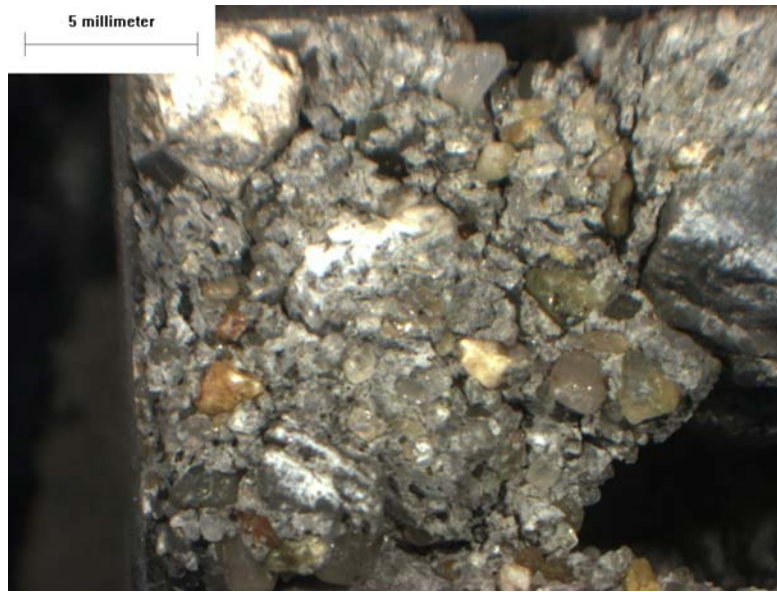
Figure 22. Paste damage in sample 27 after 81 cycles of freezing and thawing.
