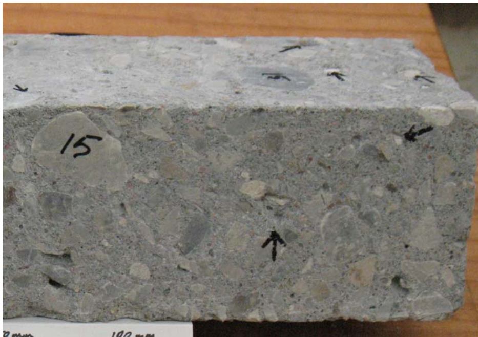
Figure 20. Cement paste fraction of sample 15 after 125 cycles of freezing and thawing. Corners are relatively sharp and paste etching is minimal.
