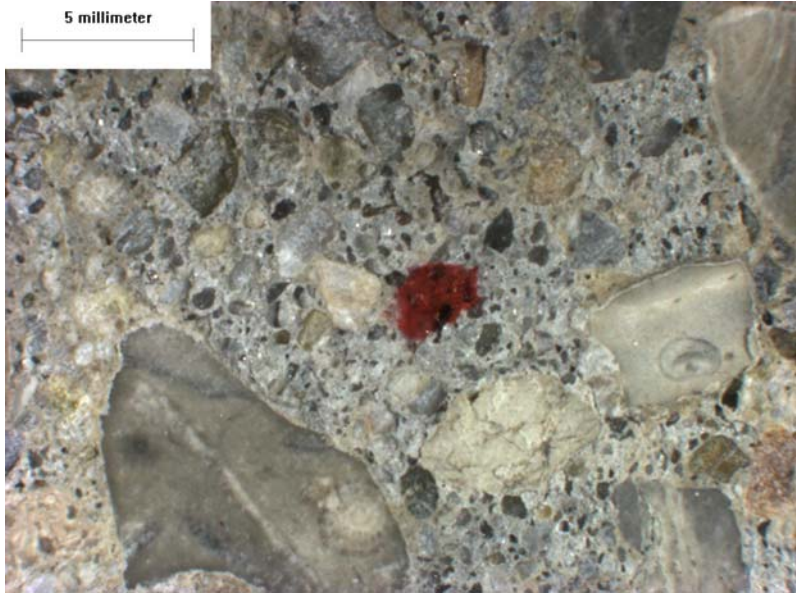
Figure 35. Mortar fraction of Core 16 after soaking in potassium acetate and then exposed to eight cycles of freezing and thawing, showing exposure of aggregate particles due to erosion of paste.
