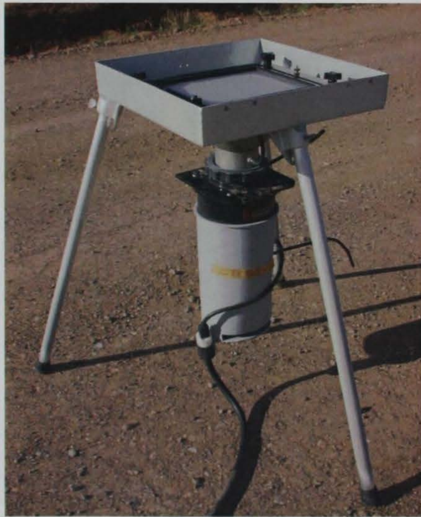
Photo 24. Stationary dust collectors used to monitor palliative effectiveness
