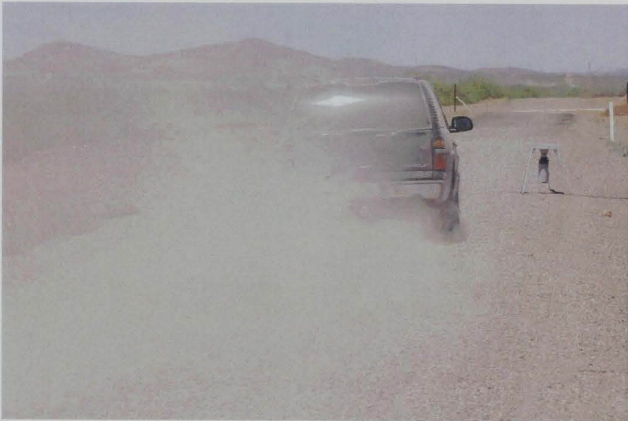
Photo 52. Very heavy dust on untreated control section during testing
