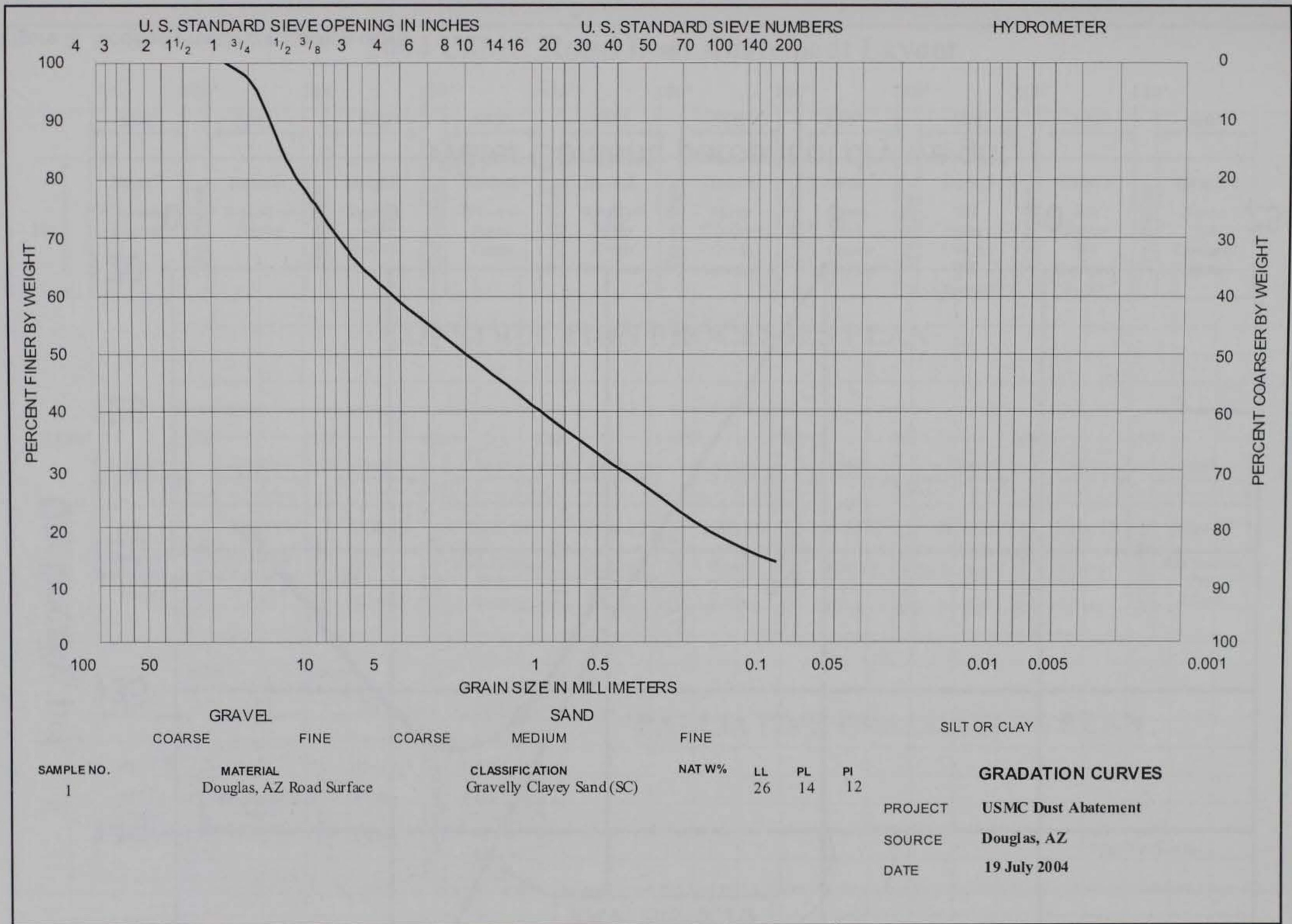
Figure 1. Soil gradation curve
