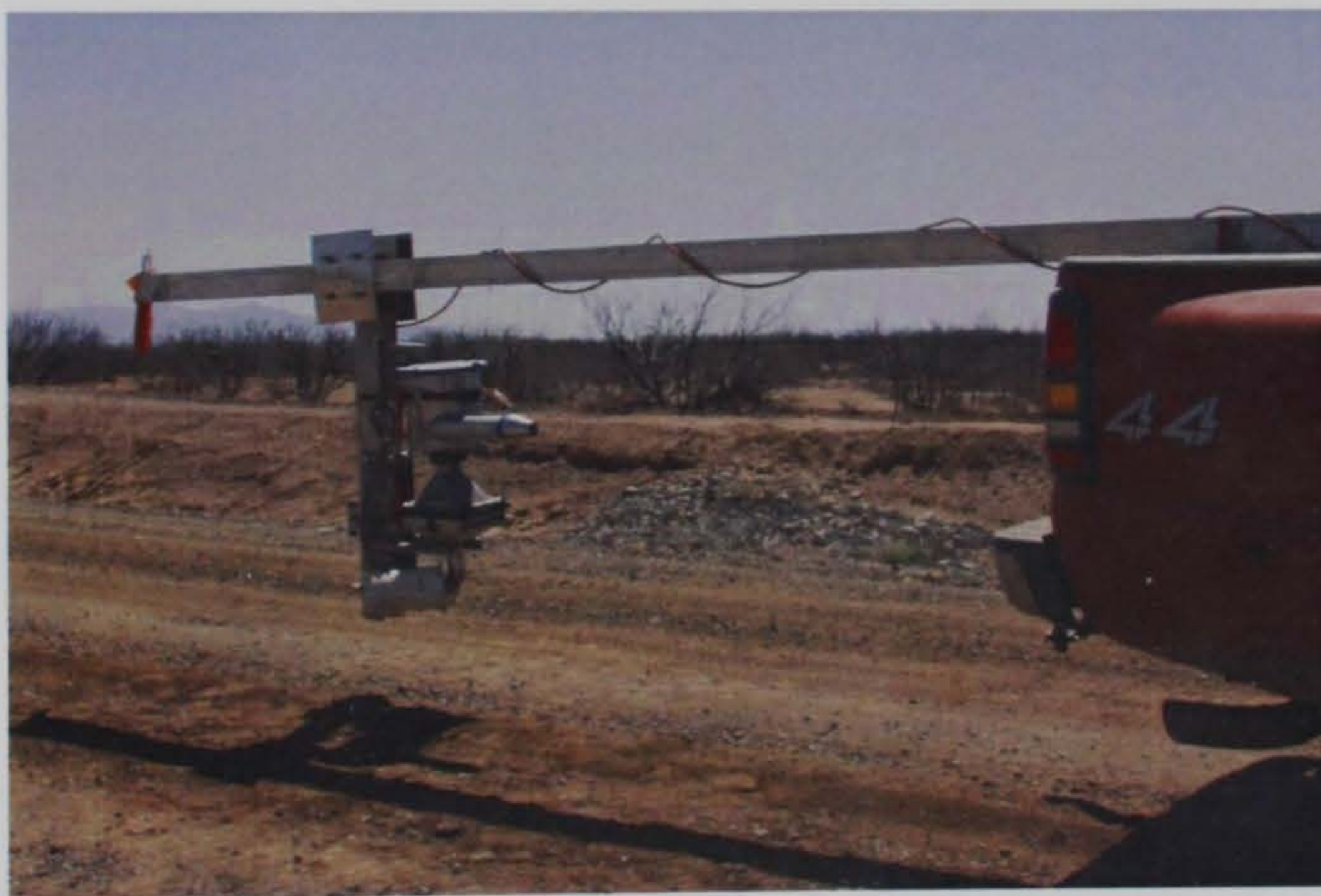
Photo 26. Tow-behind dust collection system used by MRI
