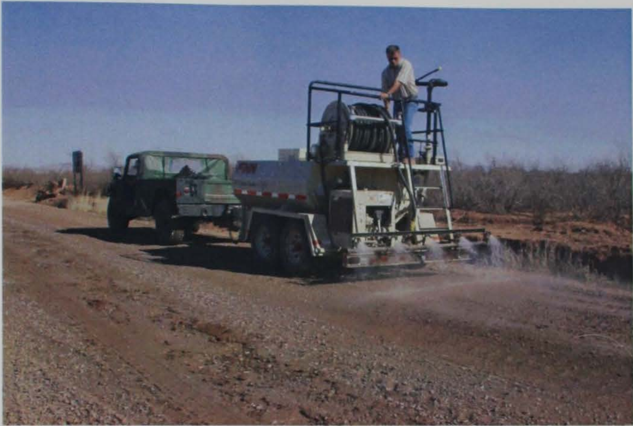
Photo 5. Finn T-90 hydroseeder pulled by HMMWV
