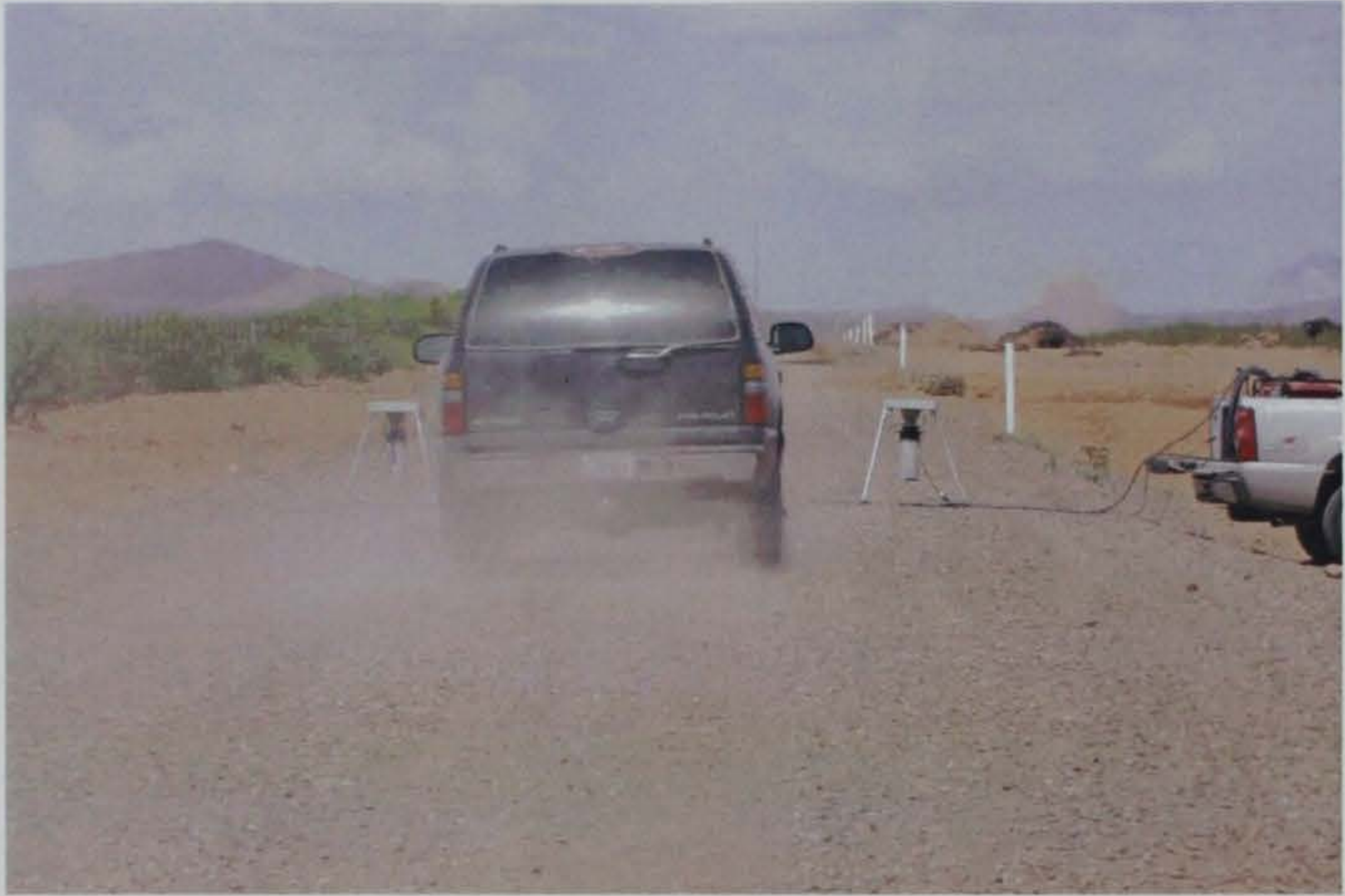
Photo 47. Moderate dust produced during testing on Secion 20, Soil-Sement®
