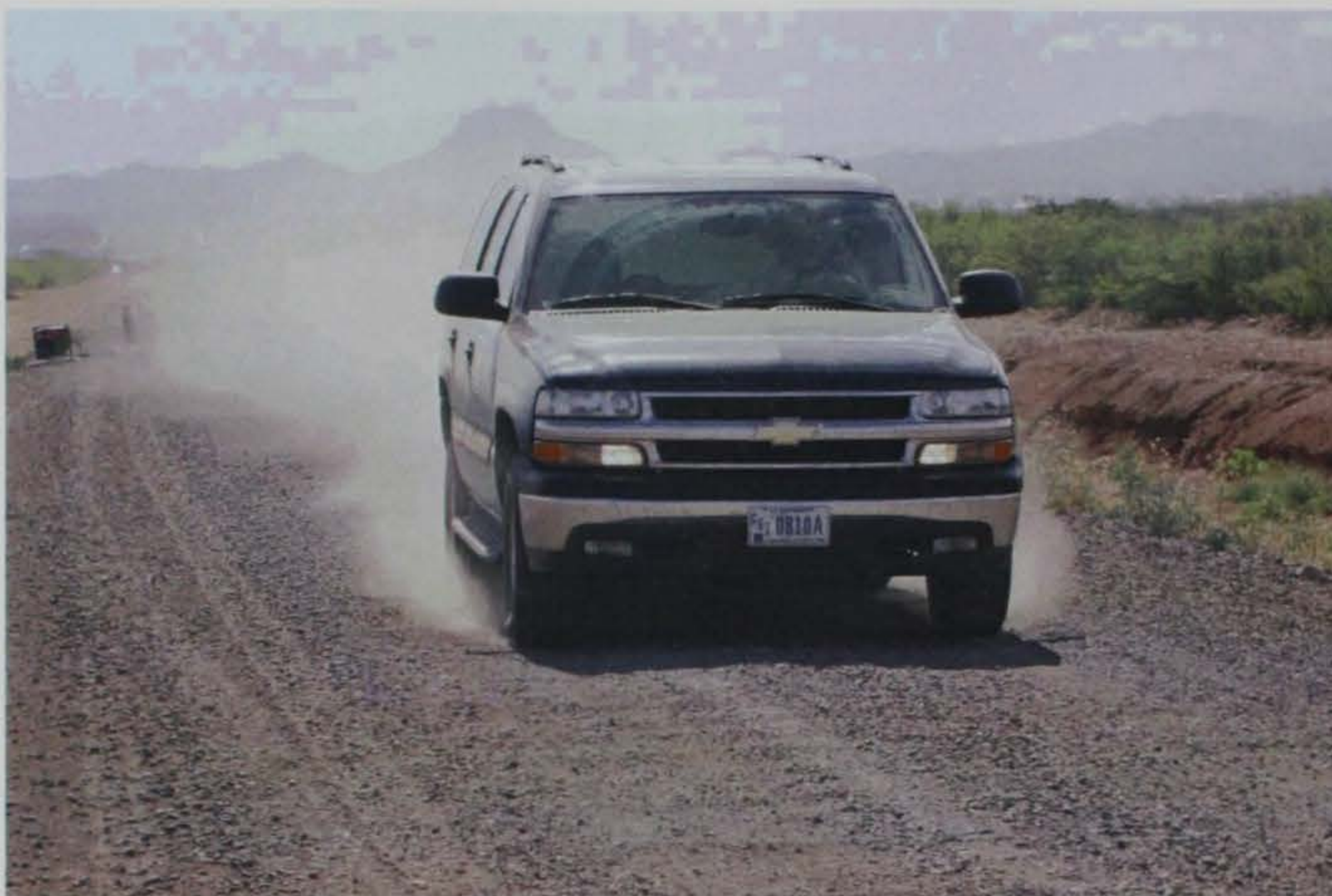
Photo 43. Blinding dust and corrugation on Section 15, Road Oyl®
