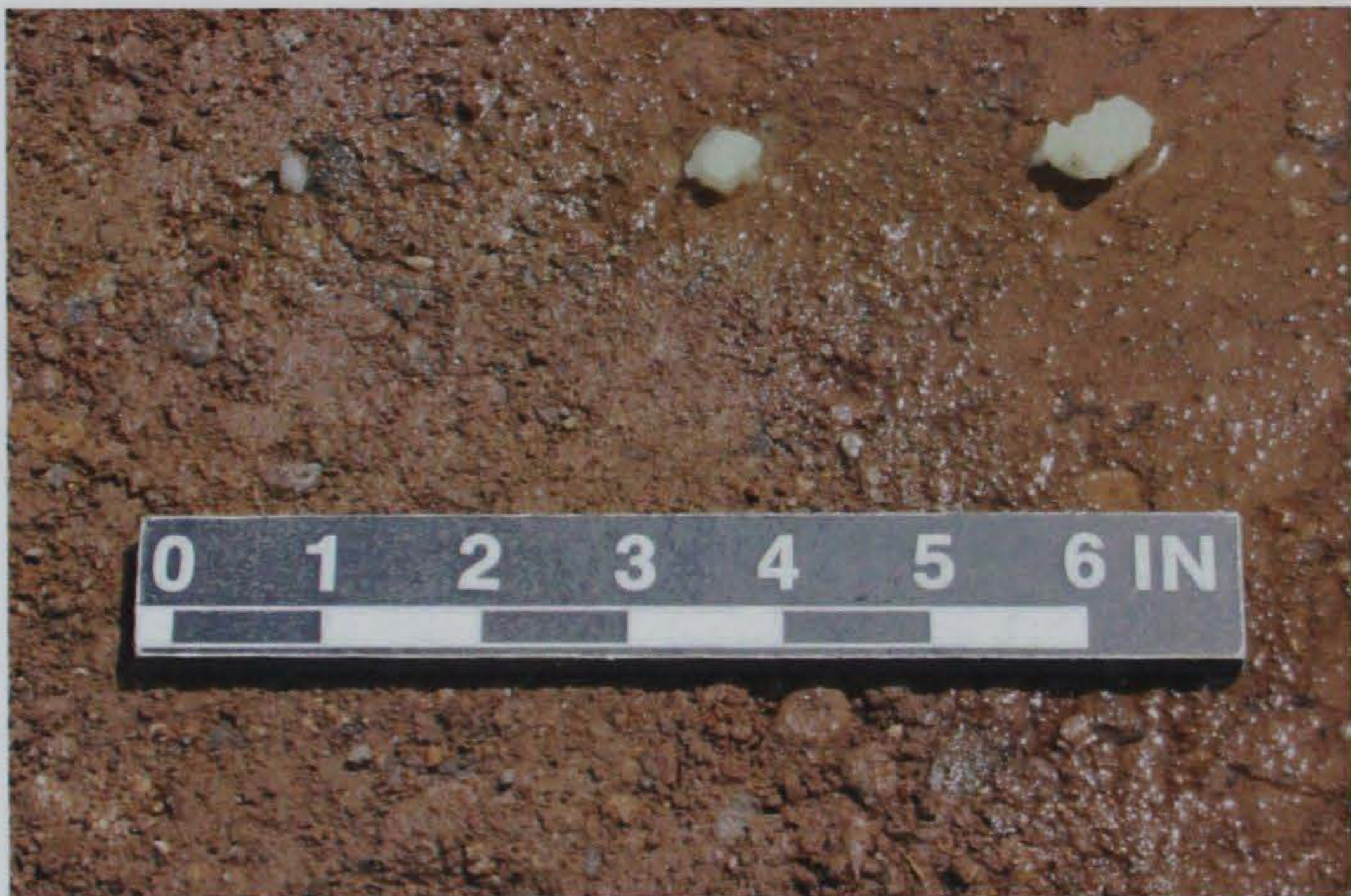
Photo 32. Balls of undissolved Hydrostik® sprayed from hydroseeder
