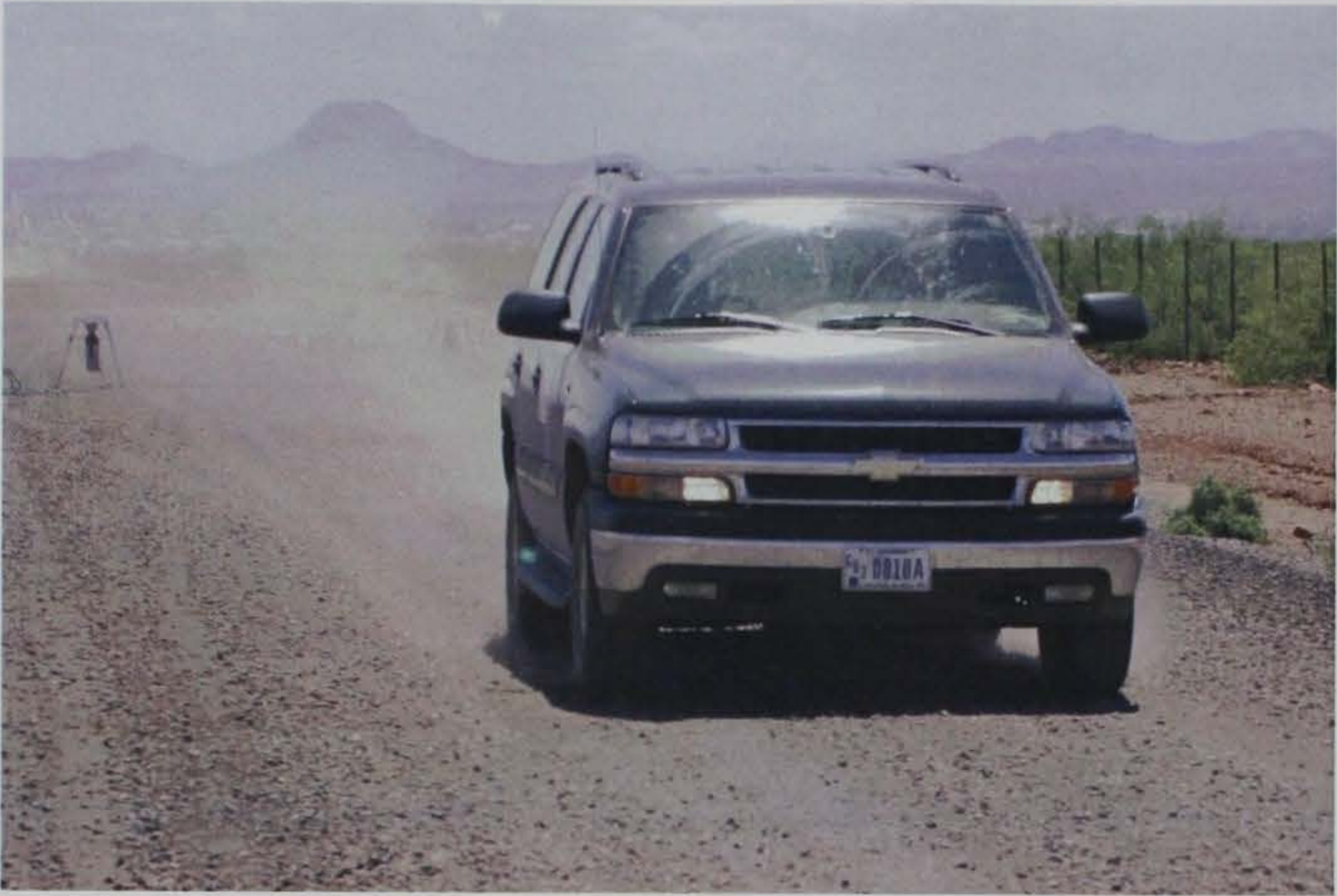
Photo 51. Reduced visibility behind vehicle on Section 23, CSS-1
