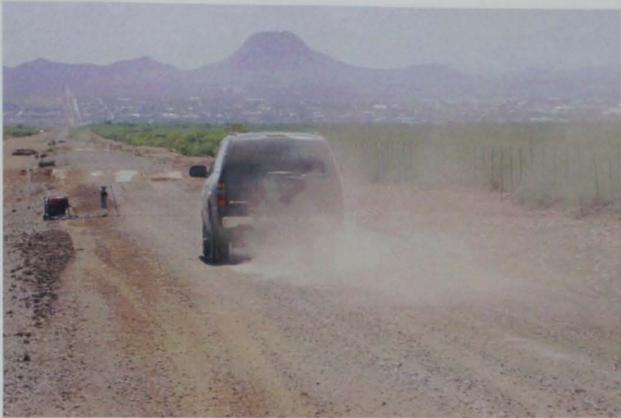
Photo 49. Heavy dust during traffic on Section 21, EK-35®
