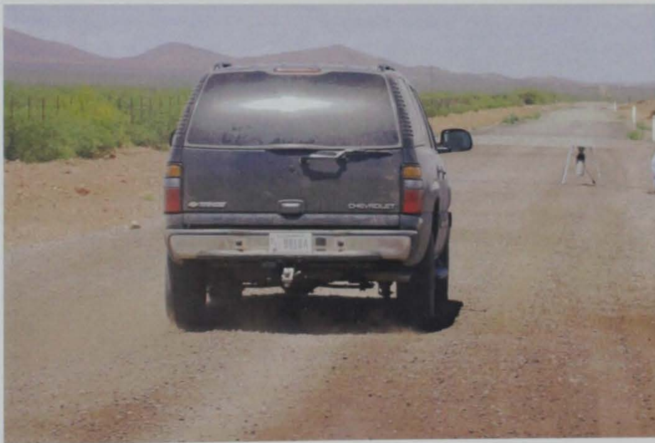
Photo 50. Light dust behind vehicle traffic on Section 22, Envirokleen®
