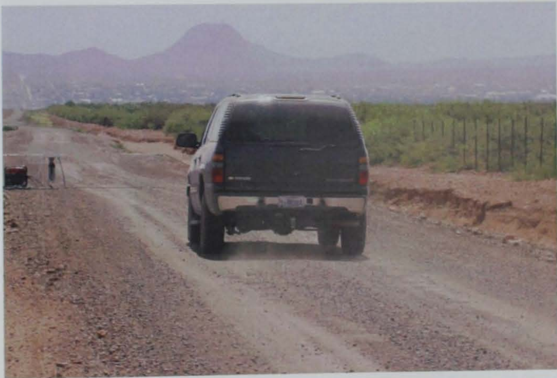
Photo 46. Good dust abatement on Section 19, Soiltac®
