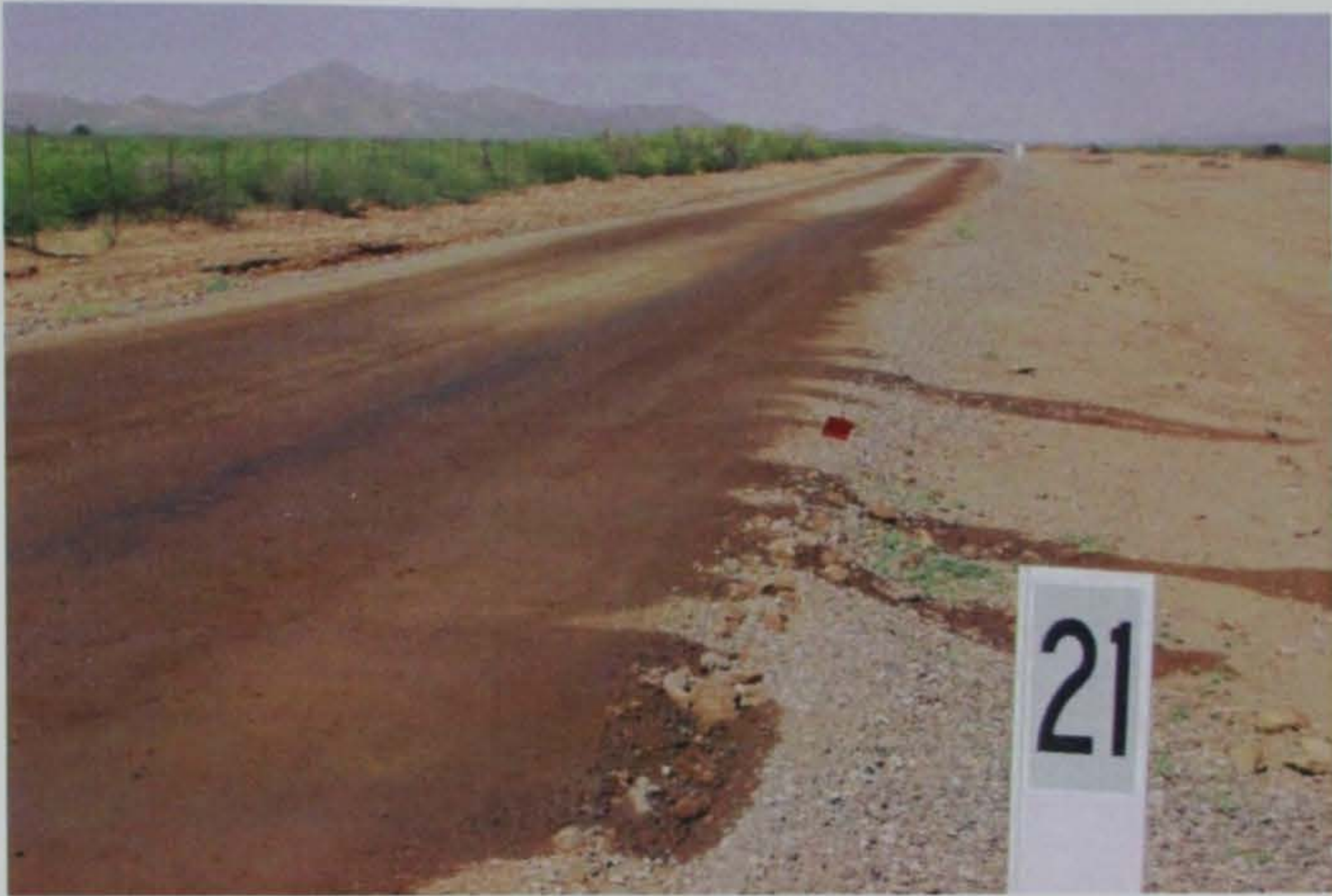
Photo 37. Uneven product distribution on Section 21 after 30 days
