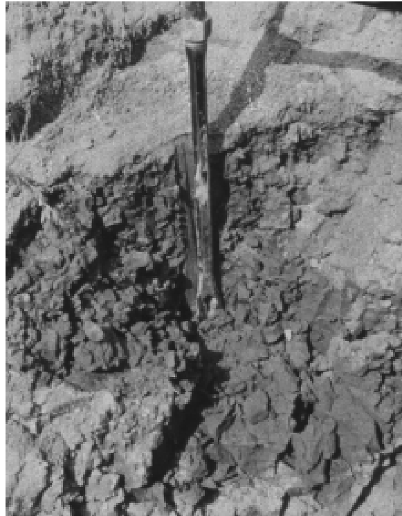
Figure 12. Test pit showing blocky soil structure caused by freeze-thaw cracking—Valley Trail test pad.
