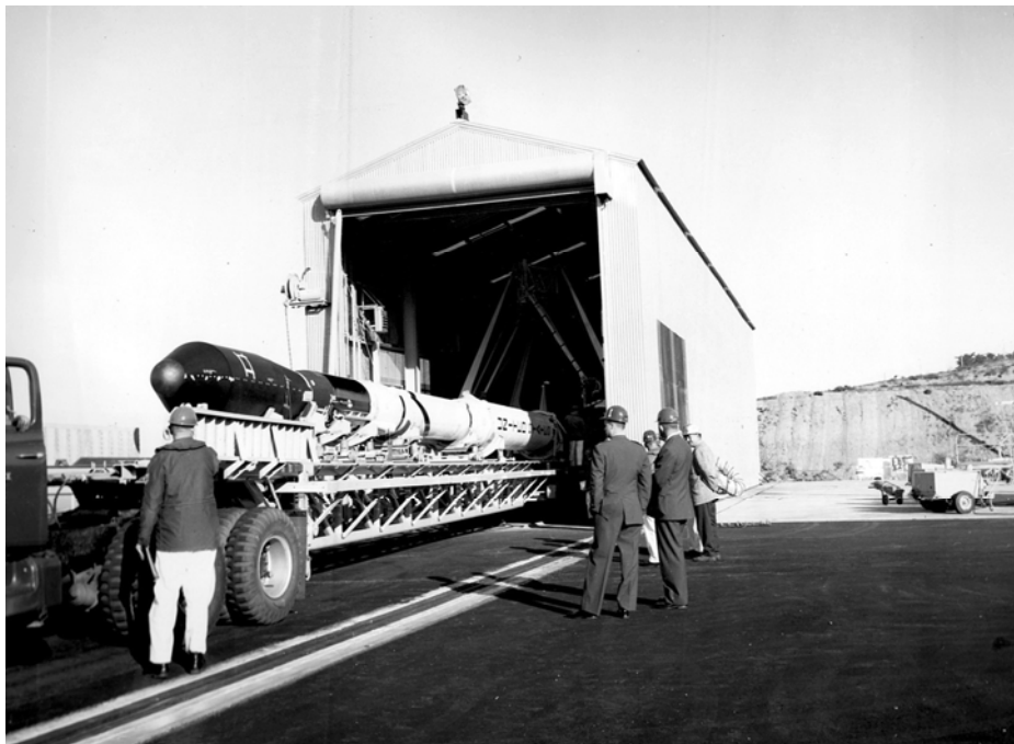
Figure 35. Scout vehicle and transporter being placed inside mobile shelter, 1963 (NARA, College Park, MD).
