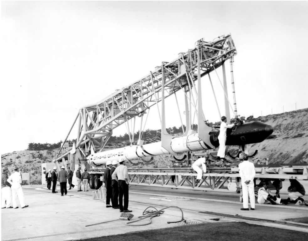
Figure 41. Scout vehicle positioned in launcher with shelter removed, 1963 (NARA, College Park, MD).
