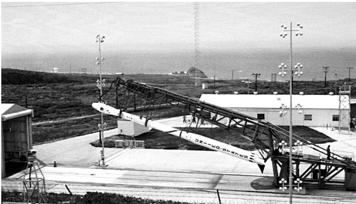
Figure 42. Scout vehicle being raised in launcher for flight, n.d. (Official NASA-USAF Photograph).
