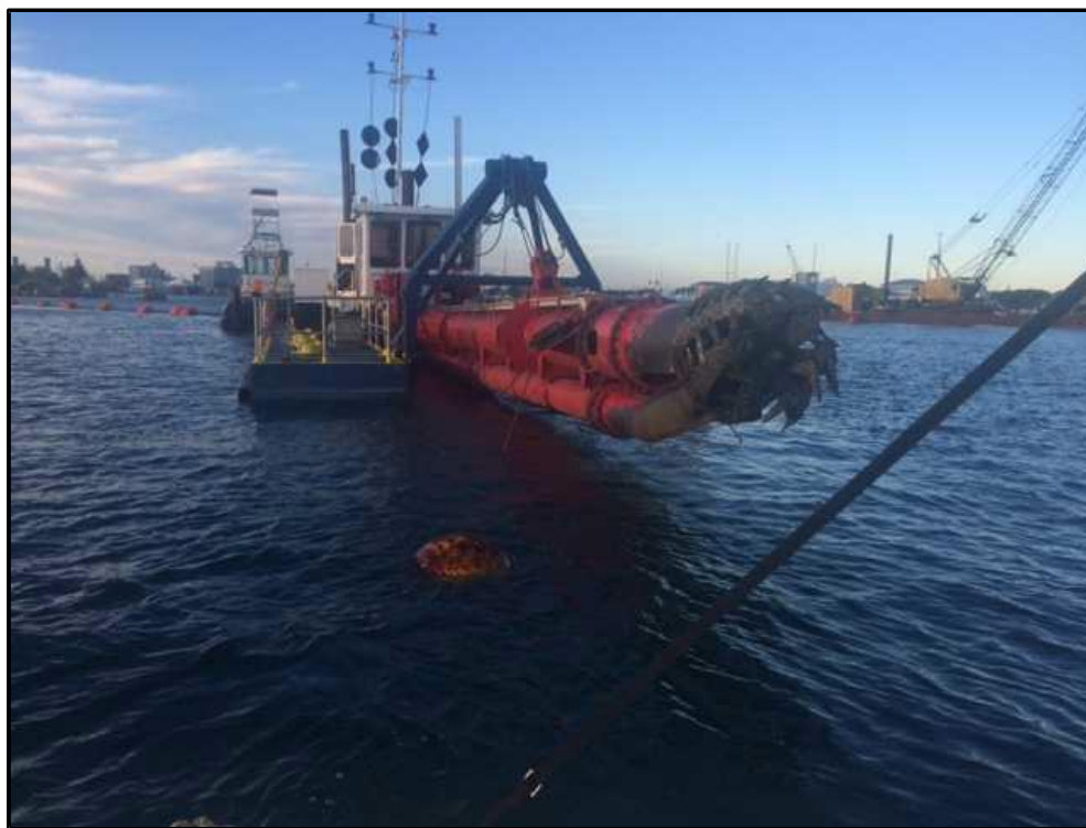
Photograph No. 1 – Dredge Equipment with Cutterhead
