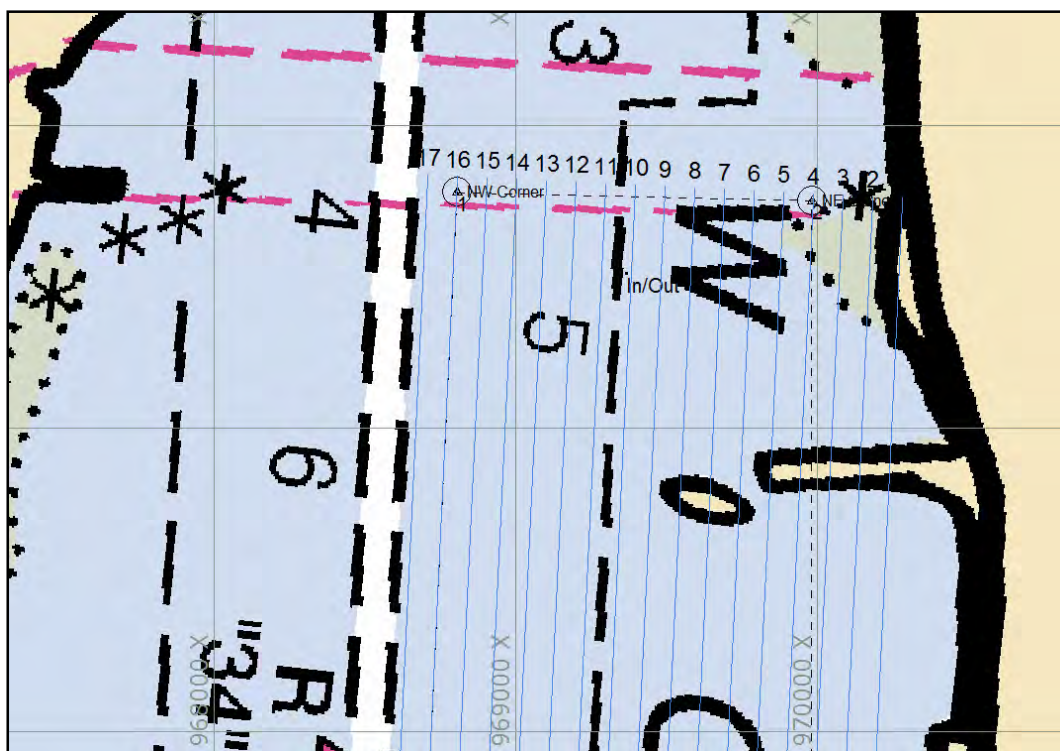
Figure 2. Chart showing the cable or pipeline crossing at the northern border of the survey area and channel stabilization jetties west of the manmade land that extend into the survey area from the east shore of Lake Worth.
