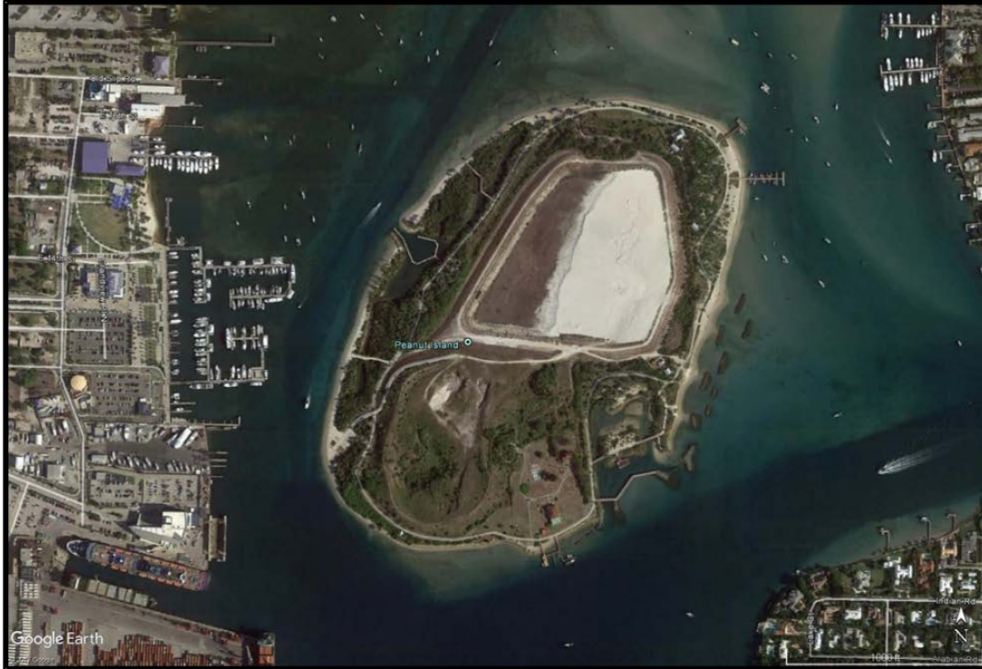
Figure 2. Peanut Island Dredged Material Management Area. Fill material will be mined from upland and loaded onto barges located at the deep-water access loading/offloading facility on the western shore (©2017 Google Earth).
