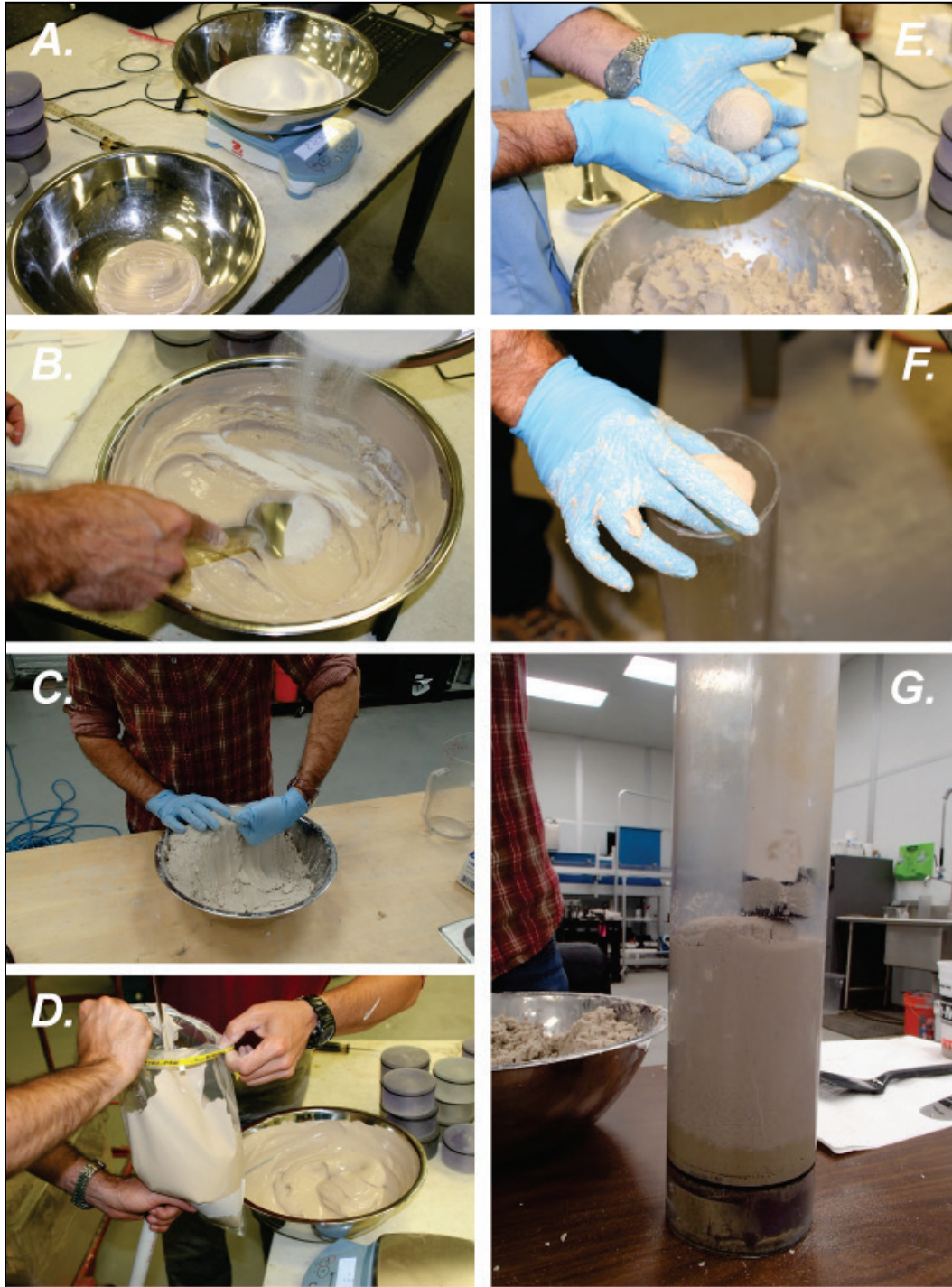
Figure 6. Photos depicting the mixing of sand and mud are presented in A – C. Photos demonstrating the methods utilized to place material in core tubes are presented in D – G.
