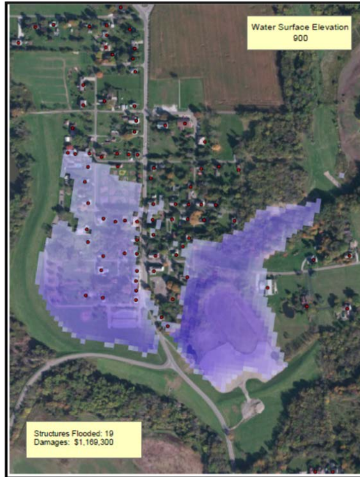
Figure 3-23 Extent of water at El. 900.
