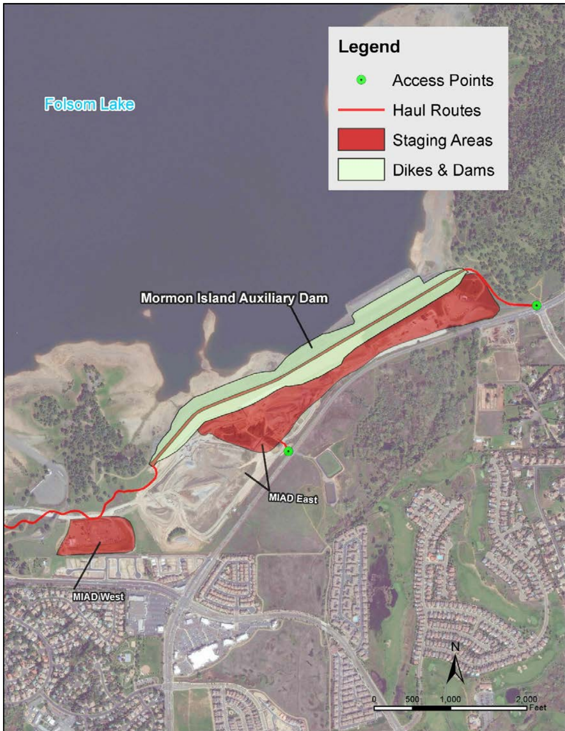
Figure 2-14. Haul routes, access points, and staging areas for the raising of Mormon Island Auxiliary Dam (MIAD) , as well as for the raising of Dikes 7 and 8 (one of the earthen raise elements).
