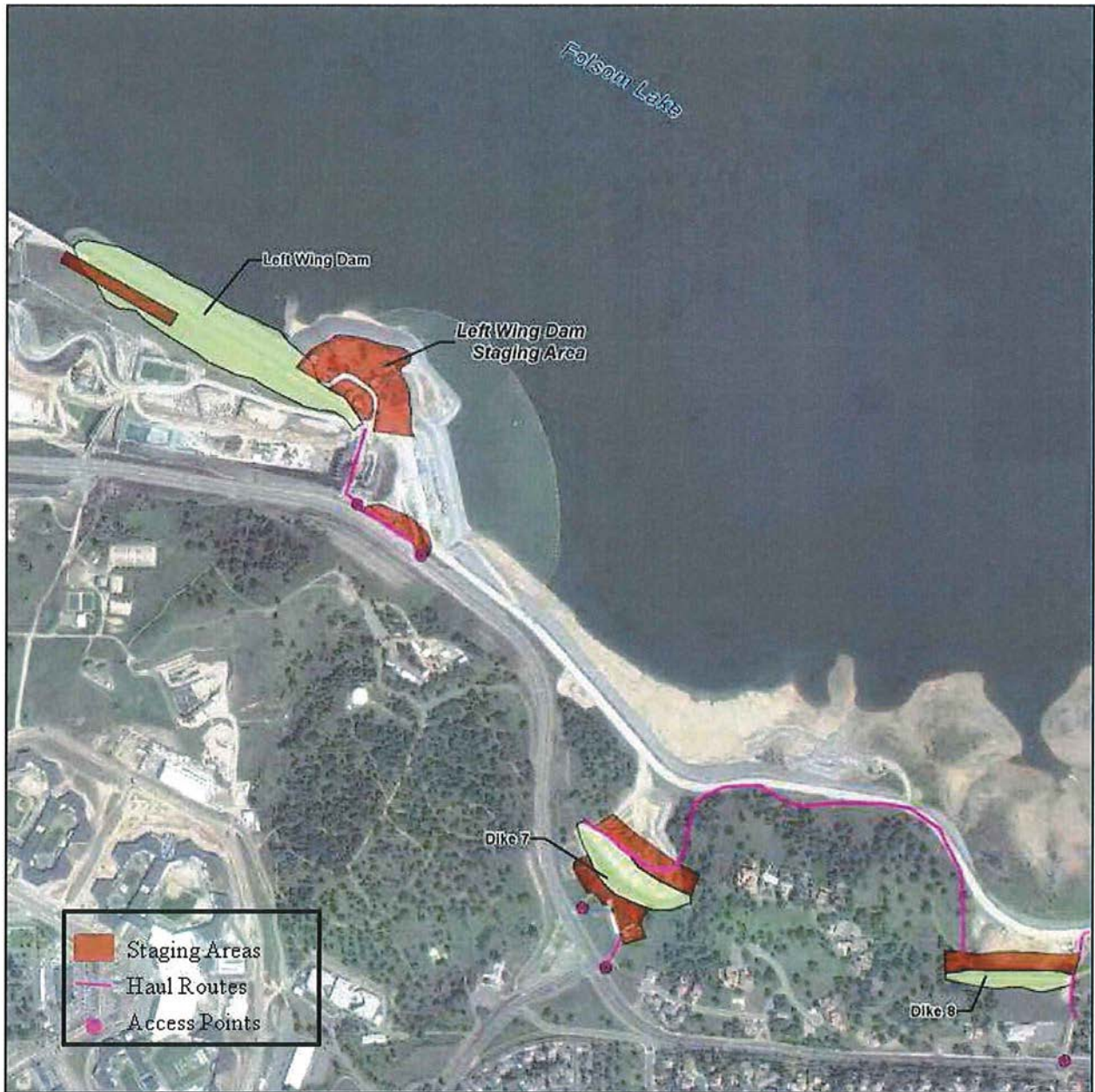
Figure 10. Staging areas, access points, and haul roads associated with Dikes 7 and 8, as well as the Left Wing Dam.
