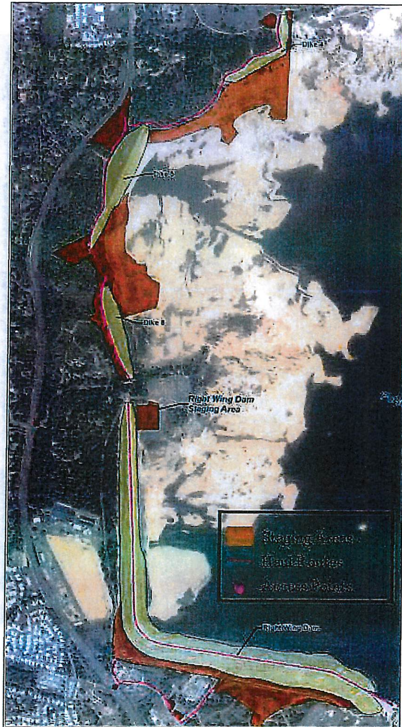
Figure 9. Staging areas, access points, and haul roads associated with Dikes 4, 5, and 6, as well as Right Wing Dam.
