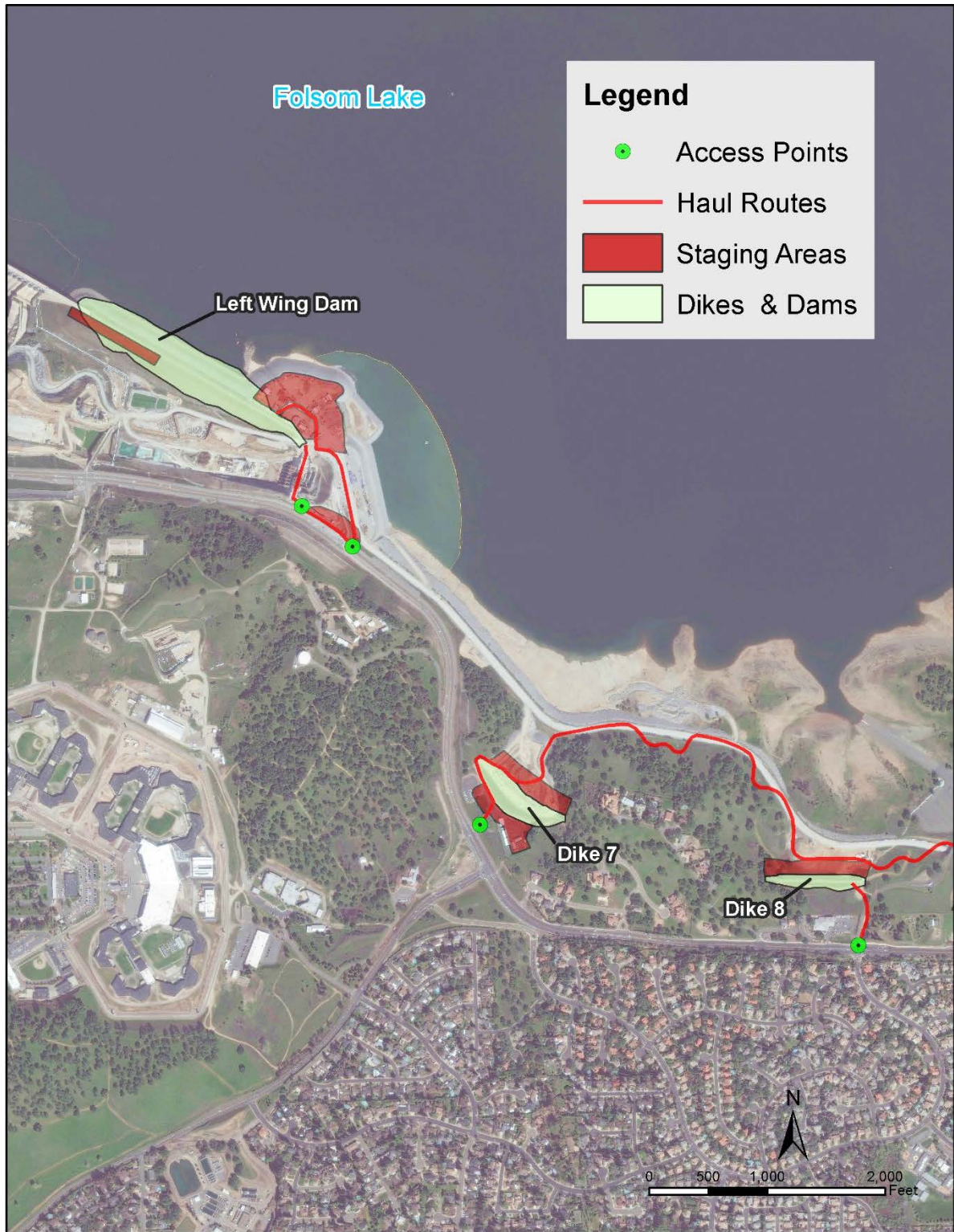
Figure 2-12. Haul routes, access points, and staging areas for the Left Wing Dam (LWD) floodwall construction work (one of the concrete floodwall elements) and for the raising of Dikes 7 and 8 and MIAD (one of the earthen raise elements).
