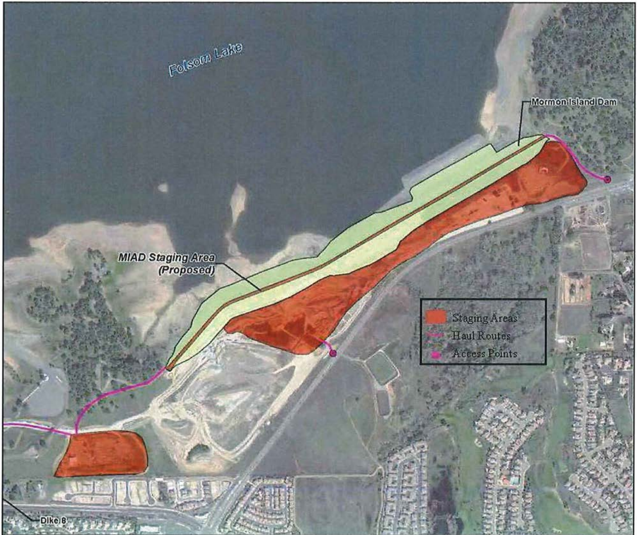
Figure 11. Staging areas, access points, and haul roads associated with Mormon Island Auxiliary Dam (MIAD).
