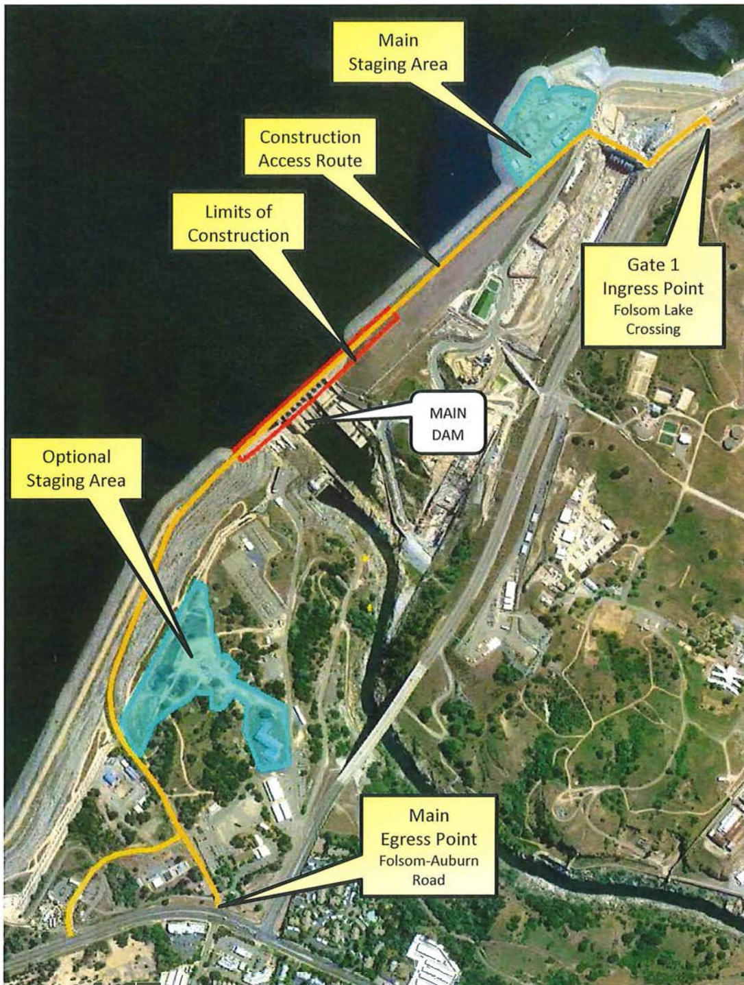
Figure 2. Main dam tainter gate refinements: Limits of construction (red lines), construction staging areas (blue lines), and construction access route (orange lines).
