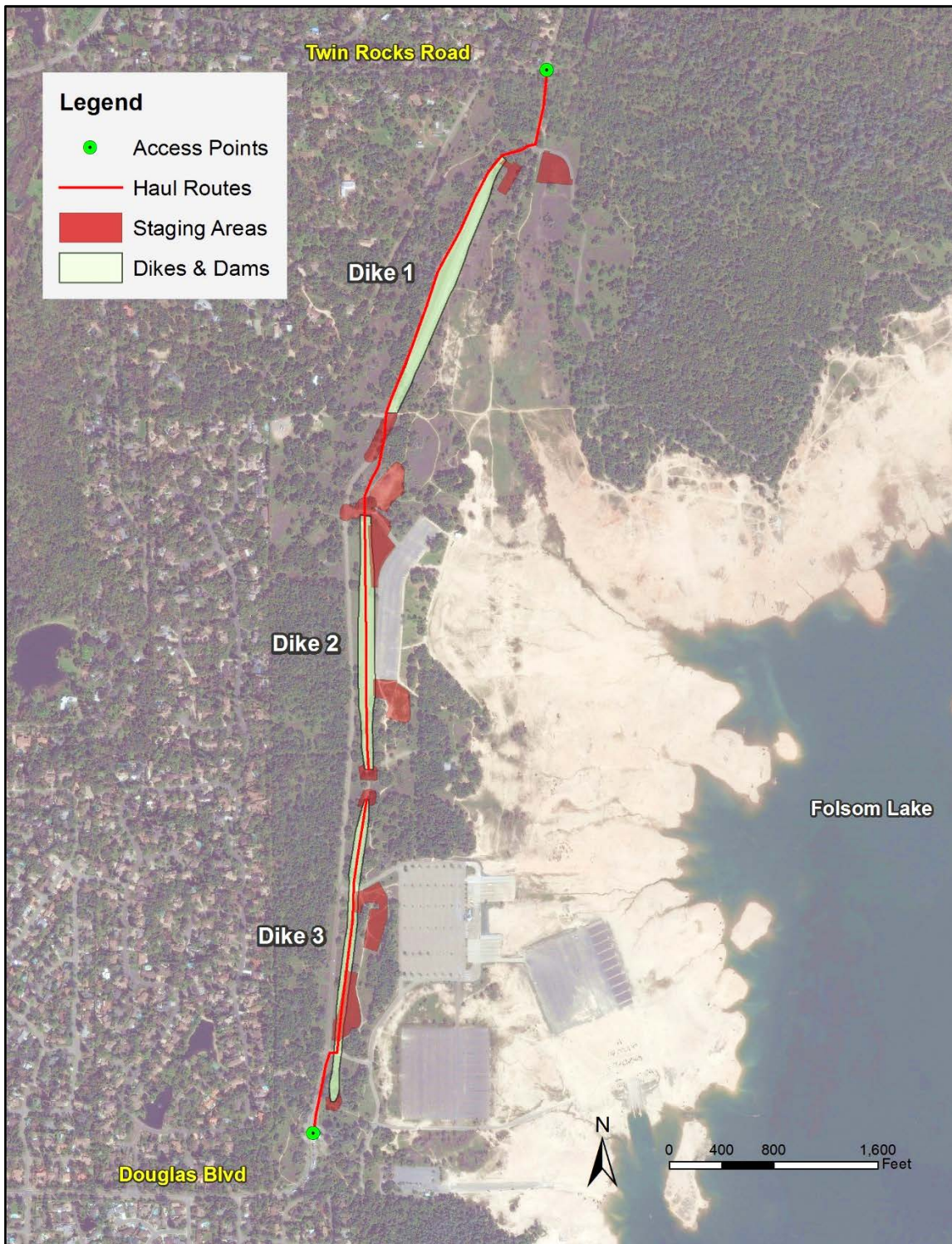
Figure 2-13. Haul routes, access points, and staging areas for the raising of Dikes 1, 2, and 3 (one of the earthen raise elements).
