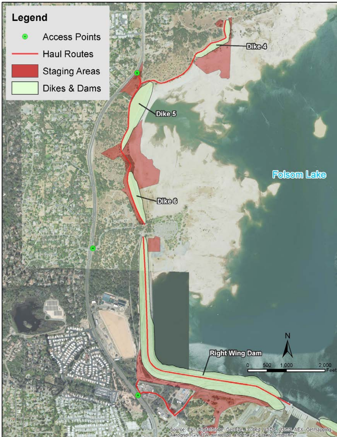
Figure 2-11. Haul routes, access points, and staging areas for the Right Wing Dam (RWD) floodwall construction work (one of the concrete floodwall elements) and for the raising of Dikes 4, 5, and 6 (one of the earthen raise elements).
