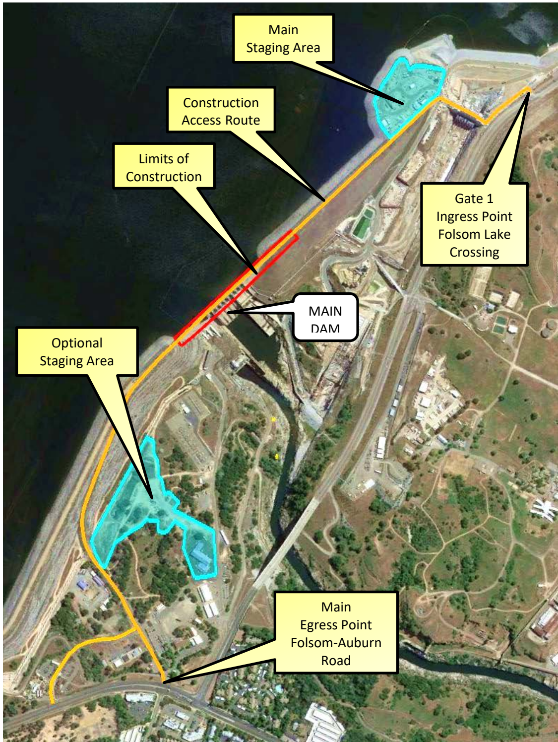
Figure 2-10. Main dam Tainter gate refinements: Limits of construction (red lines), construction staging areas (blue lines), and construction access route (orange lines).
