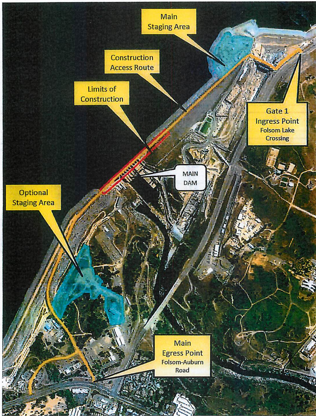
Figure 2. Main dam tainter gate refinements: Limits of construction (red lines), construction staging areas (blue lines), and construction access route (orange lines).
