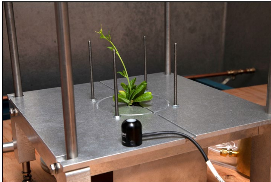
Figure 3. Mature (flowering) A. thaliana plant inserted in the guillotine base of the plant chamber, which isolates the vegetative components to the chamber, separating soil volatiles from plant volatiles. Also note the light sensor in the foreground.
