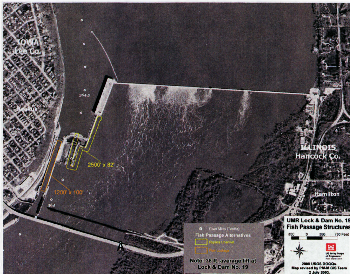
Figure D20. Potential fish passage improvements at Lock and Dam 19, Upper Mississippi River
