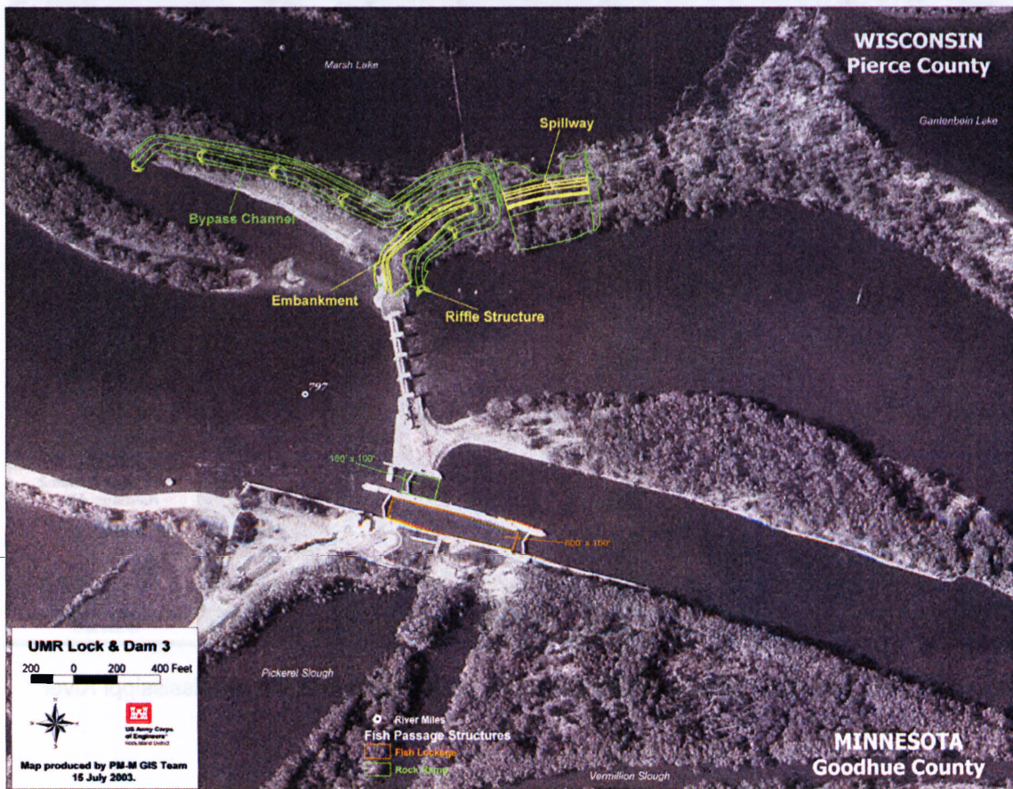
Figure D3. Potential fish passage improvements at Lock and Dam 3, Upper Mississippi River
