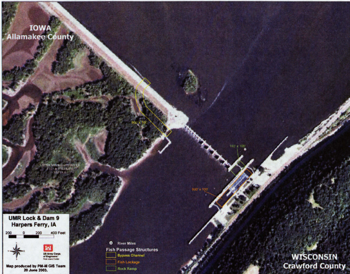
Figure D10. Potential fish passage improvements at Lock and Dam 9, Upper Mississippi River
