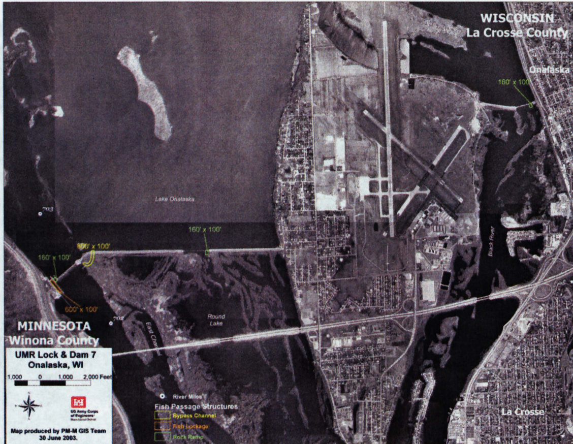
Figure D8. Potential fish passage improvements at Lock and Dam 7, Upper Mississippi River.
