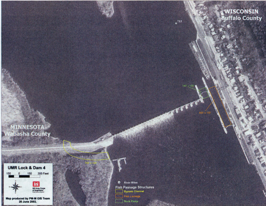
Figure D4. Potential fish passage improvements at Lock and Dam 4, Upper Mississippi River
