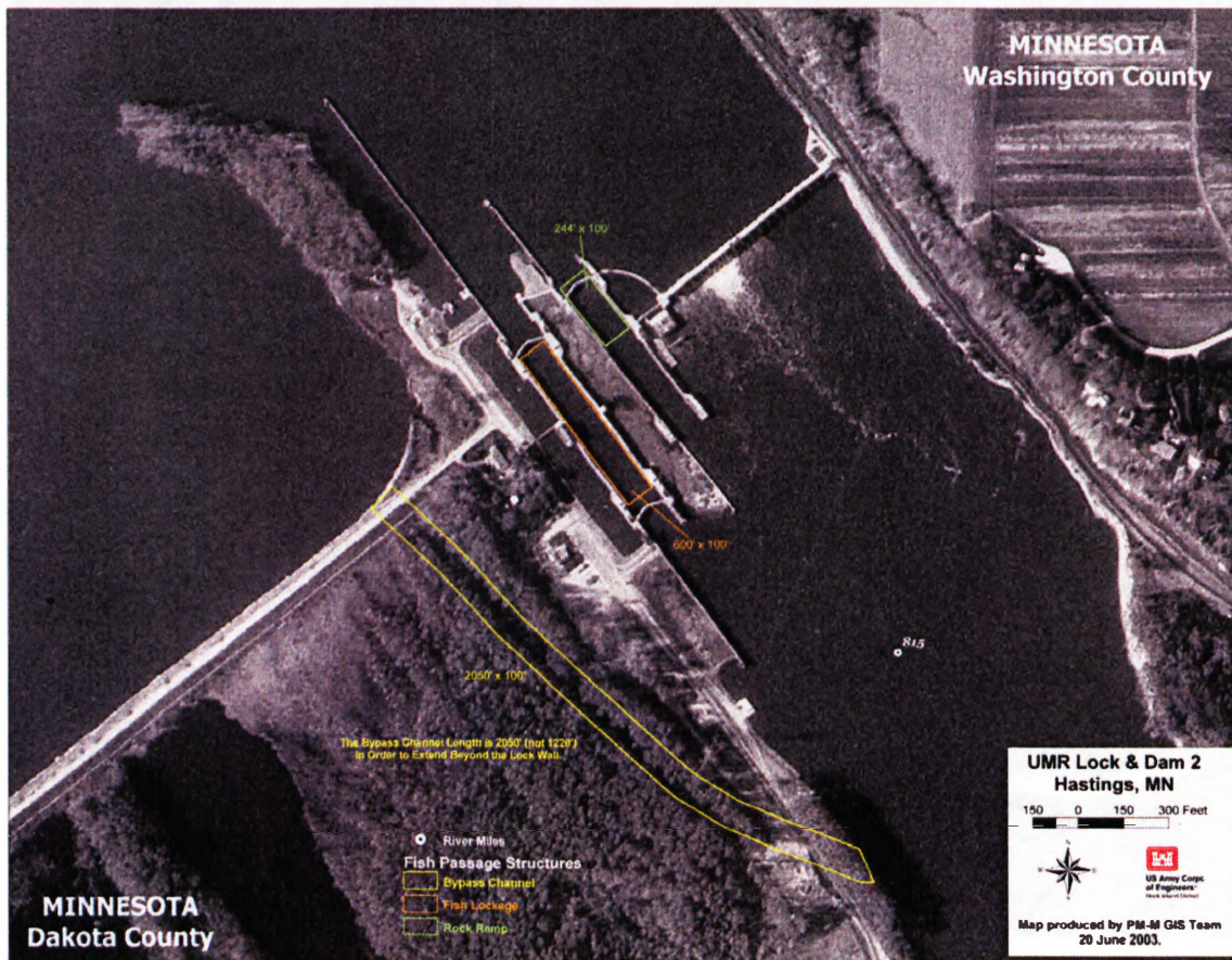
Figure D2. Potential fish passage improvements at Lock and Dam 2, Upper Mississippi River
