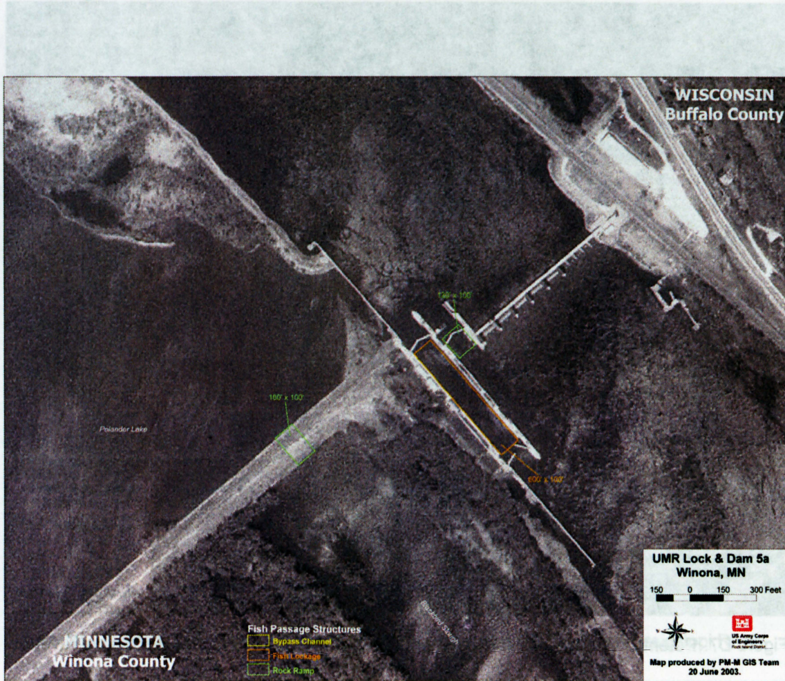
Figure D6. Potential fish passage improvements at Lock and Dam 5A, Upper Mississippi River
