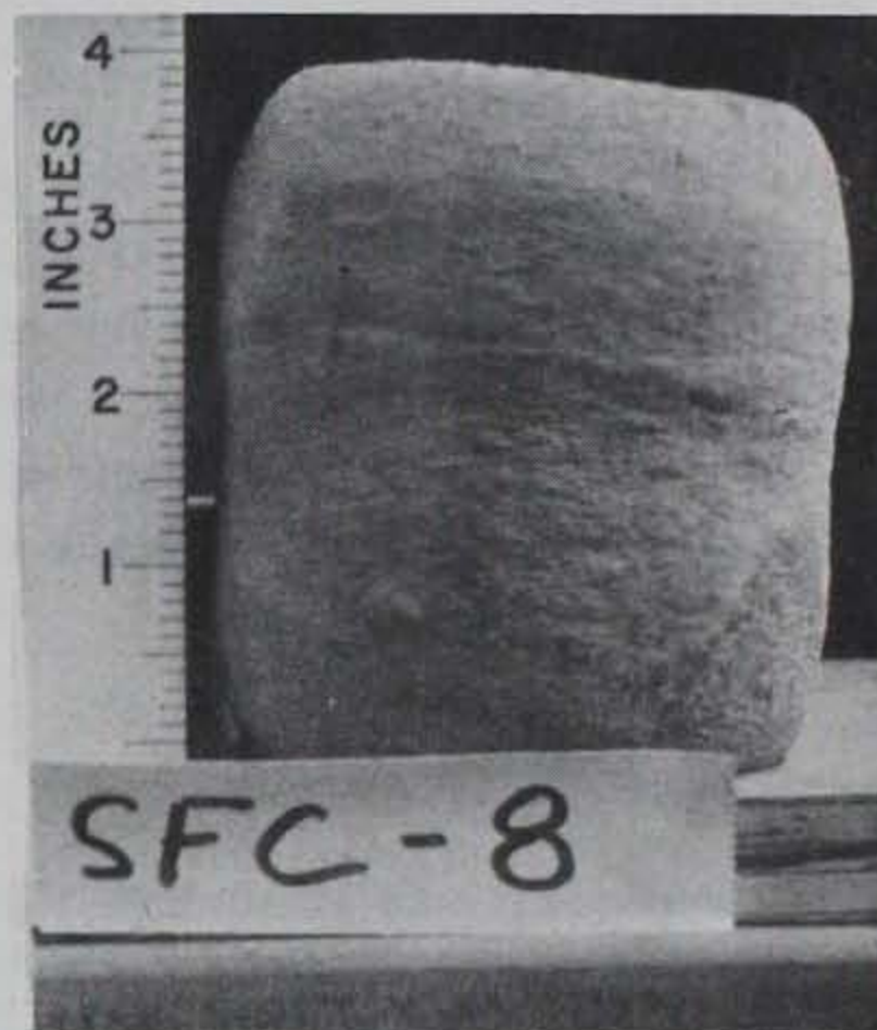
Figure 5. Typical Hanover silt and Suffield clay specimens after unconfined compression testing.
