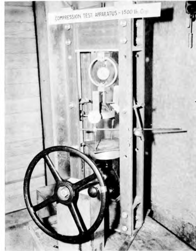
FIG. 2 1500 LB. CAP. SCREW JACK FOR TESTING SAMPLES REQUIRING RAPID TRAVEL OF JACK TO MAINTAIN RATE OF LOAD INCREASE.
