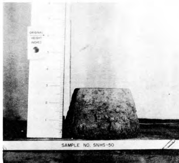
FIG. 2 TEST TEMPERATURE = +31.3^{\circ} F MAX. STRESS = 329 PSI RATE OF LOADING = 400 PSI/MIN.
