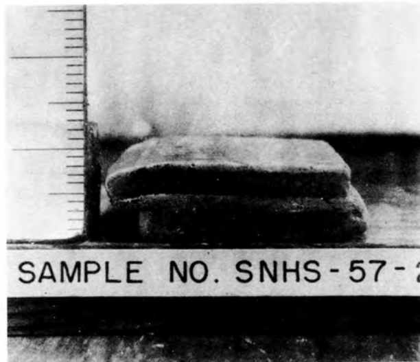
FIG. 2 NEW HAMPSHIRE SILT TEST TEMPERATURE = +31.2^{\circ} F NORMAL LOAD = 40 PSI
