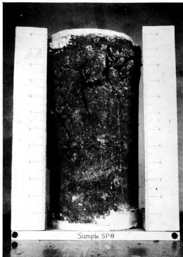
FIG. 1 TEST TEMPERATURE = -6.5^{\circ} F MAX. STRESS = 2135 PSI RATE OF LOADING = 400 PSI/MIN.
