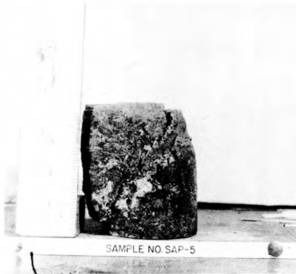
FIG. 1 TEST TEMPERATURE = -10.1^{\circ} F MAX. STRESS = 1699 PSI RATE OF LOADING = 400 PSI/MIN.
