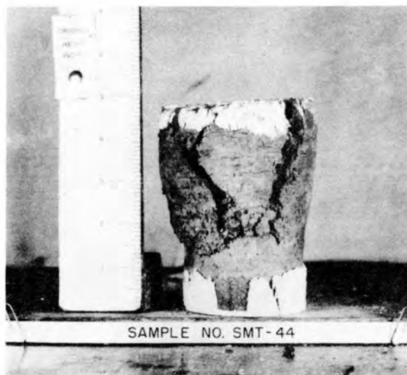
FIG. 2 TEST TEMPERATURE = +31.1^{\circ} F MAX. STRESS = 308 PSI RATE OF LOADING = 1000 PSI/MIN.
