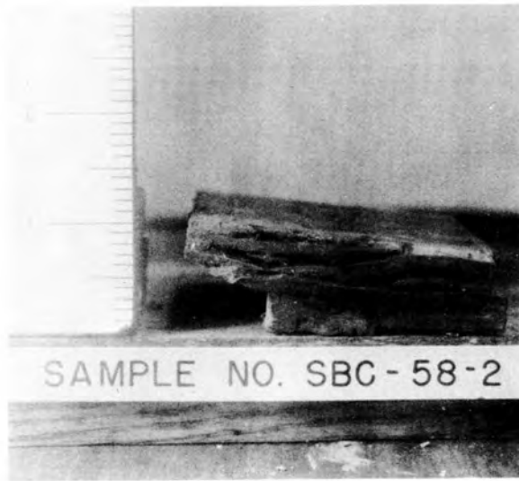
FIG. 1 BOSTON BLUE CLAY TEST TEMPERATURE = +29.6^{\circ} F NORMAL LOAD = 40 PSI
