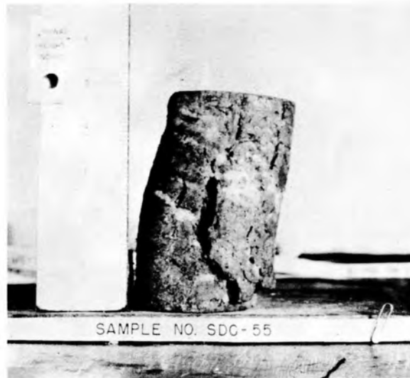
FIG. 1 TEST TEMPERATURE = -4.0^{\circ} F MAX. STRESS = 1415 PSI RATE OF LOADING = 400 PSI/MIN.
