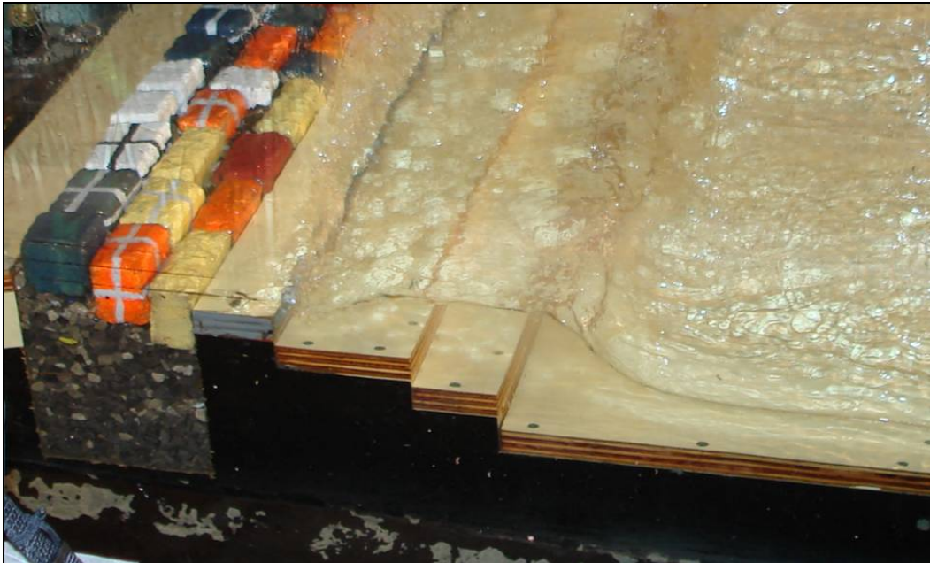
Figure 18. Wave runup on concrete steps (prior to marine mattresses being installed) (photograph courtesy of Drew Benziger, Chicago District).
