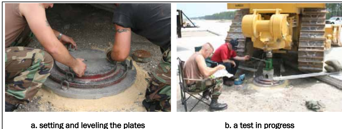
Figure 16. Plate bearing testing on the crater base course material.
