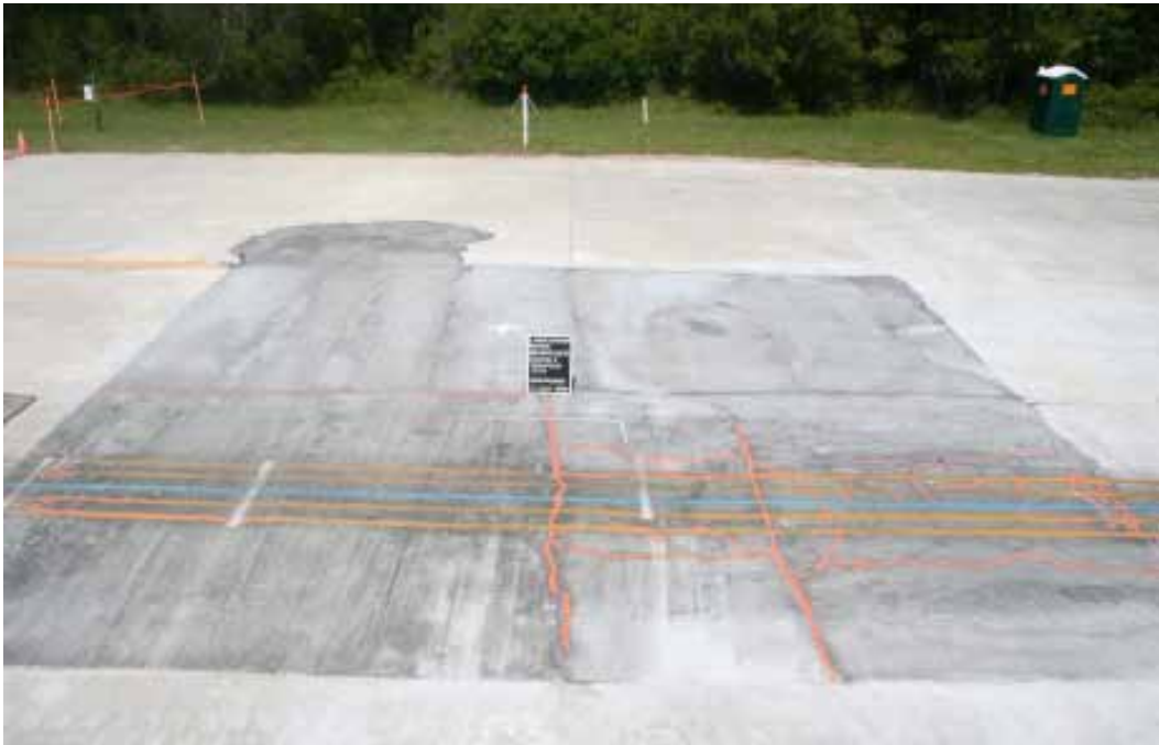
Figure 159. Surface of Crater 2 after 5,008 passes of load cart.
