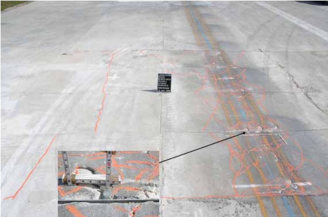
Figure 161. Surface of Crater 4 after 5,008 passes of load cart.
