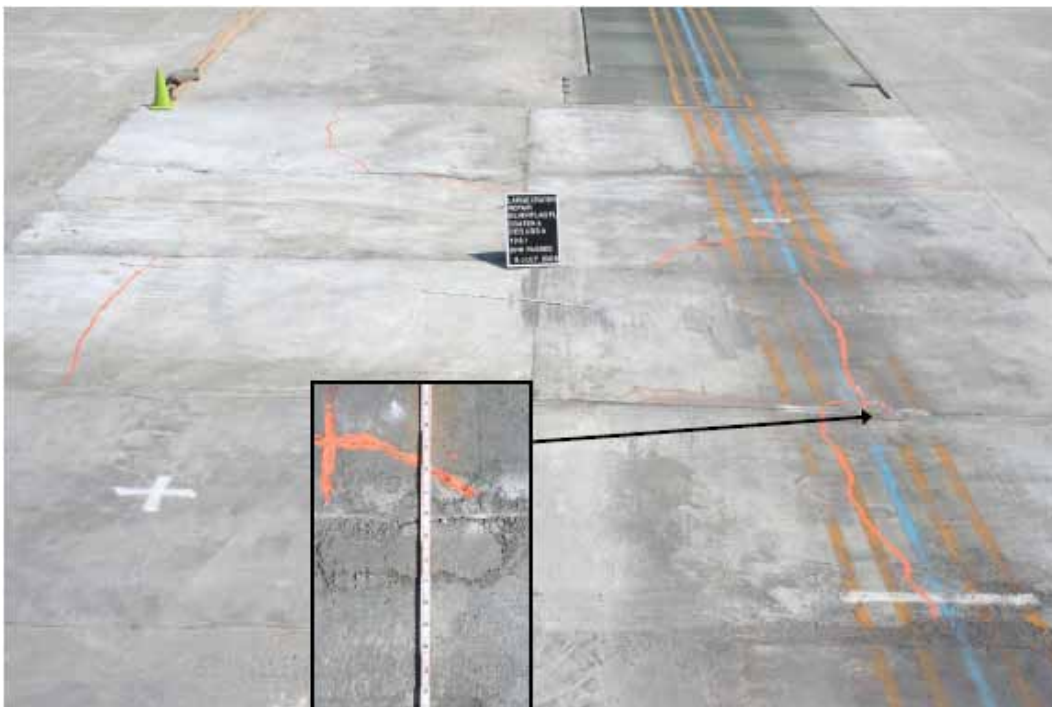
Figure 155. Crater 5 after 2,016 completed load cart passes.
