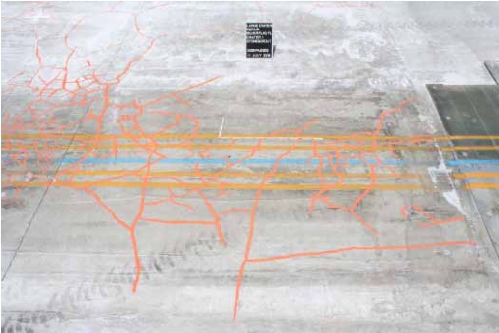
Figure 157. Crater 1 after 5,008 passes of load cart.
