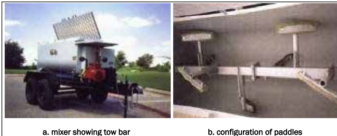
Figure 25. Portable concrete mixer, 2 yd 3 capacity, used for crater repairs.
