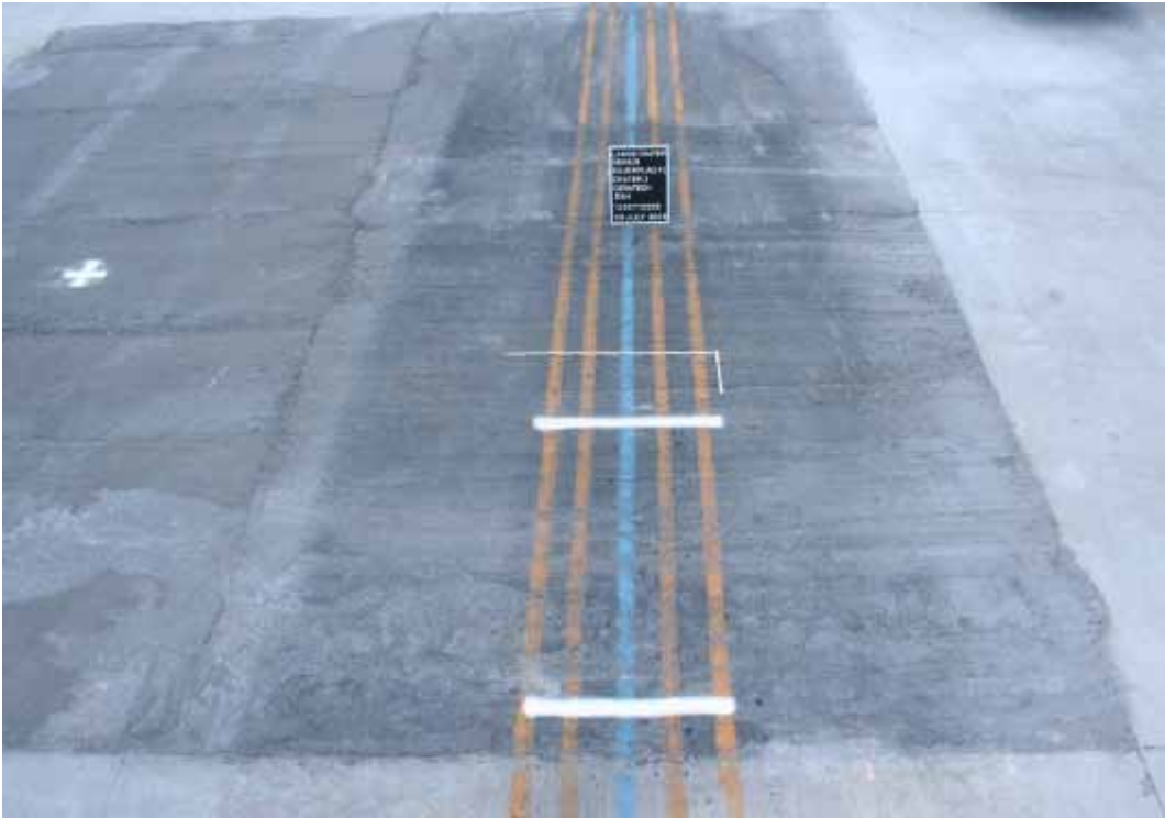
Figure 148. Crater 2 after 1,008 completed load cart passes.
