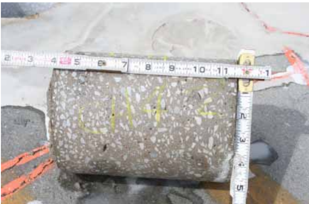
Figure 173. Core 2 from Crater 4 within traffic lane, Ultimax Concrete.
