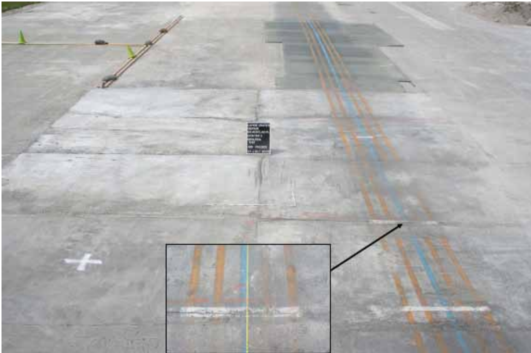
Figure 144. Crater 5 after 528 completed load cart passes.
