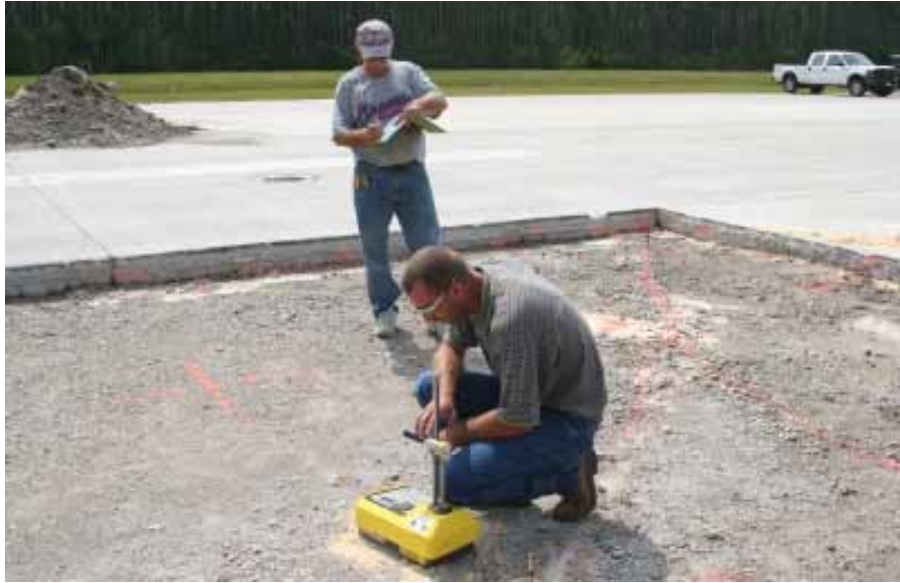
Figure 18. Soil density measurements with the Troxler nuclear gage.
