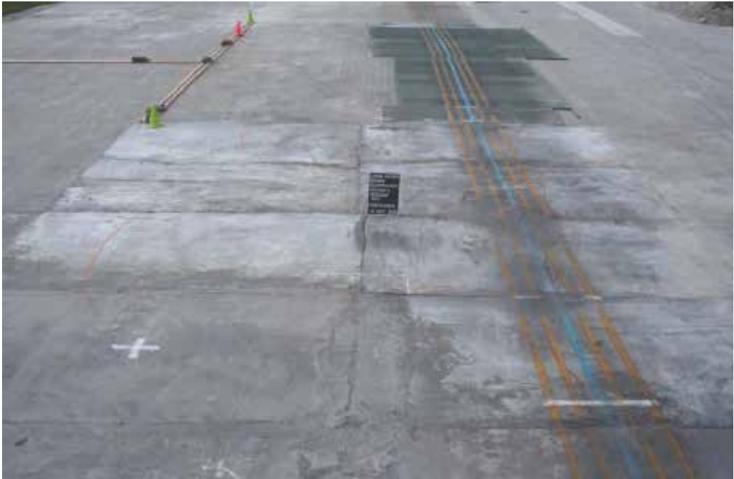
Figure 162. Surface of Crater 5 after 5,008 passes of load cart.
