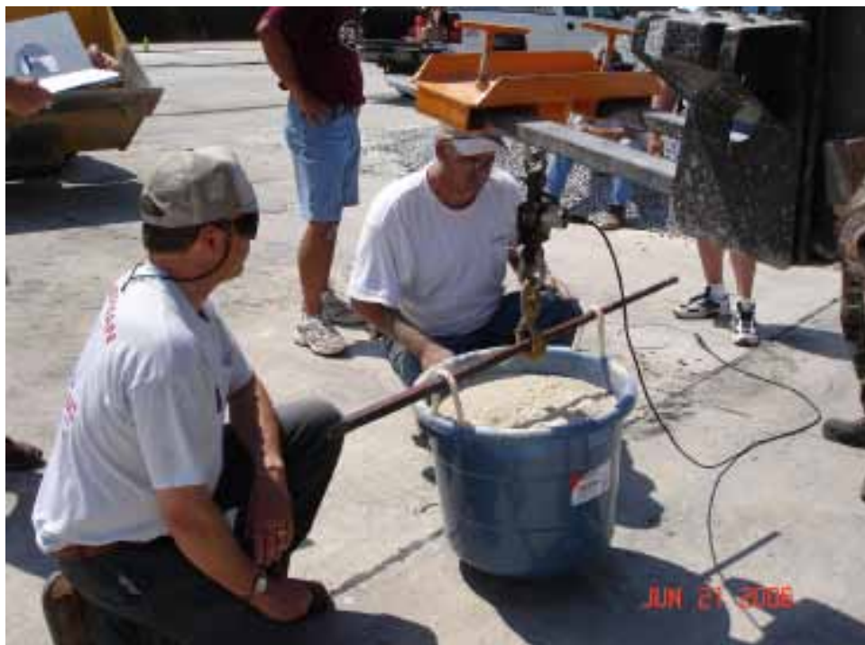
Figure 41. Calibrating the proportional mixer for Crater 6.
