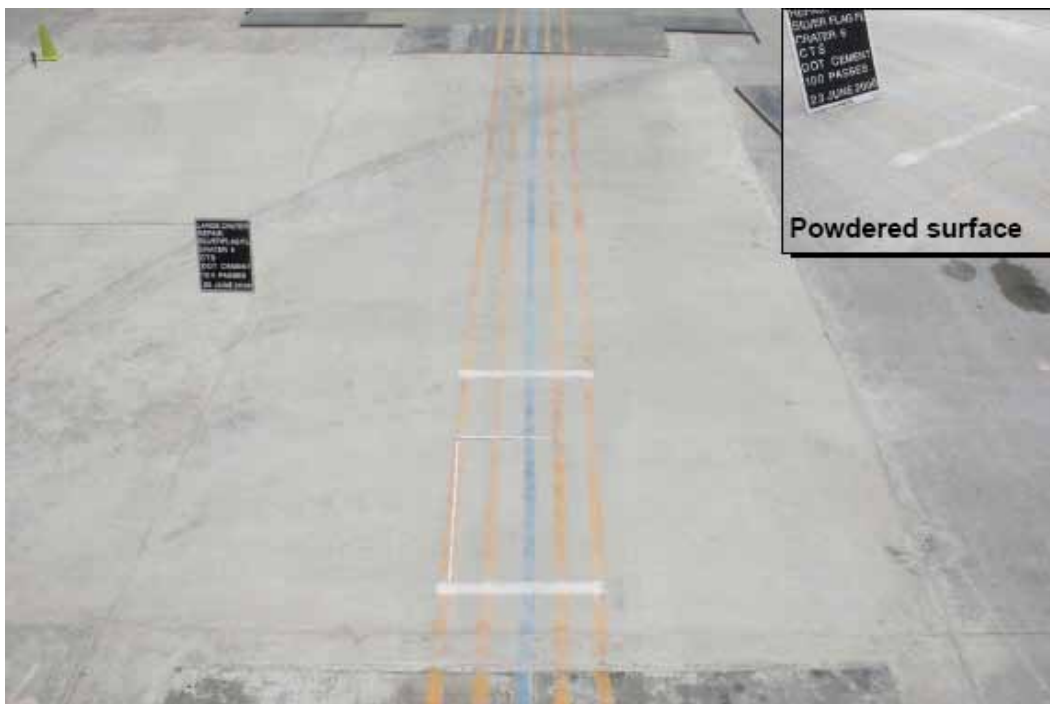
Figure 140. Crater 6 after 100 passes of load cart.
