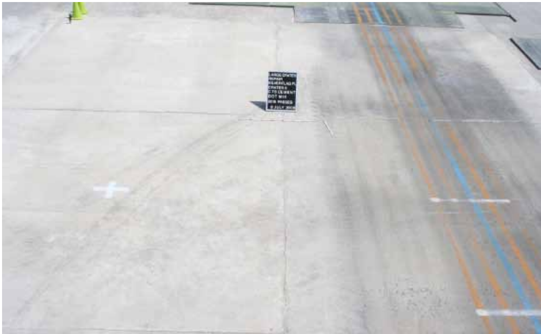
Figure 156. Crater 6 after 2,016 completed load cart passes.
