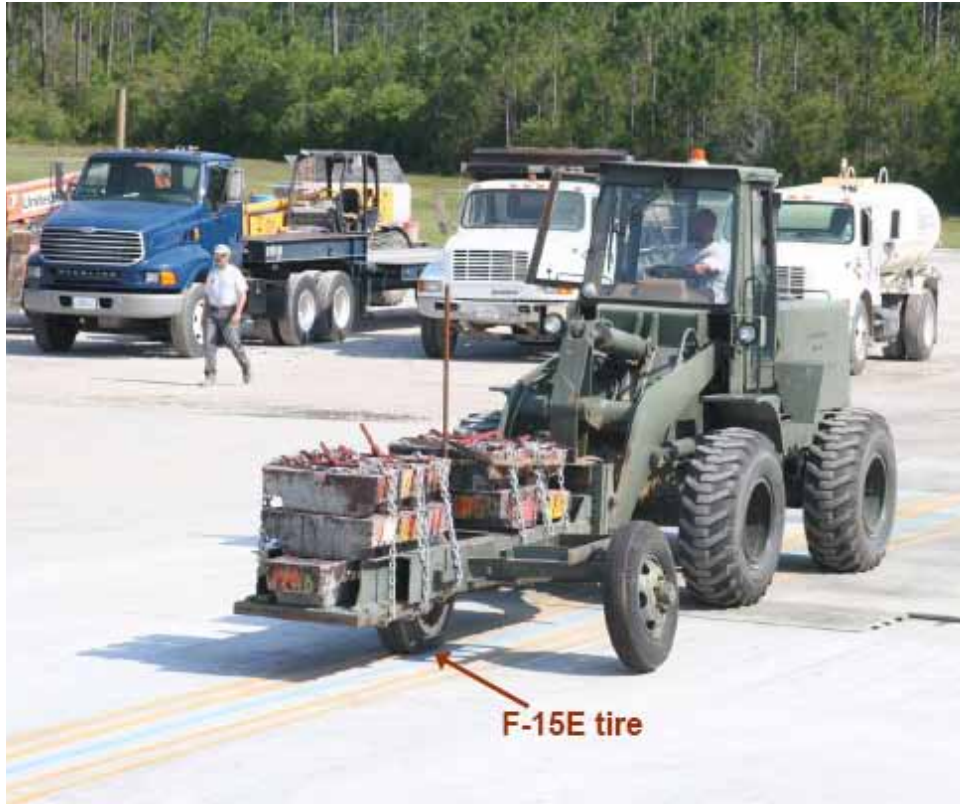
Figure 102. Photograph of F-15E load cart.
