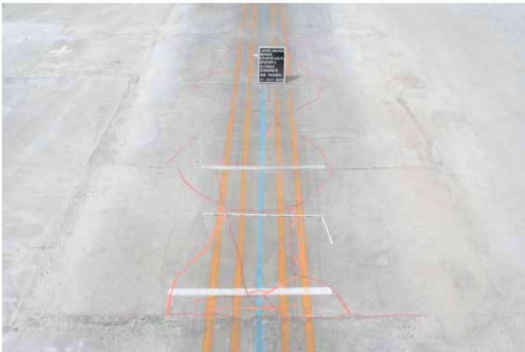
Figure 143. Crater 4 after 528 completed load cart passes.
