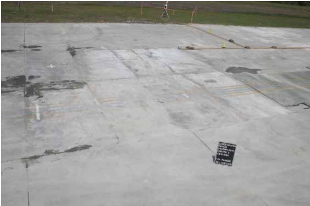
Figure 139. Crater 5 after 100 passes of the load cart.
