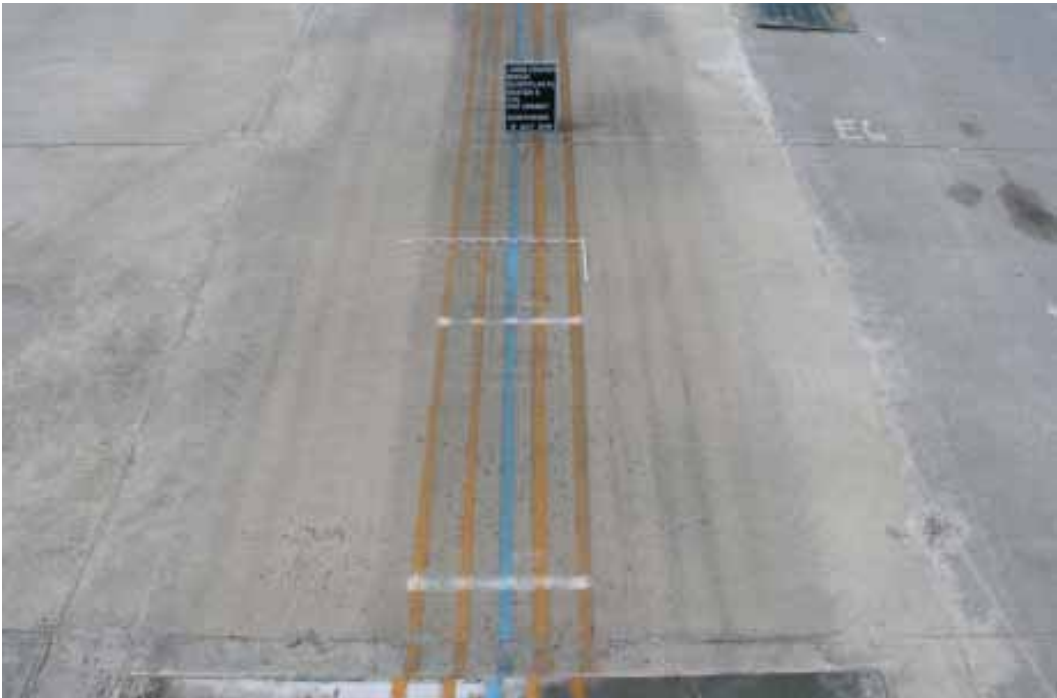
Figure 163. Surface of Crater 6 after 5,008 passes of load cart.
