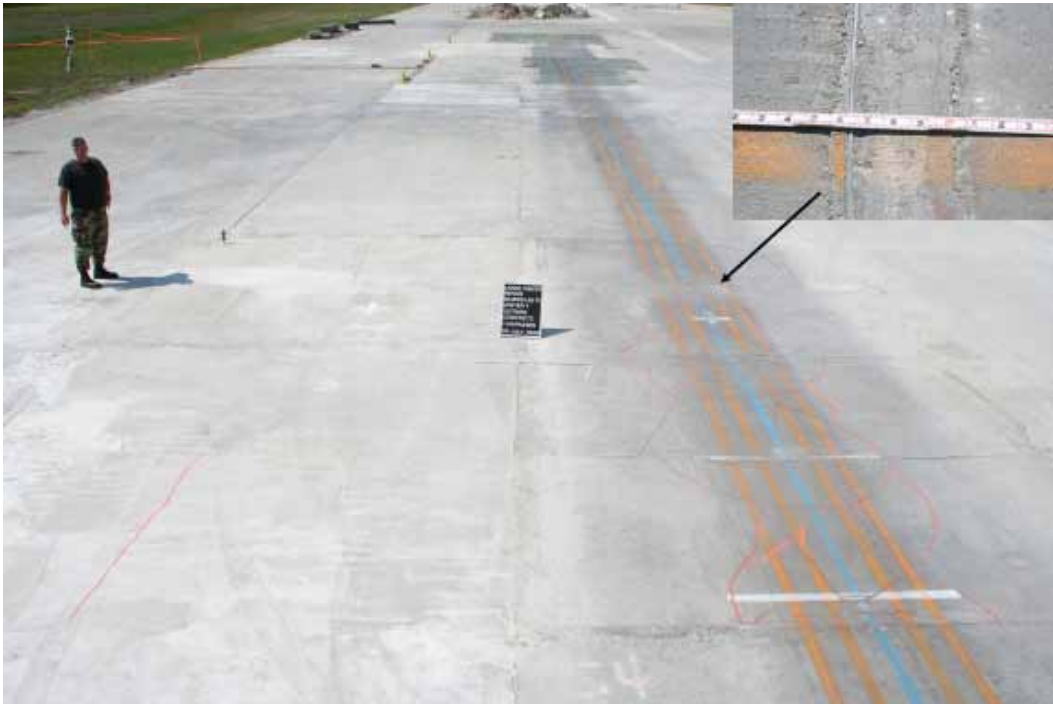
Figure 149. Crater 4 after 1,008 completed load cart passes.
