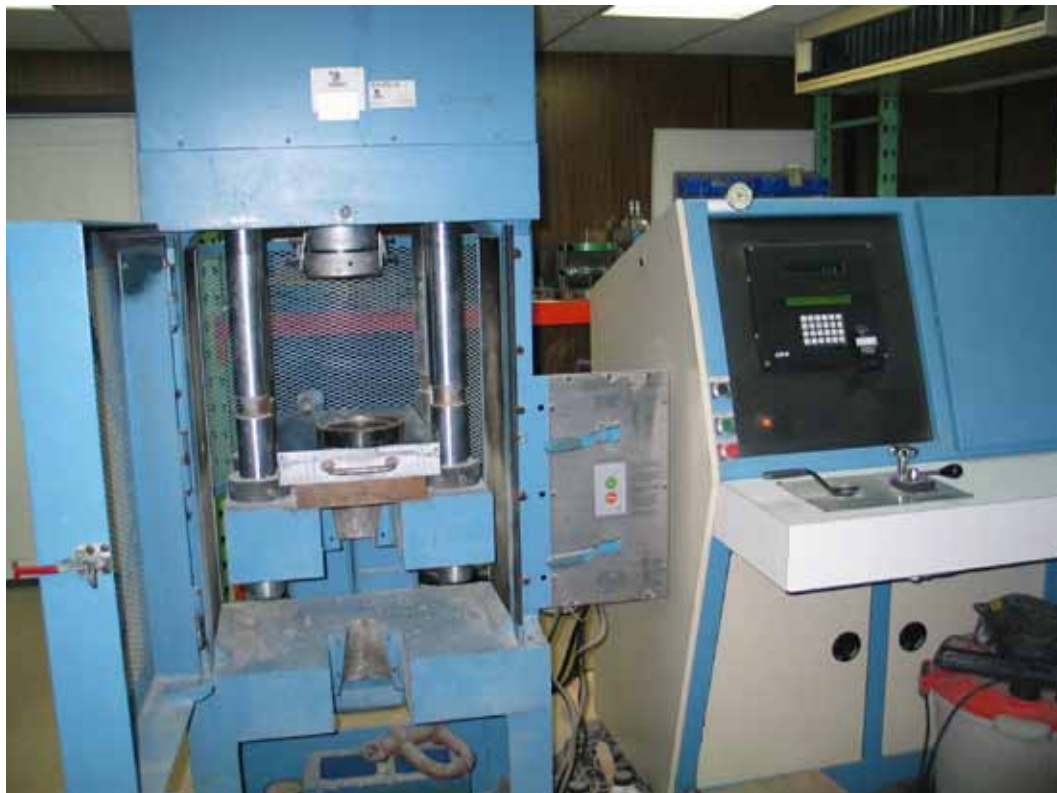
Figure 99. AFRL testing equipment for unconfined compressive strength.
