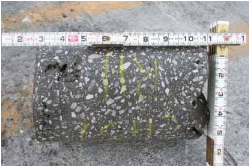
Figure 174. Core 2 from Crater 5, Degussa Thoroc 10-61 material.
