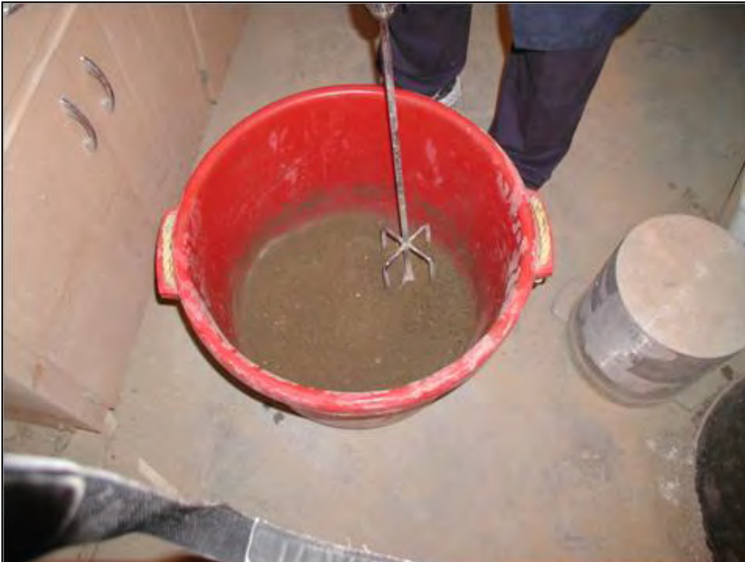
Figure 10. CH soil wetting and mixing.
