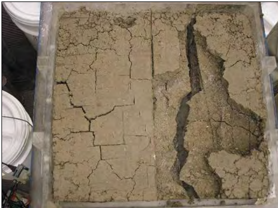
Figure 49. Offset of primary crack formation in subsurface layers.
