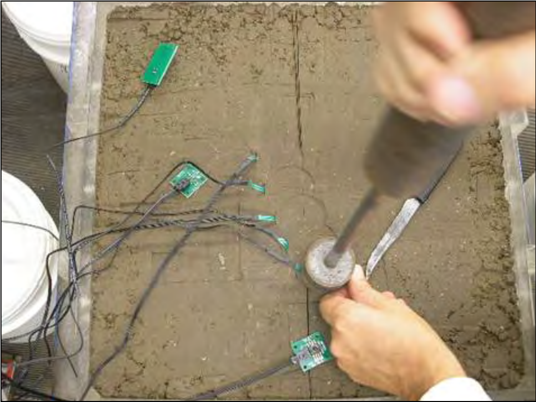
Figure 31. Piston used for compaction around sensor holes.
