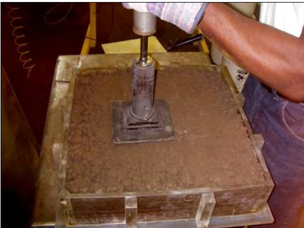
Figure 12. Soil box filled with compacted clay and compaction rammer.
