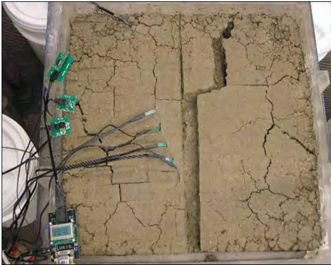
Figure 44. Major crack faulting after 1 month.
