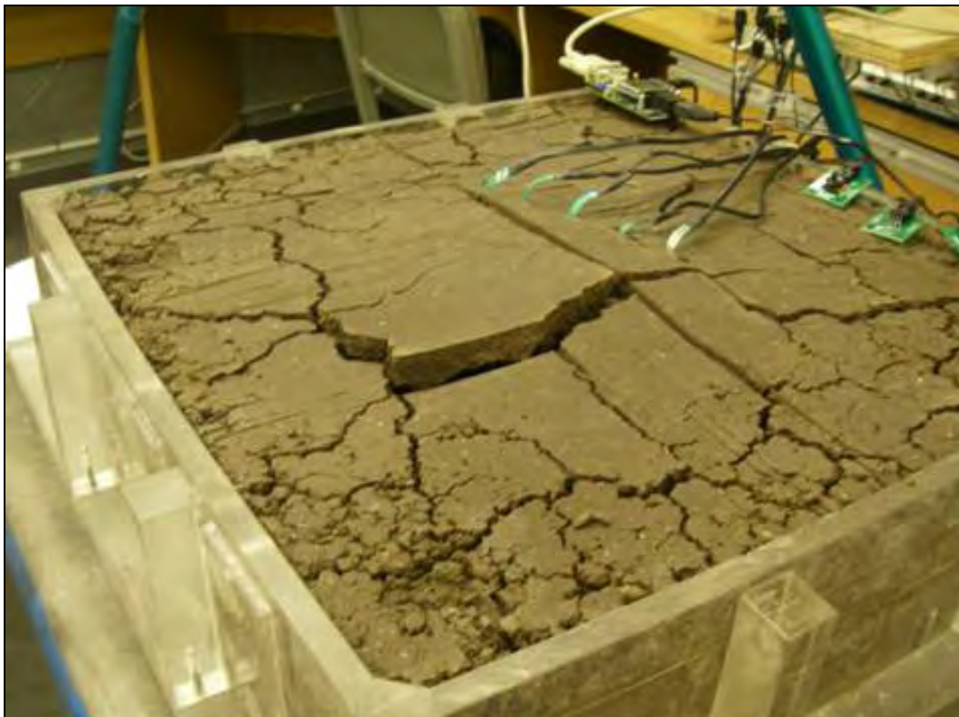
Figure 46. Surface curling in clay mass after 2 days.
