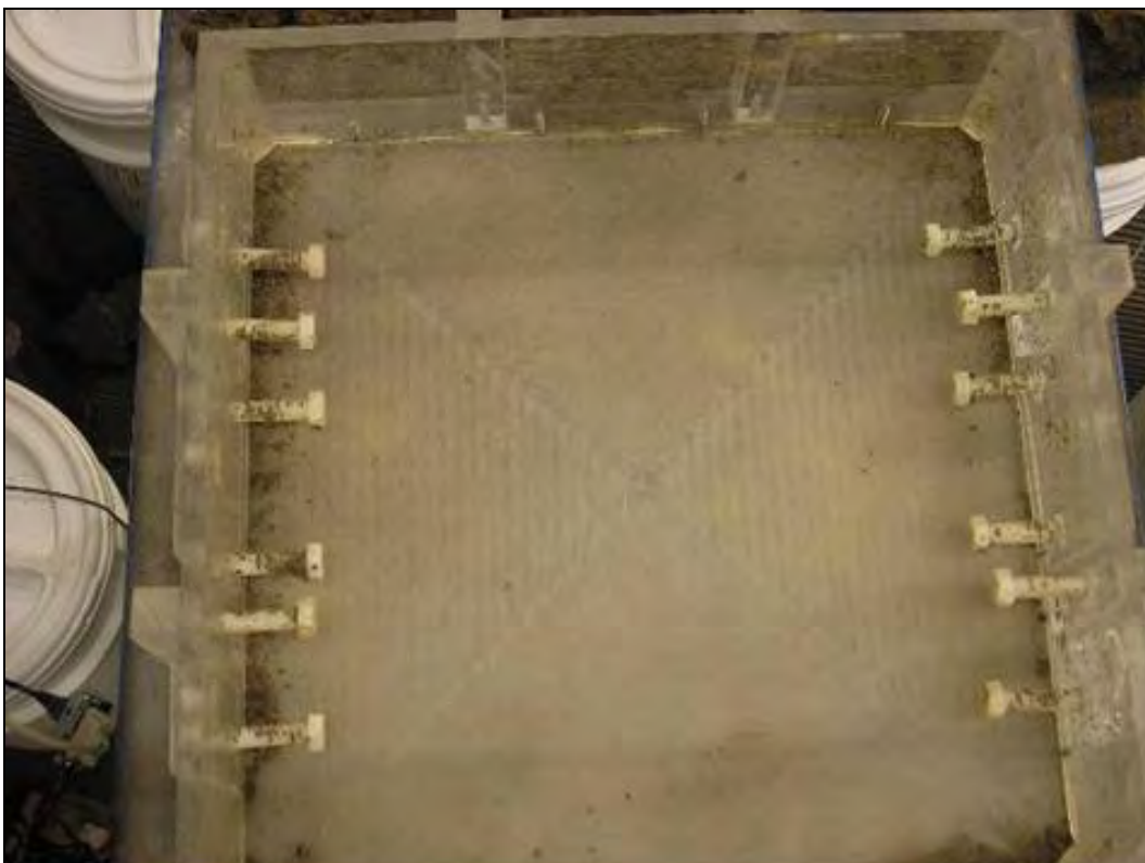
Figure 9. Soil box with soil bolts.
