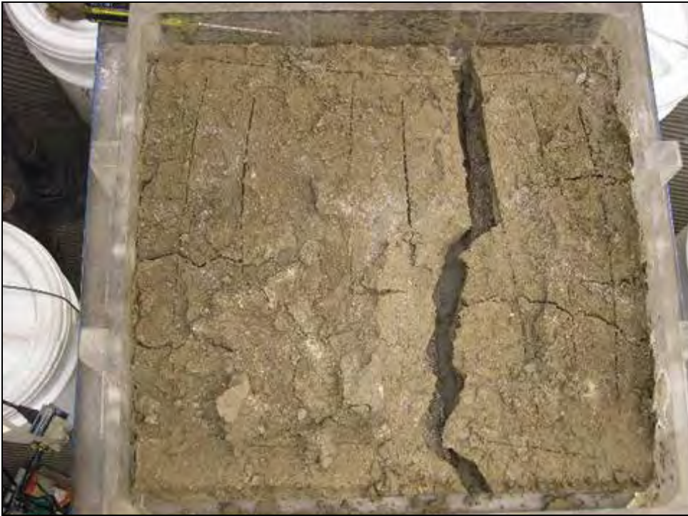
Figure 51. Effect of cracking along scoring lines between compacted lifts.
