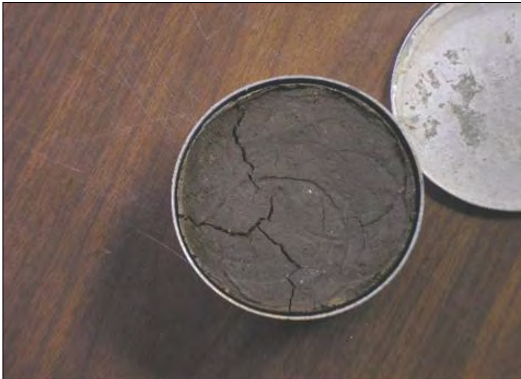
Figure 27. Soil separation from container walls.
