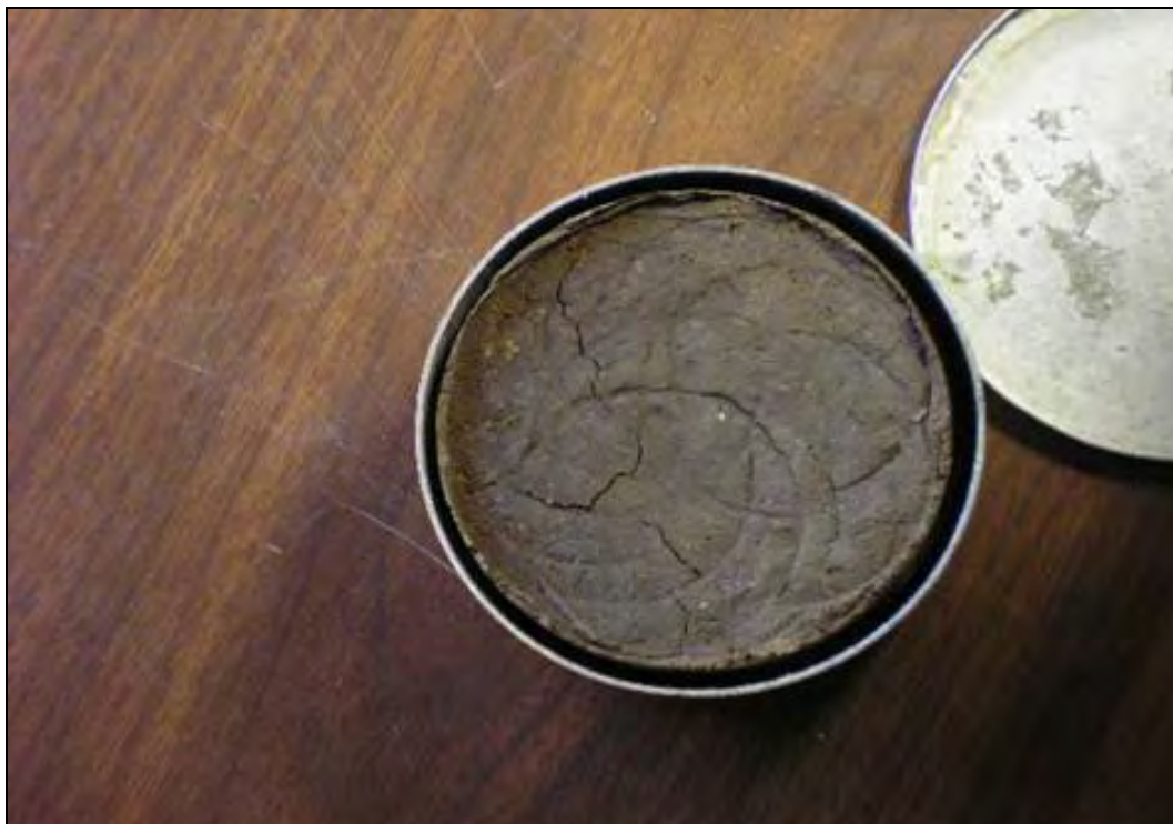
Figure 28. Closing of cracks after 1 month.
