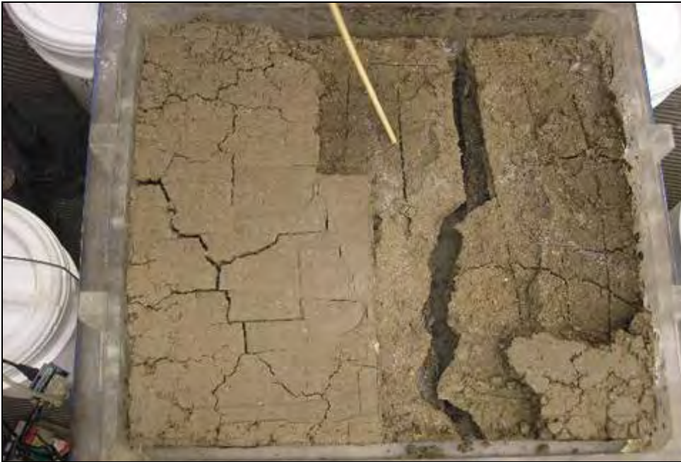
Figure 50. Crack influence due to score mark between compacted lifts.
