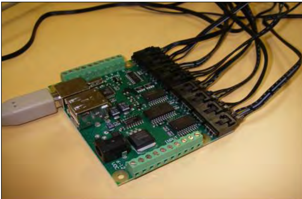
Figure 15. Acquisition board for Phidget™ sensors.
