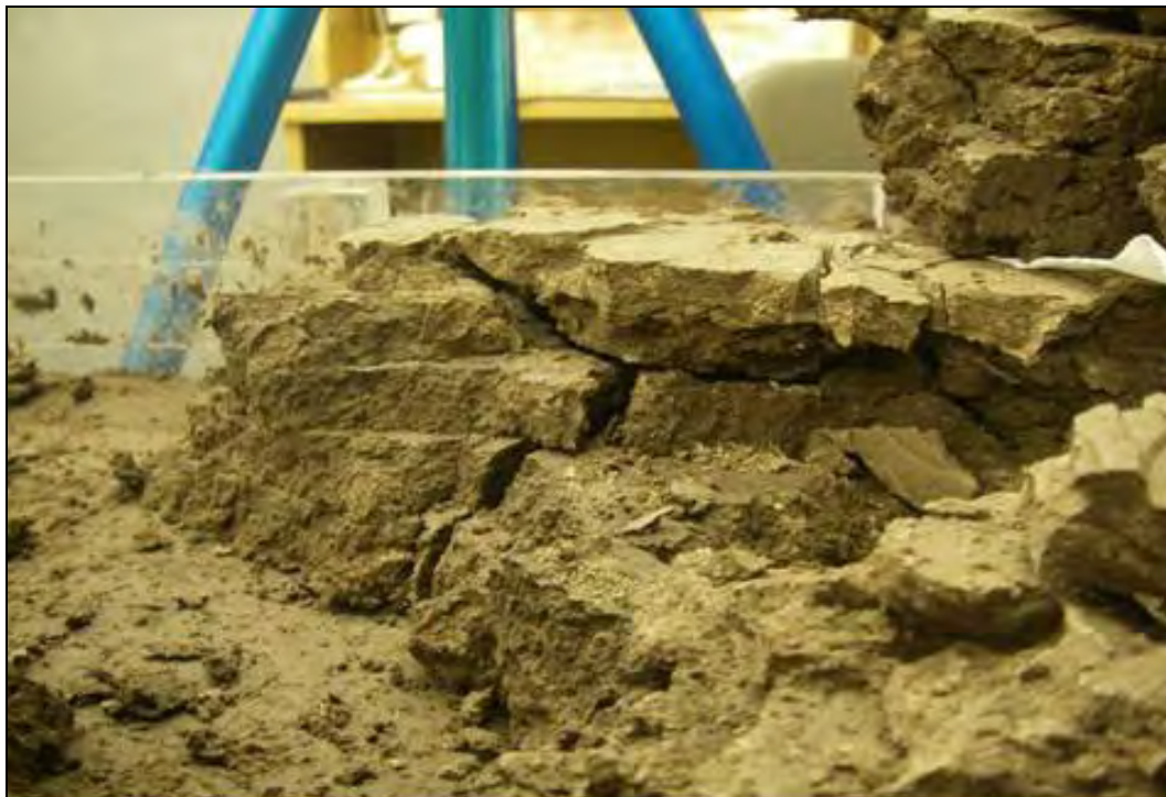
Figure 21. Downward propagation of cracks.
