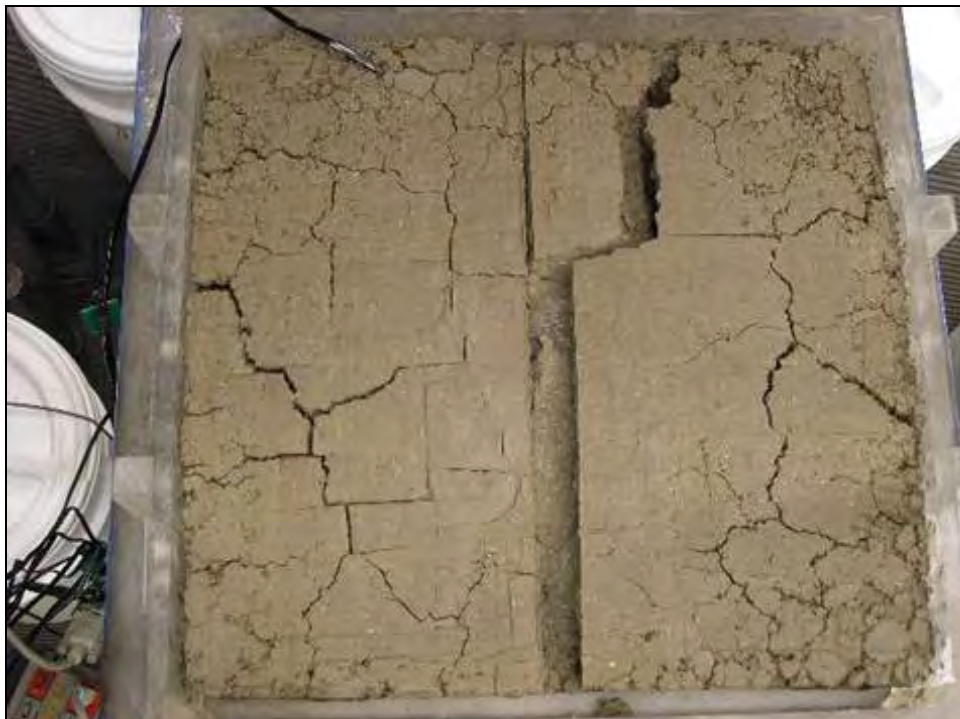
Figure 47. Primary crack formation along score at end of test.
