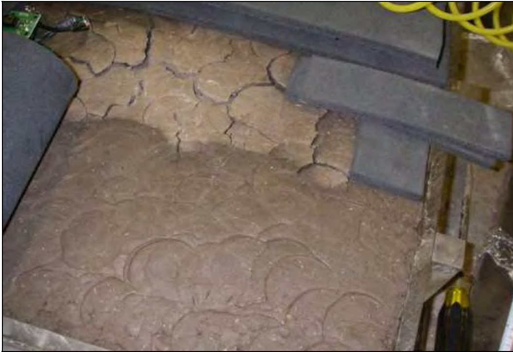
Figure 13. Contrast between dried clay under drying box and protected clay under plastic sheet at end of experiment
