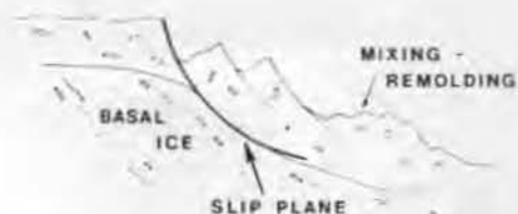
Figure 51. Schematic diagram of slump of sediment on buried basal ice of low-angle slope. Slump occurs due to rotational slip along ice/sediment interface; sediments may undergo re-molding followed by flow after slope failure.
