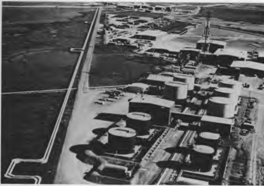
Figure 24. Part of the Prudhoe Bay oil field showing pipelines, roads and gravel pads. (Photo by D.A. Walker, 14 July 1981.)
