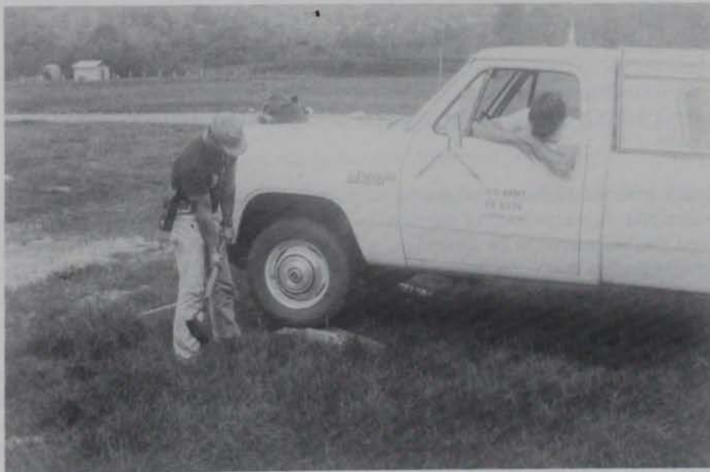
Figure 15. Source used for the S-wave refraction experiments. By recording hammer blows on each end of the beam separately, the reversed polarity of the SH waves that are generated can be used as an aid in their identification on the seismograms.
