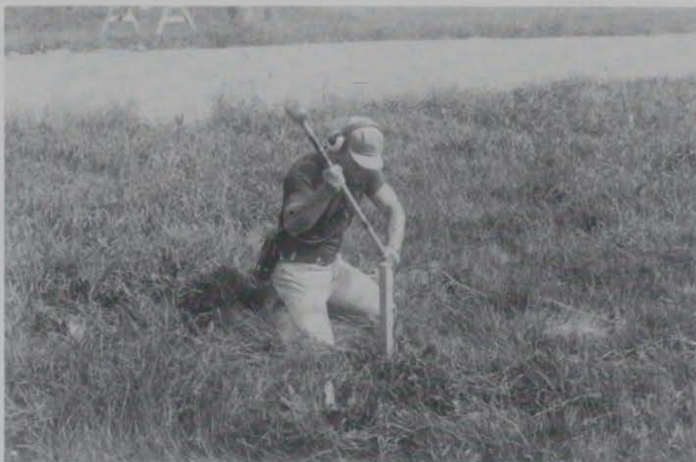
Figure 13. Source used for the P -wave refraction experiments was a vertical sledge hammer blow upon a metal plate placed on the ground. A motion-sensitive switch is taped to the hammer, and starts the recording system via the cable.
