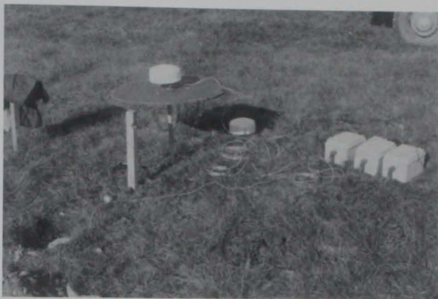
Figure 6. Emplacement of microphones (without the windscreens) and geophones. The boxes contain a battery power supply and attenuation resistance bridge for the microphones.
