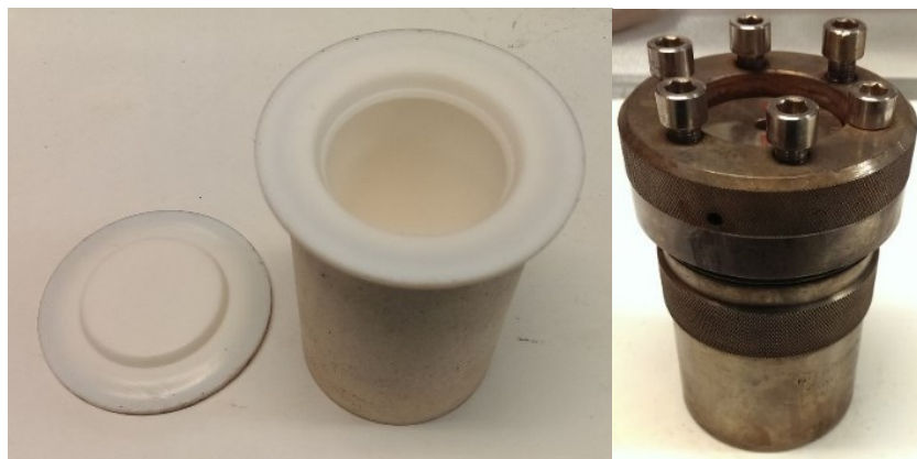
Figure 3.4 – Teflon container (left) and the closed pressure bomb (right).
