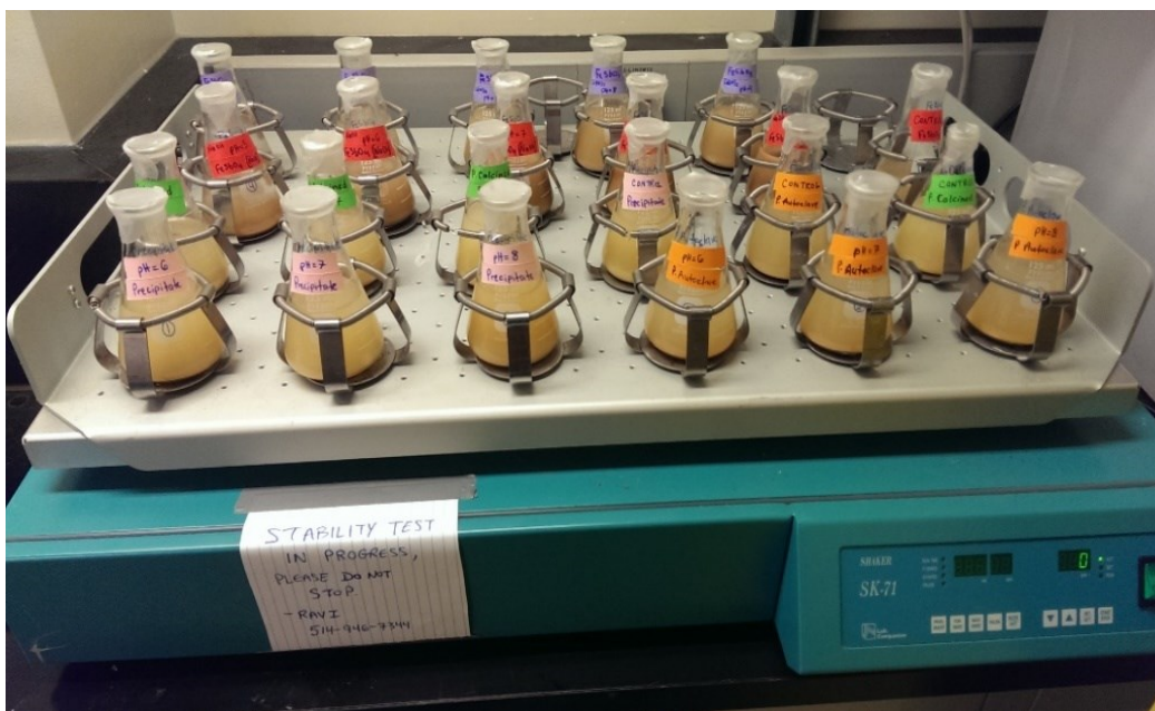
Figure 3.6 – Stability test – precipitate samples in pH controlled solutions agitated on a shaker table.
