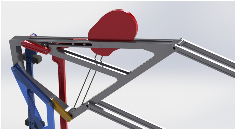
Figure 8.5: Slider-crank mechanism that is actuated by a cam.
