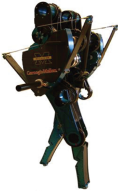
(d) Robot legs with spring loaded drivetrain [39]
