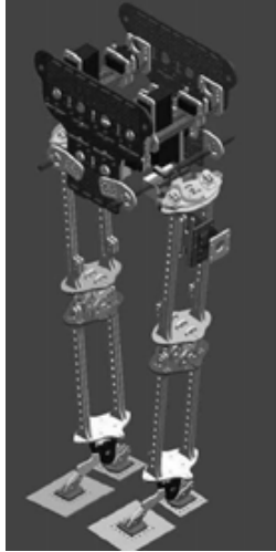
(a) Biped robot with compliant knees [37]
