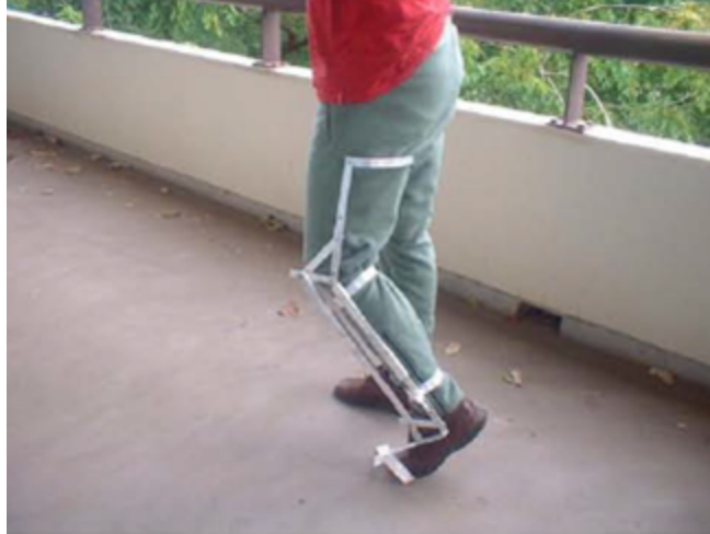
Figure 1.10: Orthotic with passive linkage [4]
