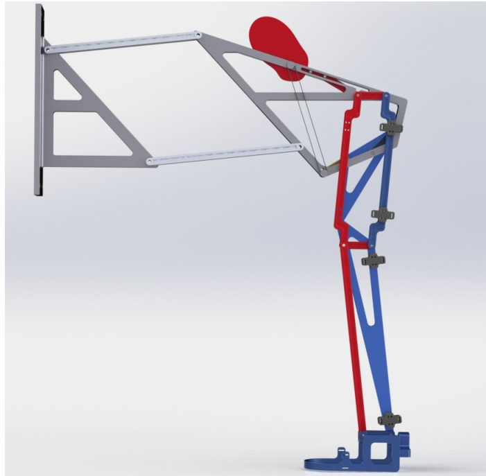
Figure 8.6: The parallelogram mechanism attaches to the six-bar linkage in order to control the foot orientation angle.
