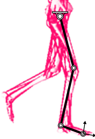
Figure 2.2: 3R chain matching the dimensions of the human leg
