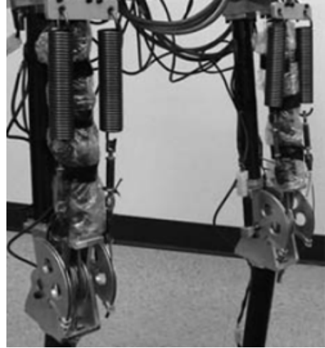
(b) Biped robot with spring loaded knees [38]
