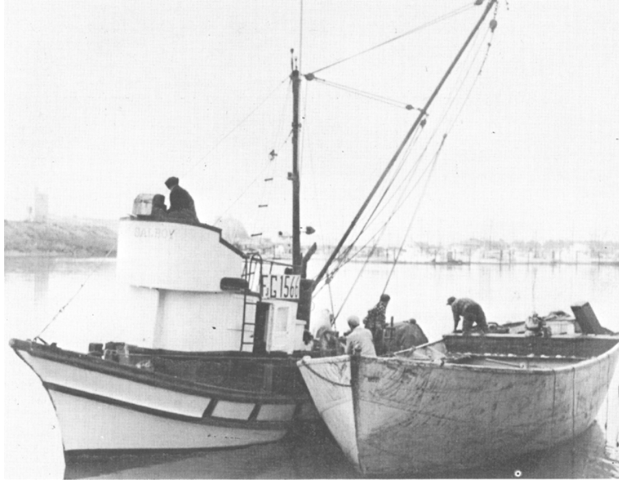
FIGURE 5. Monterey Bay lampara vessel with a 25-ton capacity lighter.
