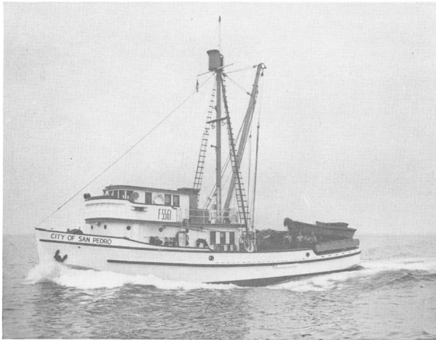
FIGURE 15. A modern purse seiner. Note two skiffs riding the net. Photograph by Kent Hitchcock, 1947.
