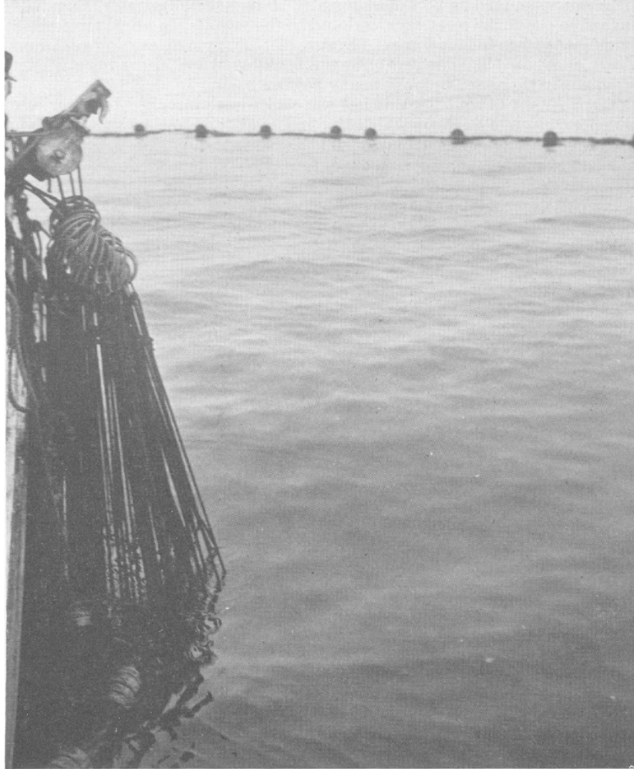
FIGURE 32. Seine has been pursed and purse rings are bunched at the davit ready to be hoisted aboard. Corkline with rubber ball floats in background. Photograph by J. B. Phillips. September, 1945.
