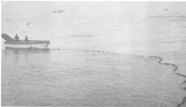
FIGURE 19. Circle completed and skiff has moved out to purse portions of the corkline. Photograph by J. E. Fitch. August, 1948.
