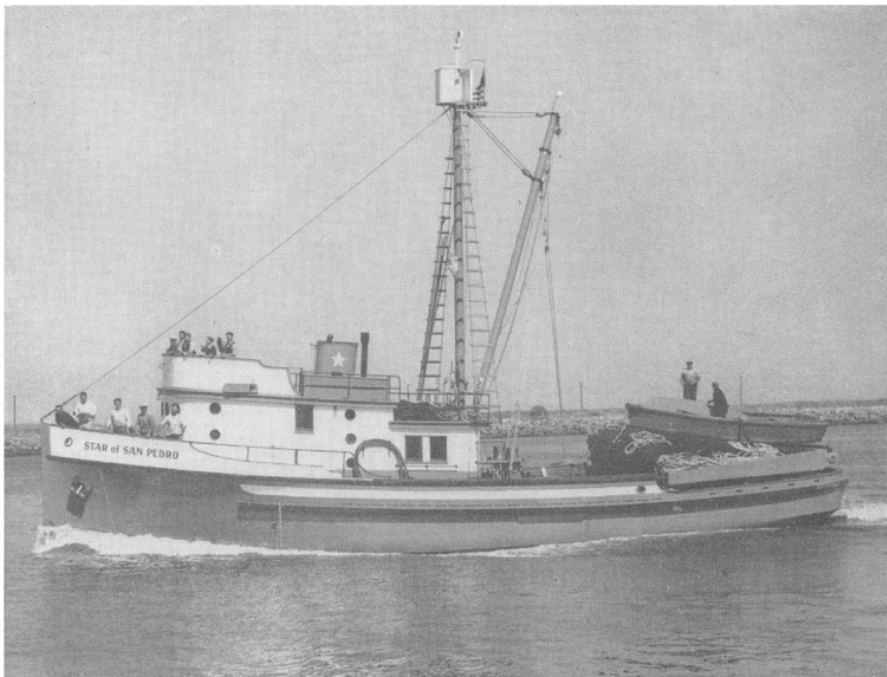
FIGURE 2. A California purse seine boat. Skiff riding the stacked net on after deck turntable. Photograph by Vernon M. Hadden.
