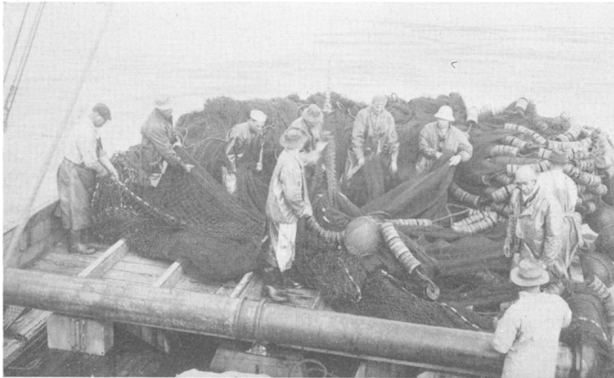
FIGURE 33. Crew on turntable stacking the bag end of a purse seine after washing it at sea. Rubber ball float shown on the corkline. Photograph by J. B. Phillips. September, 1945.
