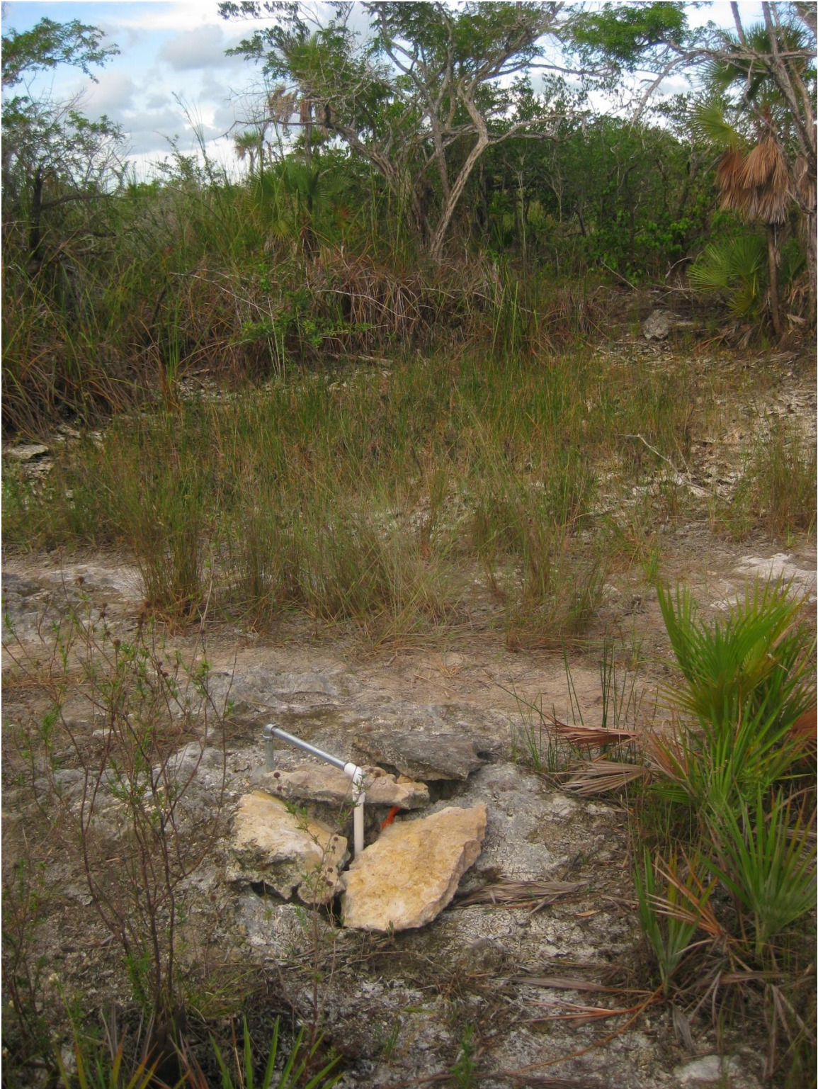
Figure 3.9 North pressure transducer installed in a small opening in the bedrock.
