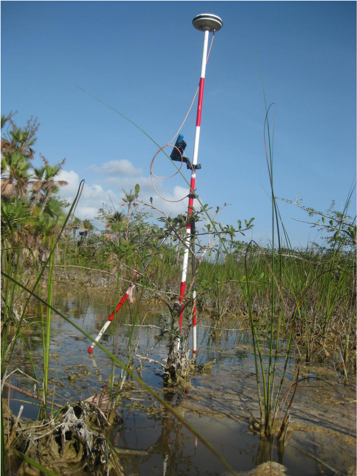
Figure 3.7 The set-up of the high-resolution GPS receiver on the datum of Group Two.
