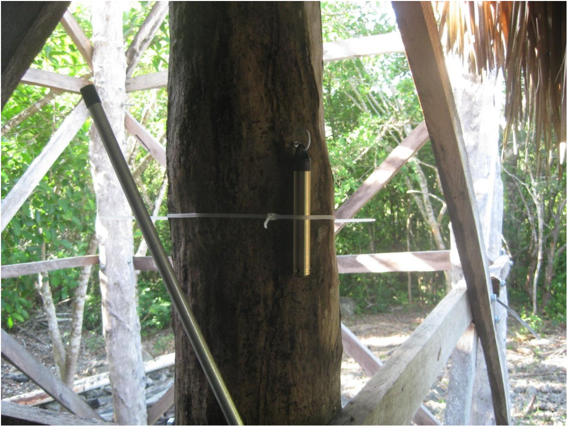
Figure 3.11 The barologger attached to a support beam at the main El Edén house.
