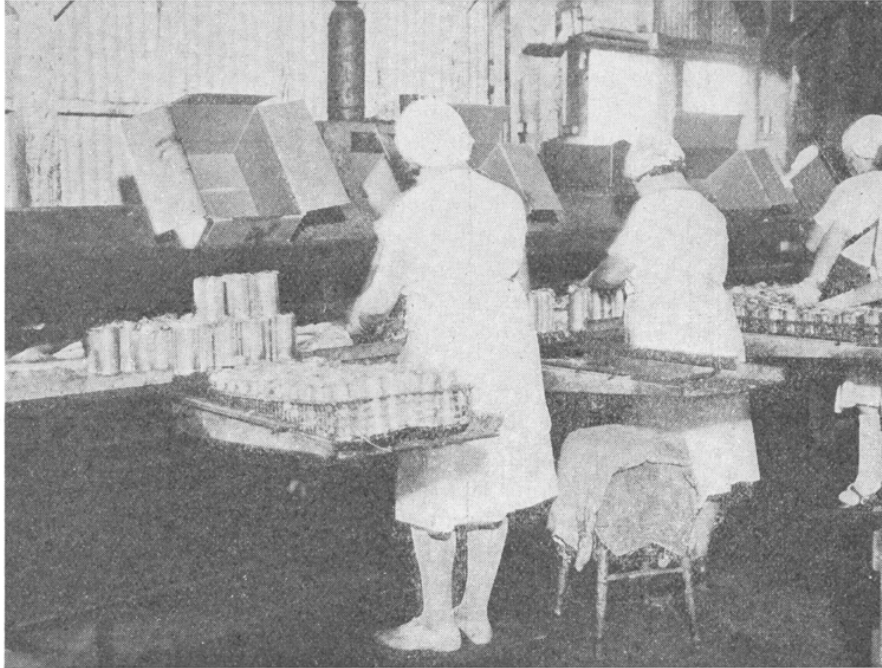
FIG. 64. Packing mackerel in one-pound tall cans at a San Pedro cannery. The empty cans are kept in the cardboard boxes above the packing table. The trays of filled cans are carried by hand to the exhaust box. Note difference between this line and one shown in figure 65. Photograph by D. H. Fry, Jr., and author, August, 1931.
