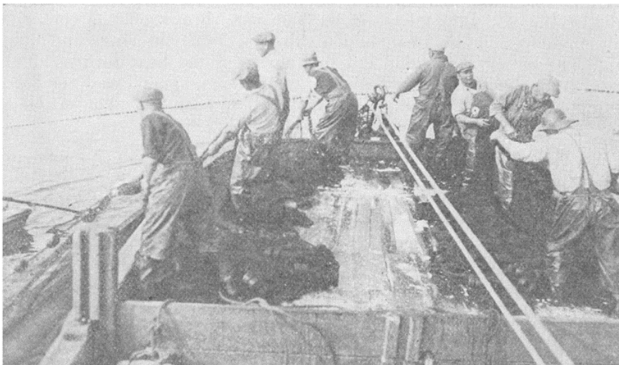
FIG. 41. Hauling in the bag of a mackerel ring net. The wings are already aboard. Note the bunched rings on the pursing block at the stern, the purse lines running forward to the winch, and the buoy keg which can be seen in the lower left corner. The skiff is still inside the circle but is leaving at the left. Photograph by author, December, 1931.
