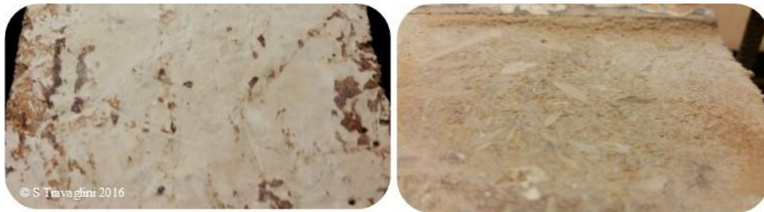
Figure 30. Sanding test specimen surface with 120 grit, showing Grade 2 - Good surface finish before (left), and Grade 3 - Fair surface finish after (right).
