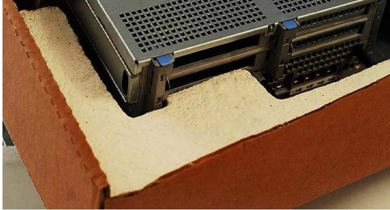
Figure 45. Ecovative Design LLC's fungi-based materials designed for Dell electronic component packaging (Ecovative Design LLC, 2019b)
