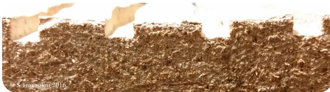
Figure 27. Milling test specimen showing profile of milled grooves.
