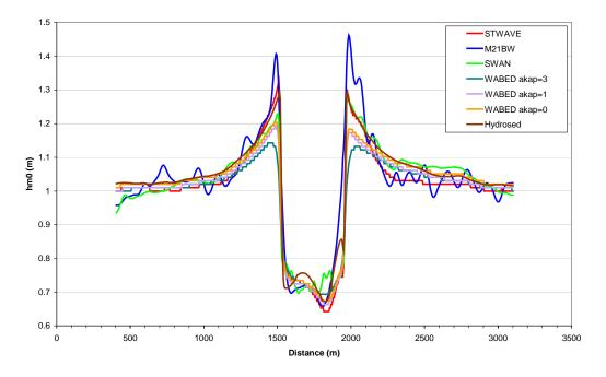
Figure 3.70 Wave Height Comparison for the 700 m Alongshore Line (12 s)
