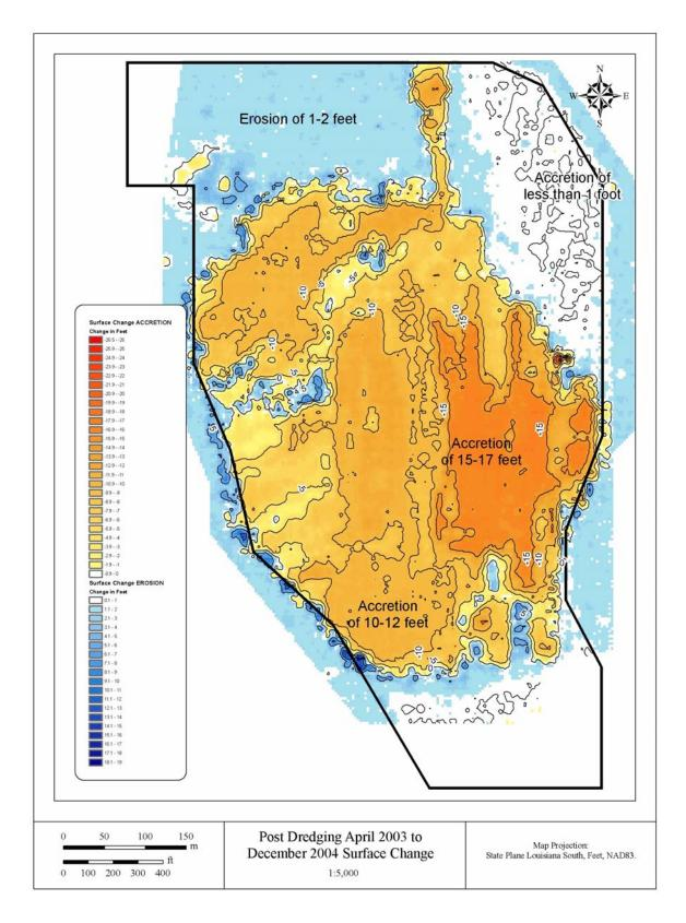
Figure 3.5 Seafloor Surface Elevation Change April 2003 to December 2004
