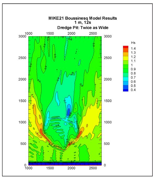
Figure 3.98 Distribution of Significant Wave Height from M21BW Results for the Twice as Wide Dredge Pit (wave conditions same as Figure 3.92 and coordinates are in meters)
