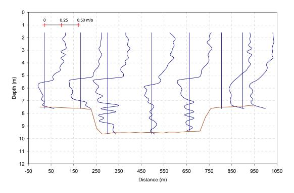
Figure B.2.13 Velocity Profiles for East-West Transect Line (File no. 190058)
