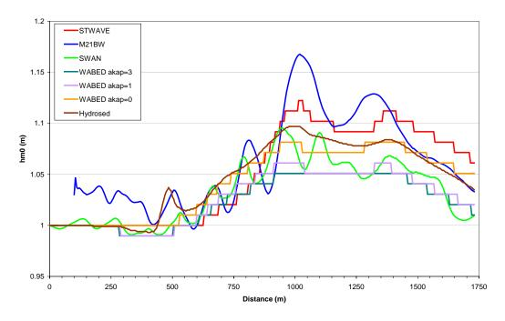
Figure 3.80 Wave Height Comparison for the 1000 m Cross Shore Line (12 s)
