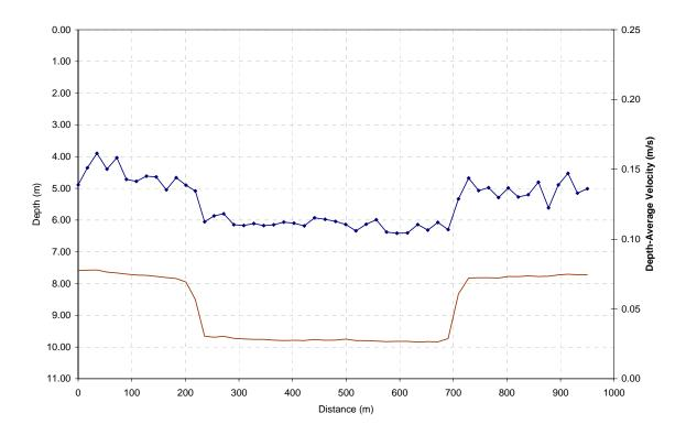
Figure B.2.29 Depth-Average Flow Velocity Change Across East-West Cross-Section (File no. 141039)
