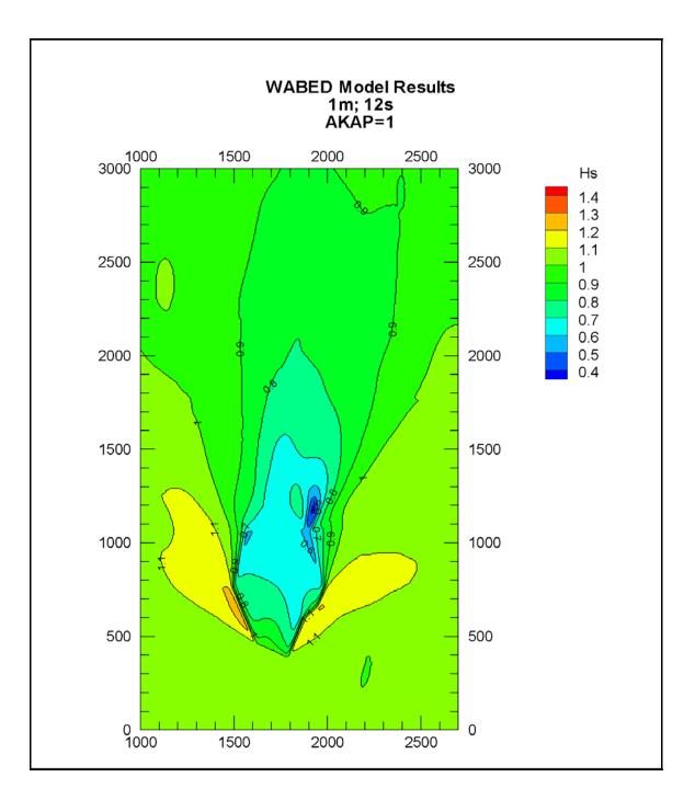
Figure 3.62 Colour Contour Plots of Significant Wave Height for  $T_p = 12s$  by WABED with Diffraction Coefficient of akap = 1(coordinates are in meters)
