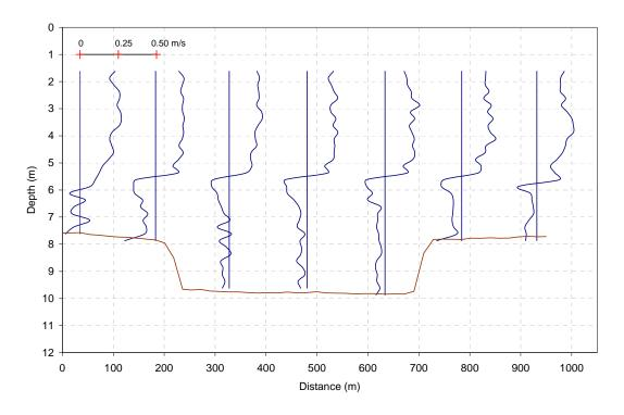
Figure B.2.9 Velocity Profiles for East-West Transect Line (File no. 141039)
