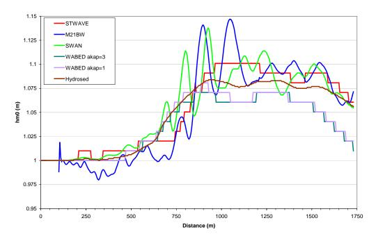
Figure 3.91 Wave Height Comparison for the 2500 m Cross Shore Line (9 s)
