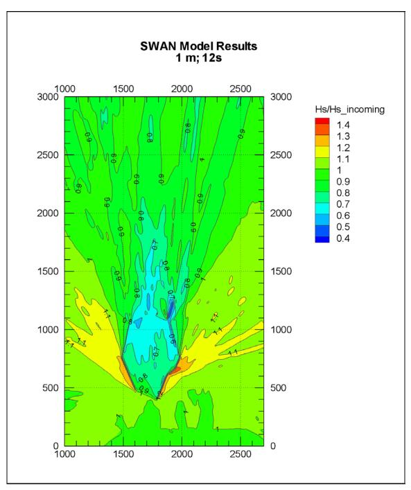
Figure 3.59 Colour Contour Plots of Significant Wave Height for Tp=12s by SWAN (coordinates are in meters)
