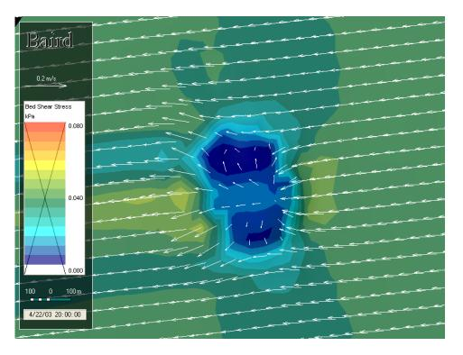
Figure 3.47b First Close-up of the Near Bed Flow Vectors Overlaid on the Bed Shears Stress Map for the Lower Flow Condition
