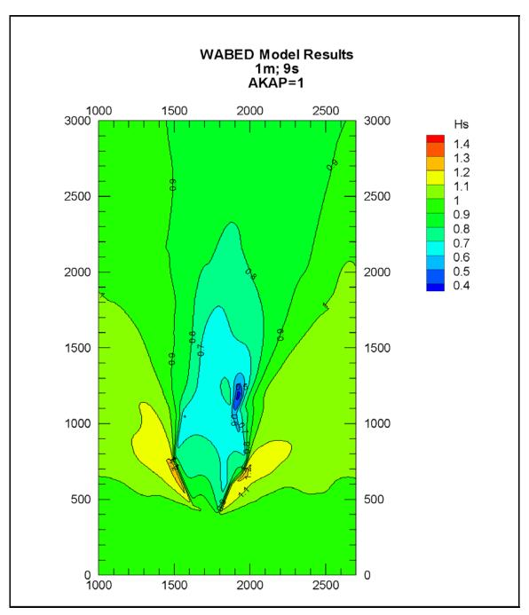
Figure 3.65 Colour Contour Plots of Significant Wave Height for  $T_p = 9$  s by WABED with Diffraction Coefficient of akap = 1(coordinates are in meters)
