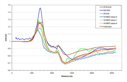
Figure 3.84 Wave Height Comparison for the 2000 m Cross Shore Line (12 s)
