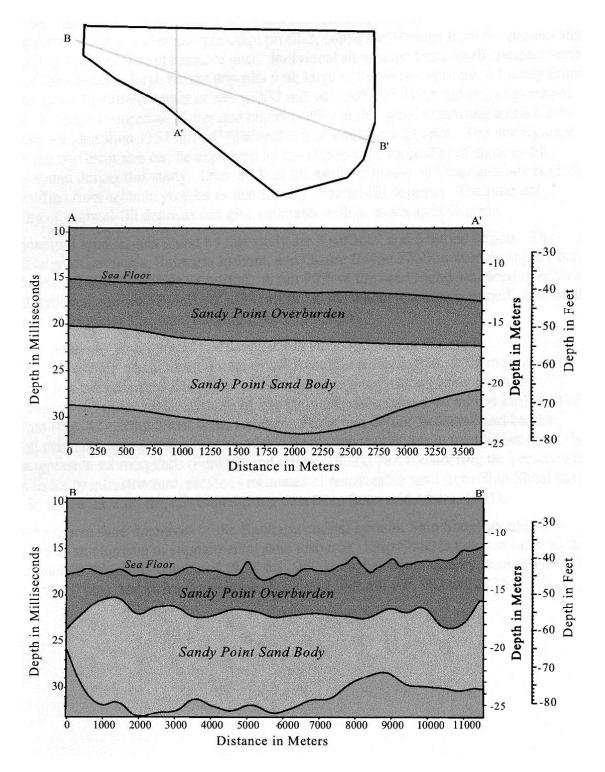
Figure 18. Schematic area map and lithostratigraphic framework model for the Sandy Point Borrow site. The upper polygon (top of figure) defines the area originally recognized by Kindinger et al. (2002) as a potential borrow site in the Barataria Bight. The approximate location of the polygon is shown in figure 1. The lower two diagrams provide schematic cross sections through the site, indicating the geometry, bounding surfaces and overburden (from Kindinger et al., 2002).
