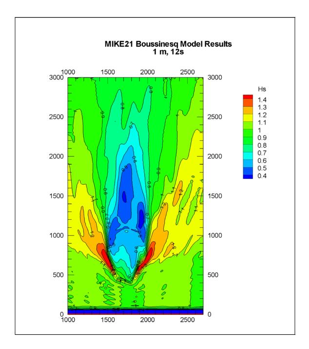
Figure 3.55 2D Map of Significant Wave Height from M21BW Results (Wave Condition: SSE, Hm0=1m, Tp=12s) and (coordinates are in meters)
