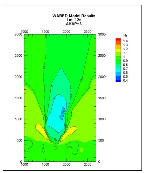
Figure 3.63 Colour Contour Plots of Significant Wave Height for  $T_p = 12$  s by WABED with Diffraction Coefficient of akap = 3(coordinates are in meters)
