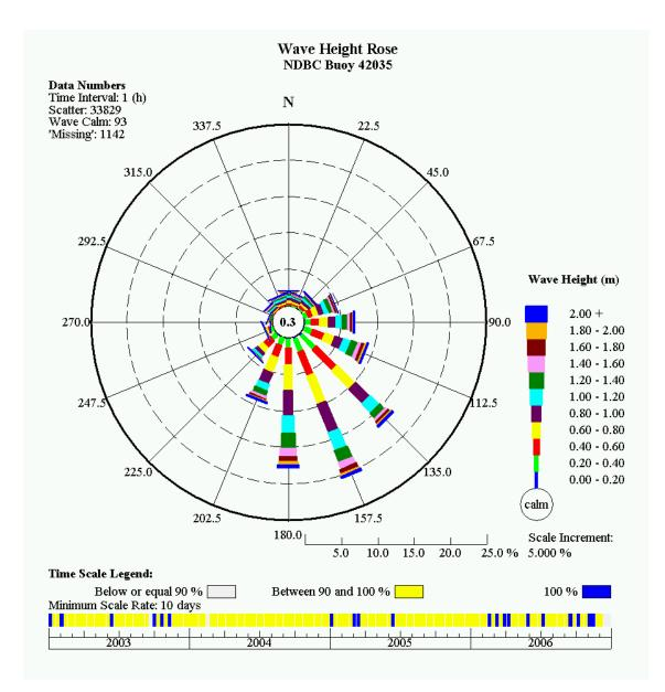
Figure 3.43 Wave Rose for Station NDBC42035 (2003 to 2006)
