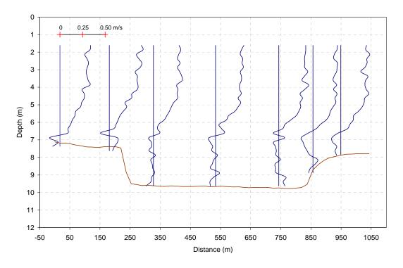
Figure B.2.7 Velocity Profiles for North-South Transect Line (File no. 10401)
