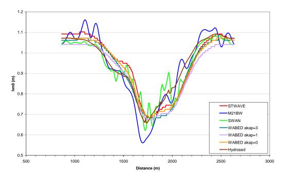
Figure 3.72 Wave Height Comparison for the 1500 m Alongshore Line (12 s)
