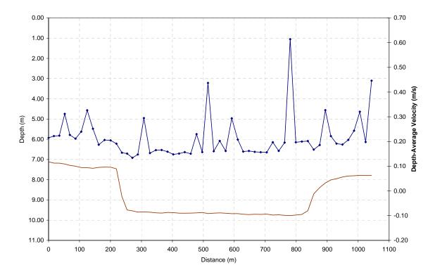
Figure B.2.28 Depth-Average Flow Velocity Change Across North-South Cross-Section (File no. 10401)
