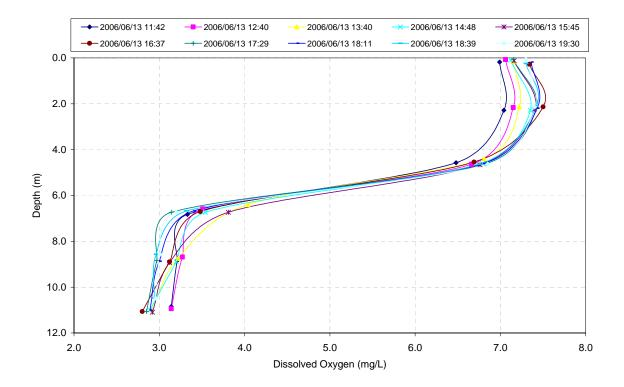
Figure 3.27 Site 2 Dissolved Oxygen Results Throughout Water Column
