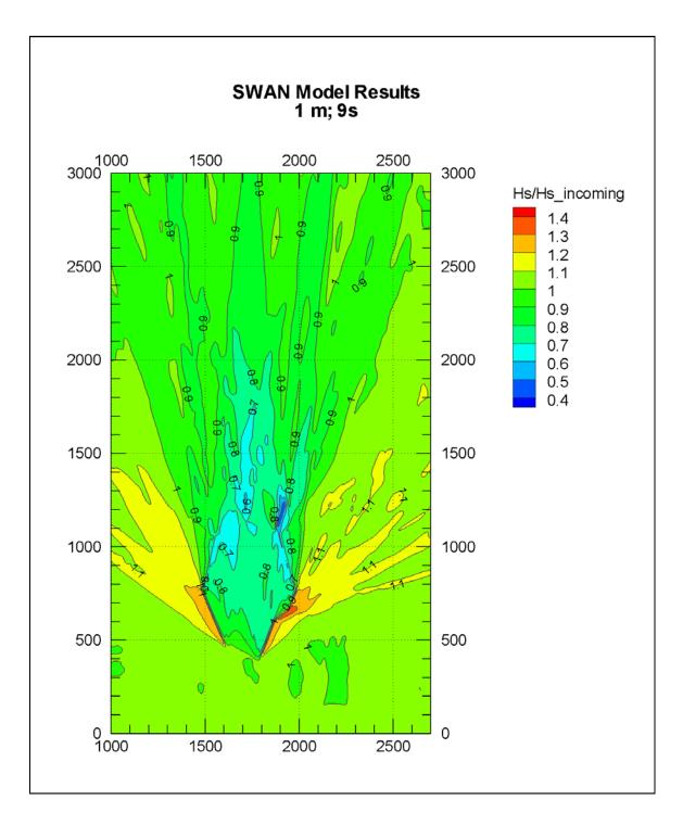
Figure 3.60 Colour Contour Plots of Significant Wave Height for Tp=9s by SWAN (coordinates are in meters)
