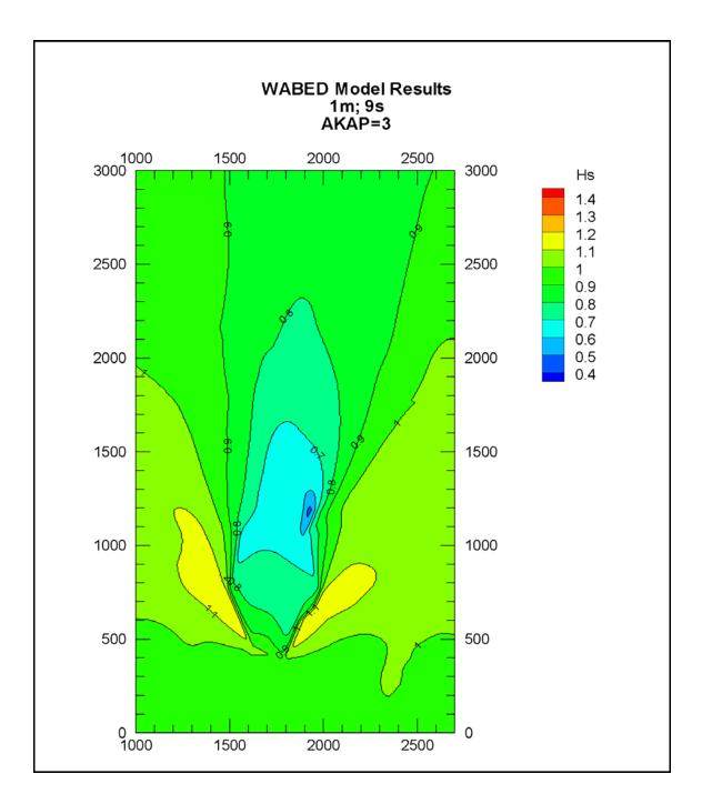
Figure 3.66 Colour Contour Plots of Significant Wave Height for  $T_p = 9$  s by WABED with Diffraction Coefficient of akap = 3(coordinates are in meters)
