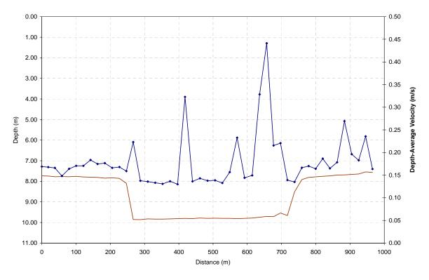
Figure B.2.30 Depth-Average Flow Velocity Change Across East-West Cross-Section (File no. 165500)
