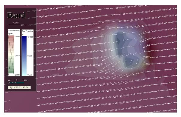
Figure 3.48c First Close-up of the Near Bed Flow Vectors Overlaid on the Suspended Sediment Concentration Map for the Higher Flow Condition
