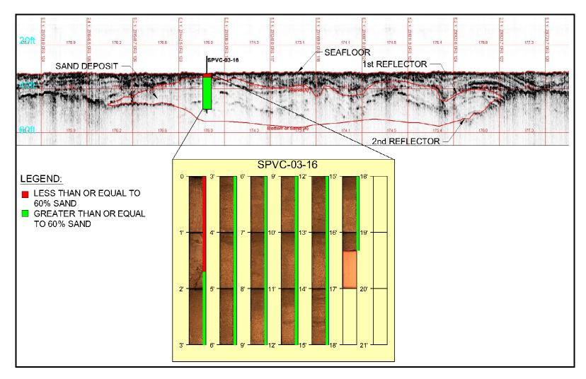
Figure 22. High-resolution seismic profile showing the subsurface geometry of the northwestern borrow site sand body and overburden. Location of cross section is shown in figure 19.
