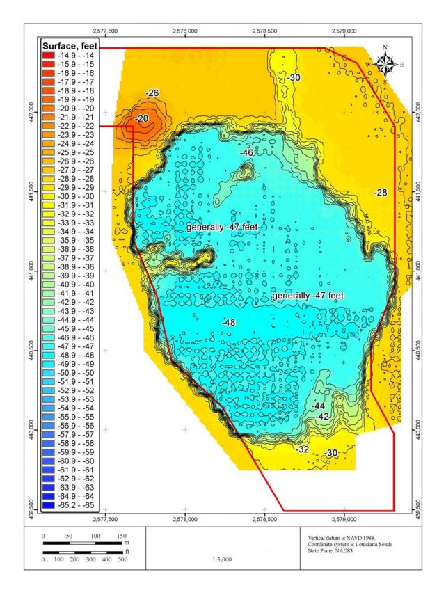
Figure 3.4 Holly Beach Dredge Pit – Bathymetry Dec. 2004 (20 Months After Dredging)
