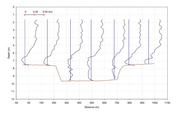
Figure B.2.15 Velocity Profiles for East-West Transect Line (File no. 3629)
