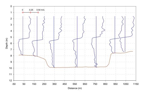
Figure B.2.3 Velocity Profiles for North-South Transect Line (File no. 162819)
