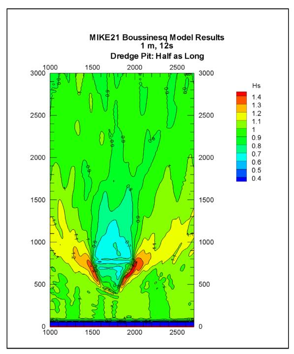
Figure 3.95 Distribution of Significant Wave Height from M21BW Results for the Half as Long Dredge Pit (wave conditions same as Figure 3.92 and coordinates are in meters)
