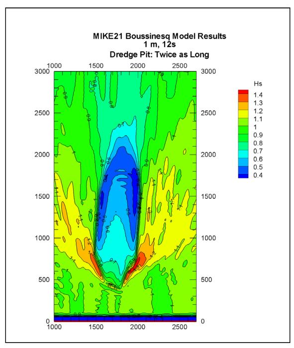
Figure 3.96 Distribution of Significant Wave Height from M21BW Results for the Twice as Long Dredge Pit (wave conditions same as Figure 3.92 and coordinates are in meters)
