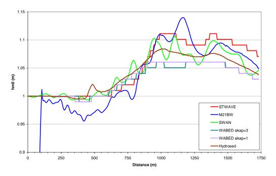
Figure 3.86 Wave Height Comparison for the 1000 m Cross Shore Line (9 s)
