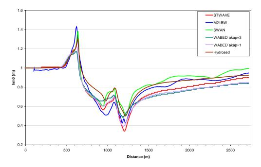
Figure 3.89 Wave Height Comparison for the 1930 m Cross Shore Line (9 s)
