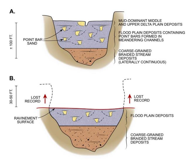
**FIGURE 8.** Stratigraphic cross-sections for the lowstand valley of the piedmont river illustrated in Figure 6 (during present highstand of sea level).
