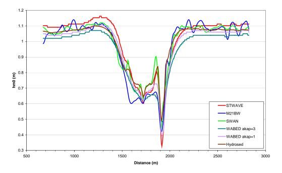
Figure 3.76 Wave Height Comparison for the 1170 m Alongshore Line (9 s)
