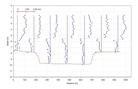
Figure 3.19 Representative Velocity Profiles for East-West Transect Line (05-Mar-2007 20:33-20:40 CST)
