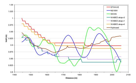
Figure 3.74 Wave Height Comparison for the 2500 m Alongshore Line (12 s)
