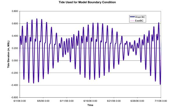
Figure 3.38 Tide Levels Used in the Model Calibration
