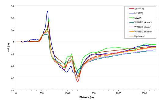
Figure 3.83 Wave Height Comparison for the 1930 m Cross Shore Line (12 s)
