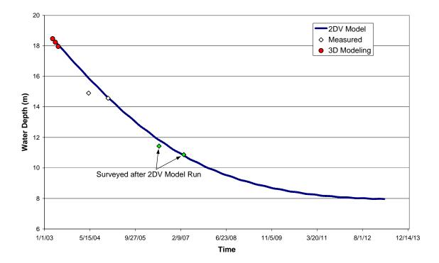
Figure 3.46a Measured and Predicted Water Depth within the Holly Beach Dredge Pit Showing the Rate of Pit Infilling
