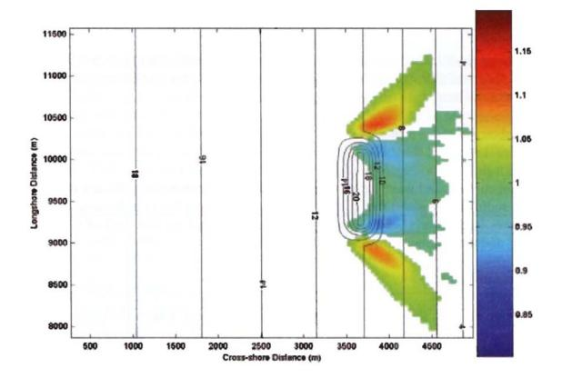
Figure 2.3 Ratio of Computed Wave Height of Baseline Pit Case and Reference Pit Case (without pit) (pit at 10 m depth contour; offshore wave: H<sub>s</sub>=3.36 m, T<sub>p</sub>=8.8 s, Dir=270 °; coast on right side) Figure courtesy of van Rijn et al (2005). SANDPIT. Figure 7.3.5, p.99
