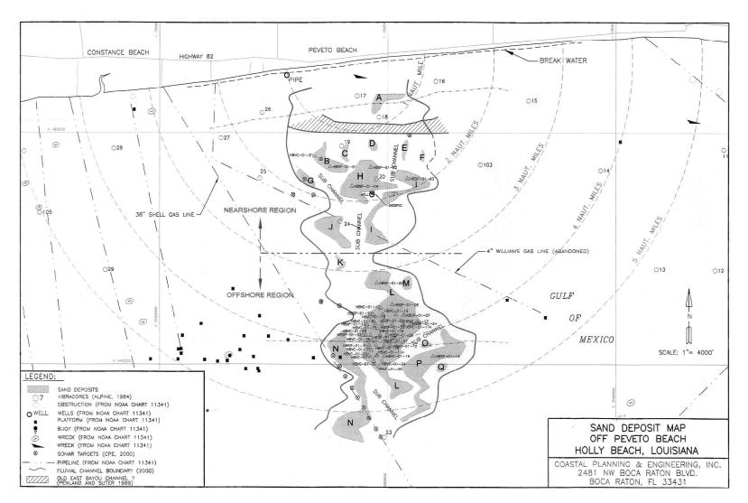
Figure 13. Base map of the primary sand bodies in the Pevoto channel system. CPE (2002) labeled these bodies as A to O and focused primarily on the unit L (south-central location) for additional detailed investigations as a borrow target.
