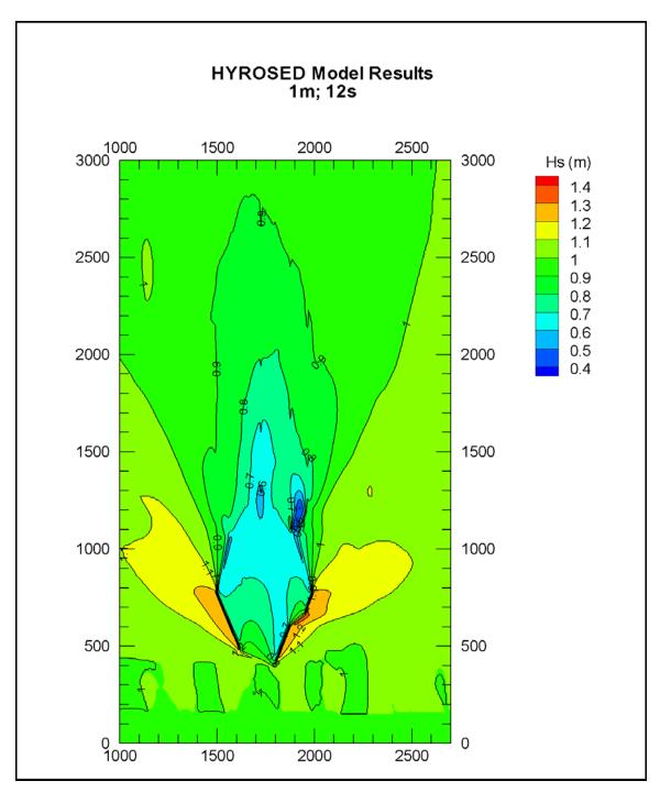
Figure 3.67 Colour Contour Plots of Significant Wave Height for Tp=12s by HYDROSED (coordinates are in meters)
