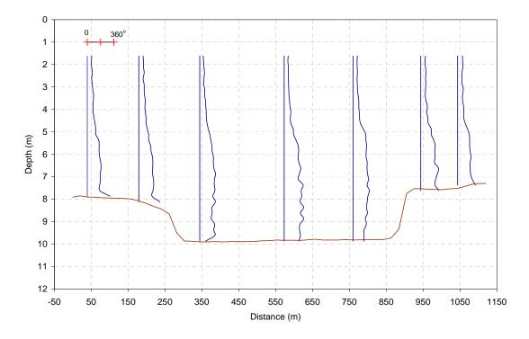
Figure B.2.4 Direction Profiles for North-South Transect Line (File no. 162819)
