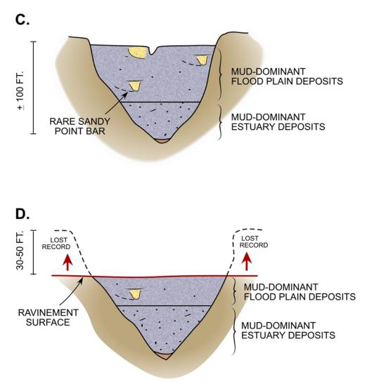
**FIGURE 9.** Stratigraphic cross-sections for the lowstand valley of the coastal plain river illustrated in Figure 6 (during present highstand).
