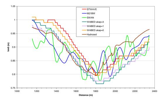
Figure 3.73 Wave Height Comparison for the 2000 m Alongshore Line (12 s)
