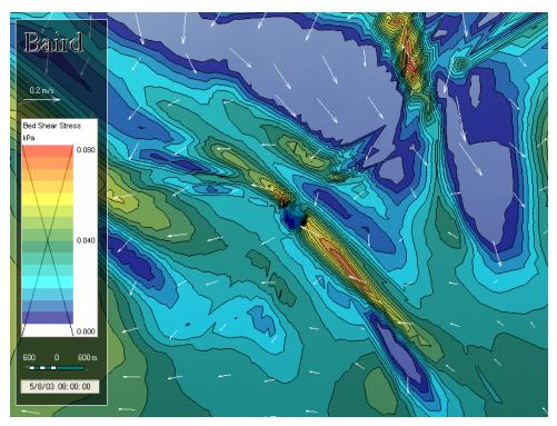
Figure 3.49a Near Bed Flow Vectors Overlaid on the Bed Shears Stress Map for the Full Model Domain and Complicated Combined Condition
