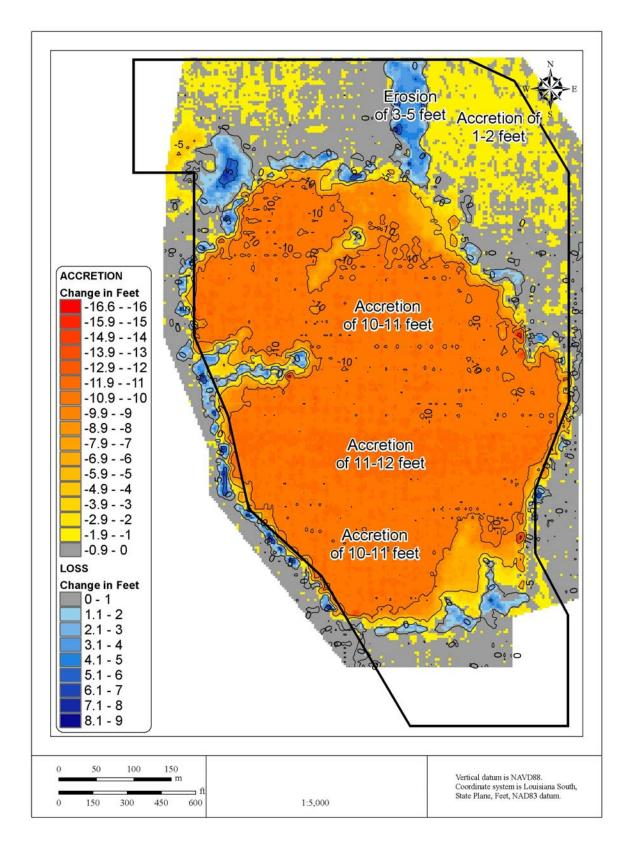
Figure 3.6 Seafloor Surface Elevation Change December 2004 to June 2006
