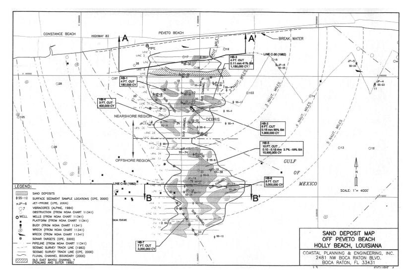
Figure 9. Base map of the sand-rich strata within the Pevoto Channel. Note the distribution of the sand bodies relative to the distribution of sub-channels as defined by CPE (2002). Lines of cross section A-A' and B-B' correspond to the location of figures 11 and 12, respectively.
