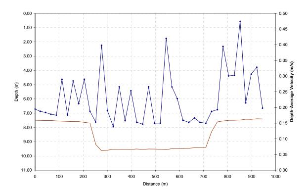
Figure B.2.31 Depth-Average Flow Velocity Change Across East-West Cross-Section (File no. 190058)
