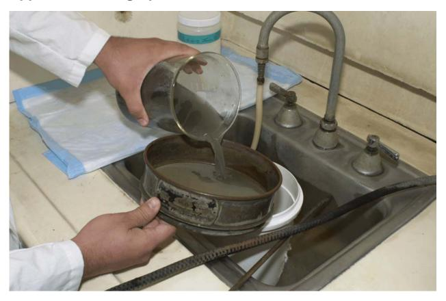
Figure A1 Sieving sediment on a 0.5 mm sieve
