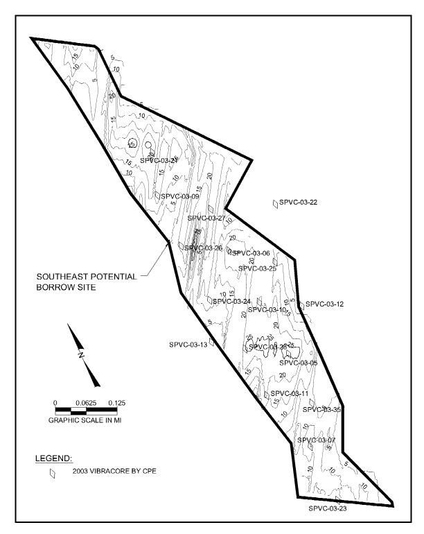
Figure 24. Isopach map of the sand body within the southeast borrow area. Contours are in feet.
