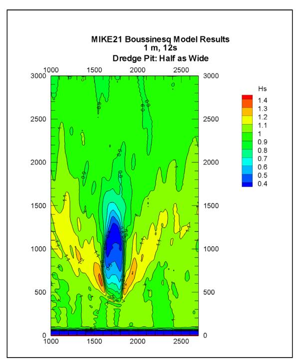
Figure 3.97 Distribution of Significant Wave Height from M21BW Results for the Half as Wide Dredge Pit (wave conditions same as Figure 3.92 and coordinates are in meters)
