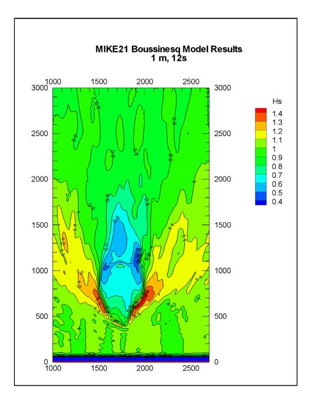
Figure 3.92 Distribution of Significant Wave Height from M21BW Results for Immediate Post-Dredge Depth of 18 m (Wave Condition: SSE, Hm0=1m, Tp=12 s and coordinates are in meters)
