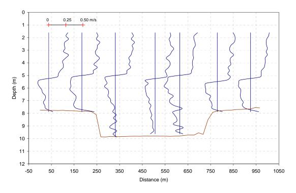
Figure B.2.11 Velocity Profiles for East-West Transect Line (File no. 165500)
