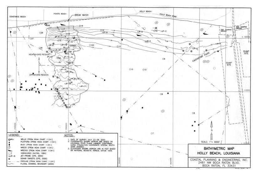
Figure 10. Base map of the Pevoto Channel showing the bathymetry of the study site. Contours are shown in feet NGVD 29.
