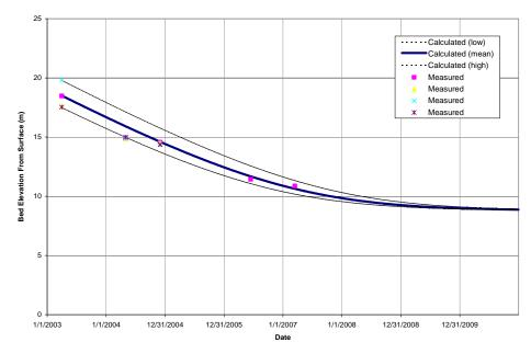
Figure 3.50 The Estimated Water Depth in the Pit Using the Analytical Solution (Equation 3.7)
