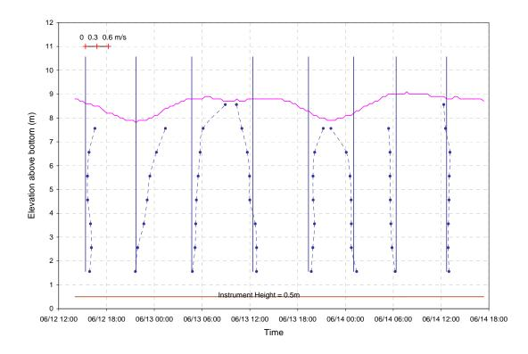
Figure 3.15 Current Velocity Profiles at Site 7 (beyond the area influenced by the pit), June 2006
