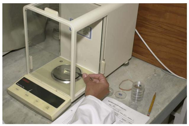
Figure A3 Weighing aluminum trays for biomass measurements
