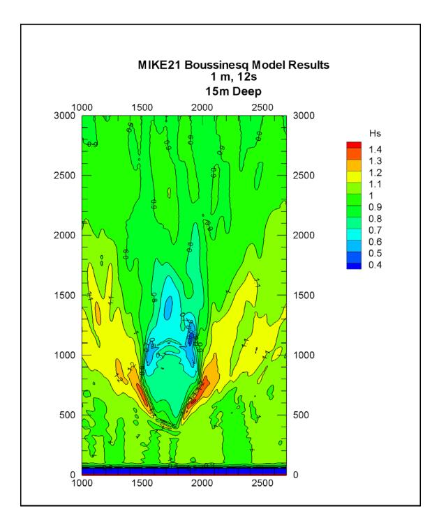
Figure 3.94 Distribution of Significant Wave Height from M21BW Results for a 15 m Dredge Pit (wave conditions same as Figure 3.92 and coordinates are in meters)
