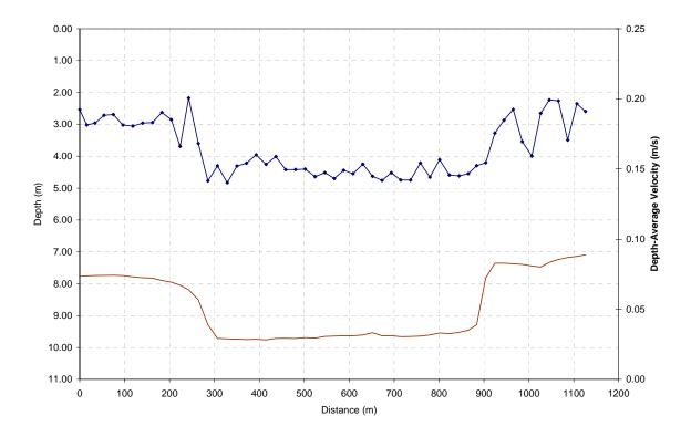
Figure B.2.27 Depth-Average Flow Velocity Change Across North-South Cross-Section (File no. 183610)
