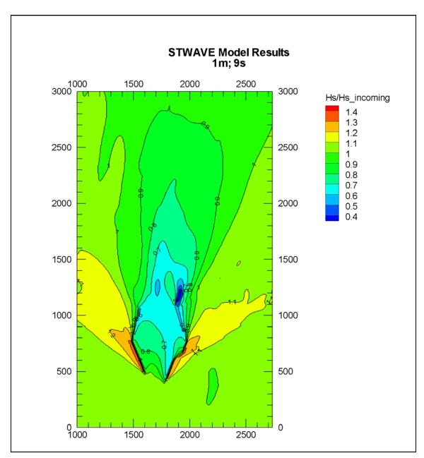
Figure 3.58 Colour Contour Plots of Significant Wave Height for Tp=9s by STWAVE (coordinates are in meters)
