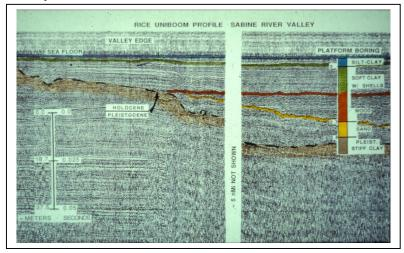
Figure 4. Seismic profile across the ancestral Sabine River valley. The chaotic seismic facies in the base of the valley is fluvial sand and gravel that was sampled by the platform boring shown in this figure.
