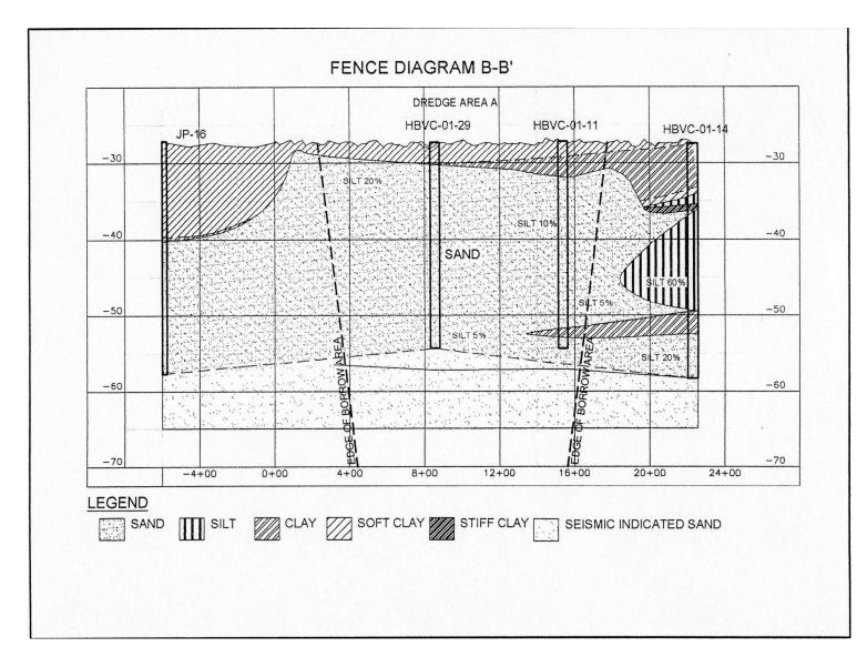
Figure 16. Lithostratigraphic cross section B-B' across sand body L. Location of cross section shown in figure 14. Note the variation in facies composition and thickness as compared to figure 15.
