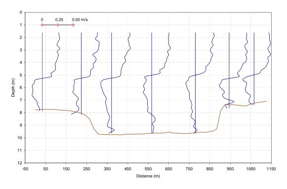
Figure B.2.5 Velocity Profiles for North-South Transect Line (File no. 183610)
