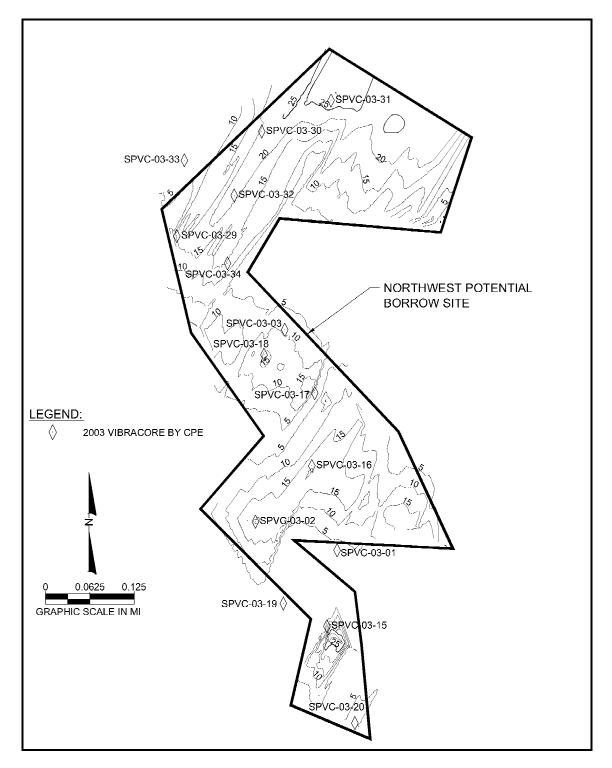
Figure 21. Isopach map of the sand body within the northwest borrow area of the Sandy Point site. Contours are in feet.
