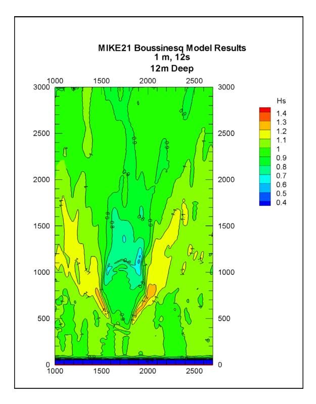
Figure 3.93 Distribution of Significant Wave Height from M21BW Results for a 12 m Dredge Pit (wave conditions same as Figure 3.92 and coordinates are in meters)
