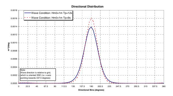
Figure 3.53 Directional Spectra for 9s and 12s Wave Conditions
