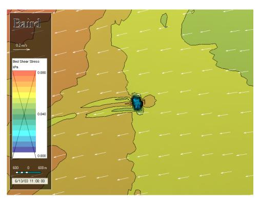
Figure 3.48a Near Bed Flow Vectors Overlaid on the Bed Shears Stress Map for the Full Model Domain and the Higher Flow Condition
