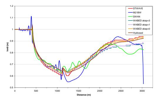
Figure 3.82 Wave Height Comparison for the 1750 m Cross Shore Line (12 s)
