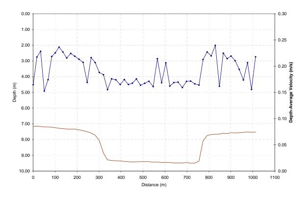
Figure B.2.36 Depth-Average Flow Velocity Change Across Diagonal Cross-Section (File no. 233424)
