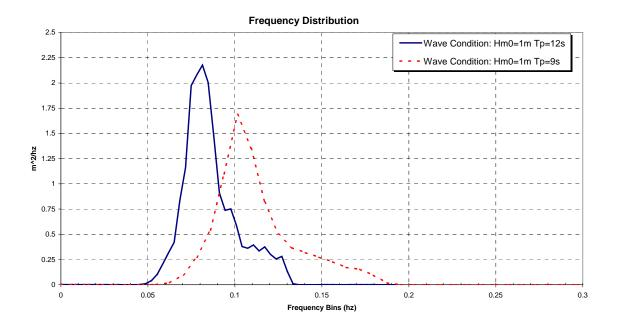
Figure 3.54 Frequency Spectra for 9s and 12s Wave Conditions
