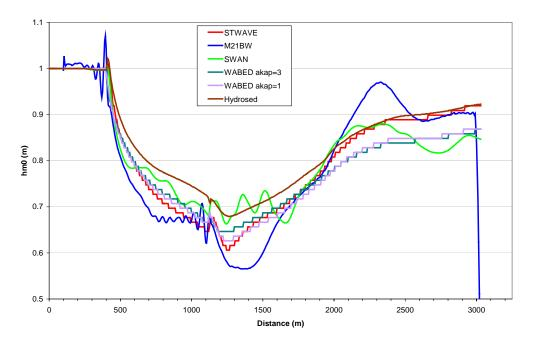
Figure 3.88 Wave Height Comparison for the 1750 m Cross Shore Line (9 s)
