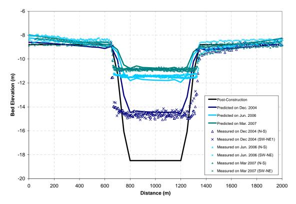
Figure 3.46b Measured and Predicted (2DV Model) Pit Infilling and Pit Margin Erosion for the Holly Beach Dredge Pit
