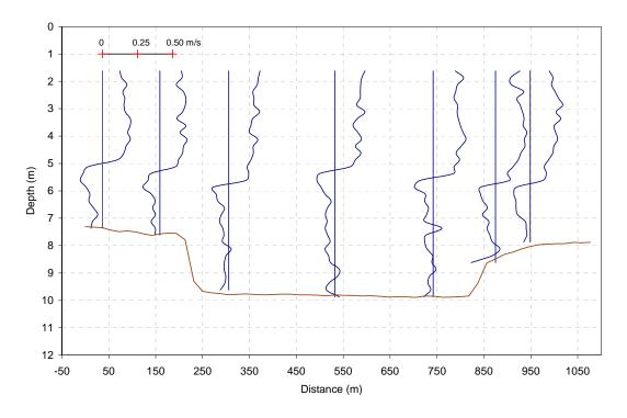
Figure B.2.1 Velocity Profiles for North-South Transect Line (File no. 143243)
