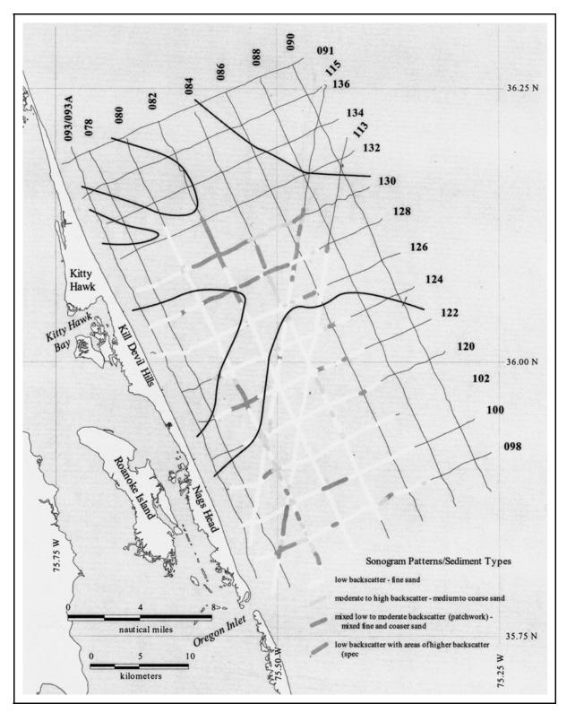
**FIGURE 11** Distribution of the main side-scan sonar signatures seen in a portion of the inner continental shelf in the Kitty Hawk, NC area. The heavy lines in the upper half of the diagram locate the boundaries of a major lowstand valley. From Boss et al. (1999).
