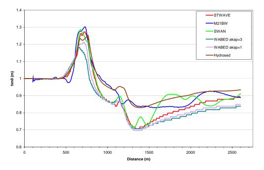
Figure 3.90 Wave Height Comparison for the 2000 m Cross Shore Line (9 s)
