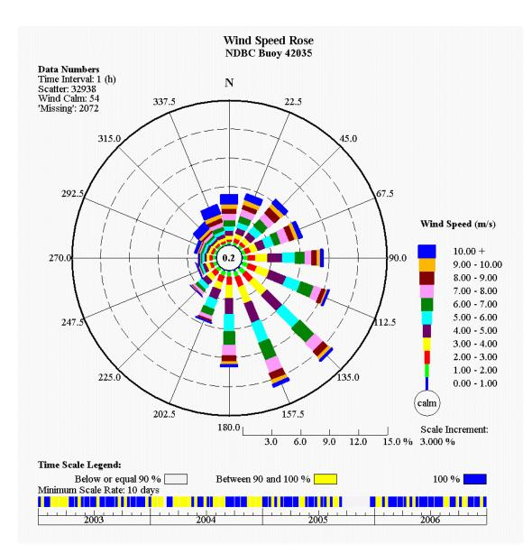
Figure 3.42 Wind Rose for Station NDBC42035 (2003 to 2006)
