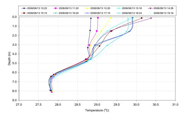
Figure 3.33 Site 7 Temperature Results Throughout Water Column
