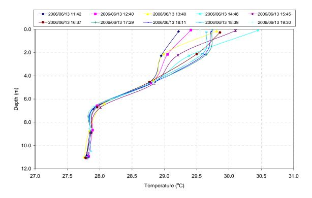
Figure 3.28 Site 2 Temperature Results Throughout Water Column
