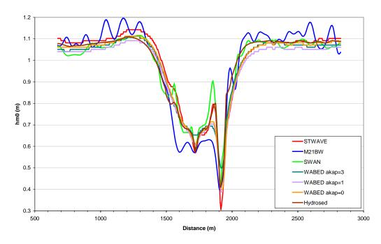
Figure 3.71 Wave Height Comparison for the 1170 m Alongshore Line (12 s)
