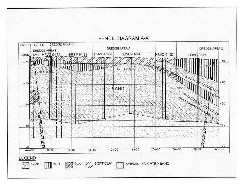
Figure 15. Lithostratigraphic cross section A-A' across sand body L. Location of cross section shown in figure 14. Variability in thickness of the silty and clayey overburden exists along this line but generally ranges between 1 and 3 m (0.3 and 9 ft).
