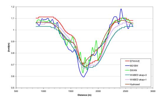
Figure 3.77 Wave Height Comparison for the 1500 m Alongshore Line (9 s)
