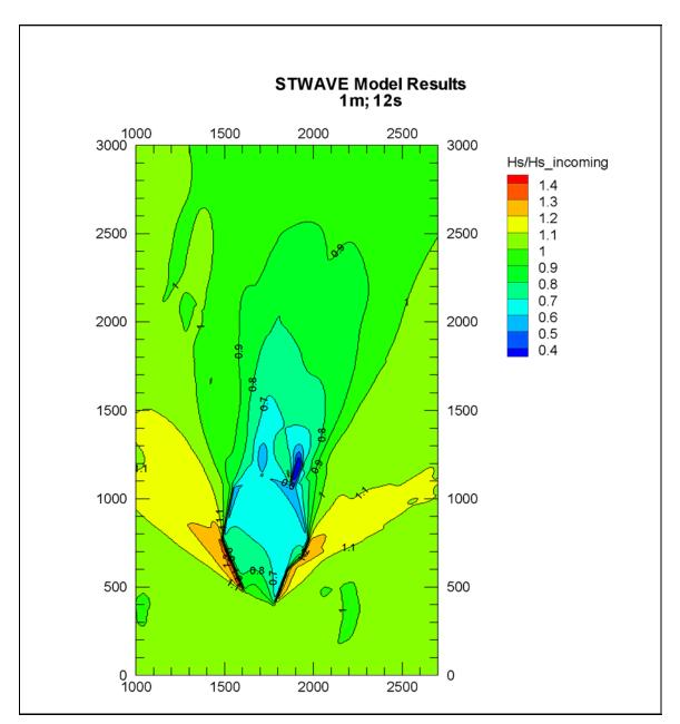
Figure 3.57 Colour Contour Plots of Significant Wave Height for Tp=12s by STWAVE (coordinates are in meters)
