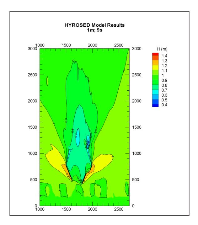
Figure 3.68 Colour Contour Plots of Significant Wave Height for Tp=9s by HYDROSED (coordinates are in meters)
