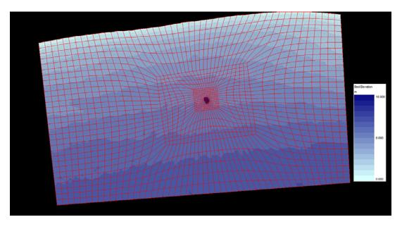
Figure 3.37 Grid Used for 3D Morphological Modeling
