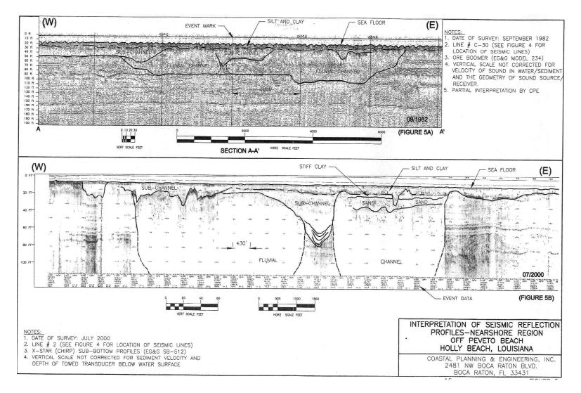
Figure 11. High-resolution seismic profiles across the northern part of the Pevoto channel showing the subsurface geologic framework of the fluvial sedimentary bodies and stratigraphic characteristics of the overburden. Upper seismic profile is from investigations conducted by the U.S. Geological Survey in the 1980's and lower profile is from CPE (2002) approximately across the same location. Location of profile is shown in figure 9.
