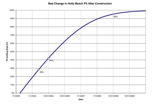
Figure 3.51 Predicted Infilling of the Pit in Terms of Percent Full Using the Analytical Solution ( Equation 3.8)
