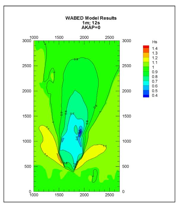
Figure 3.61 Colour Contour Plots of Significant Wave Height for  $T_p = 12s$  by WABED with Diffraction Coefficient of akap = 0(coordinates are in meters)
