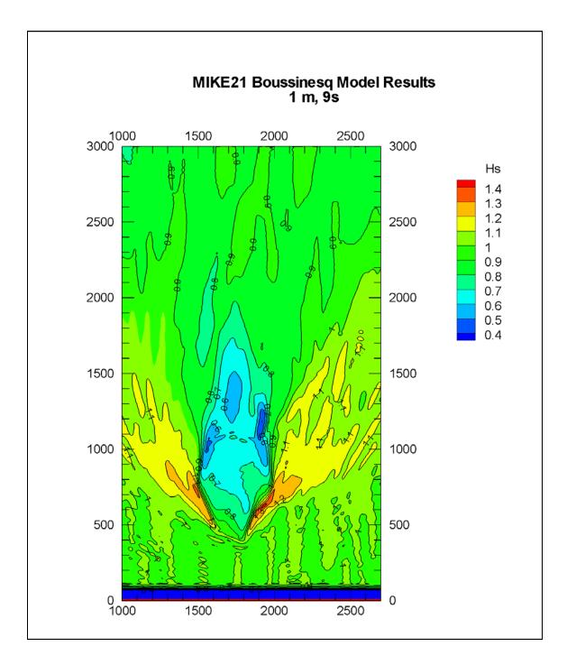
Figure 3.56 2D Map of Significant Wave Height from M21BW Results (Wave Condition: SSE, Hm0=1m, Tp=9s) and (coordinates are in meters)
