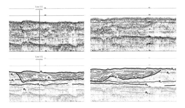
**FIGURE 17.** Seismic reflection profile across a lowstand valley off Kitty Hawk, North Carolina. The plan view outline of the valley is shown on the map in Figure 11. From Boss and Hoffman (2001).
