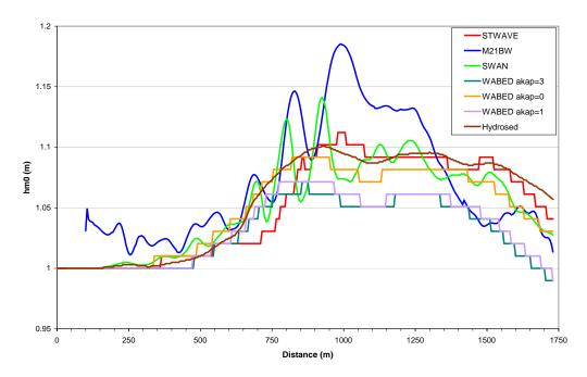
Figure 3.85 Wave Height Comparison for the 2500 m Cross Shore Line (12 s)
