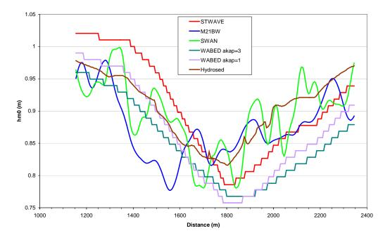
Figure 3.78 Wave Height Comparison for the 2000 m Alongshore Line (9 s)
