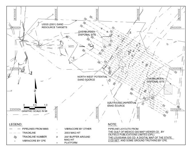
Figure 19. Base map of the Sandy Point borrow site defined by Kindinger et al. (2002) (light gray outer polygon). Within this polygon CPE (2002) defined a northwest and southeast borrow site using vibracores and high-resolution seismic profiles.
