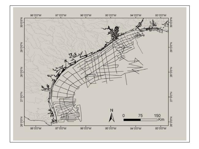
Figure 1. Track lines of high-resolution seismic data used to map fluvial channels on the Texas continental shelf.
