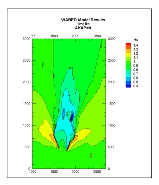
Figure 3.64 Colour Contour Plots of Significant Wave Height for  $T_p = 9$  s by WABED with Diffraction Coefficient of akap = 0(coordinates are in meters)
