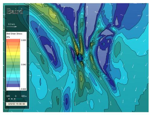
Figure 3.49b Near Bed Flow Vectors Overlaid on the Bed Shears Stress Map for the Full Model Domain and Complicated Combined Condition
