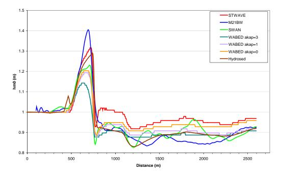
Figure 3.81 Wave Height Comparison for the 1500 m Cross Shore Line (12 s)
