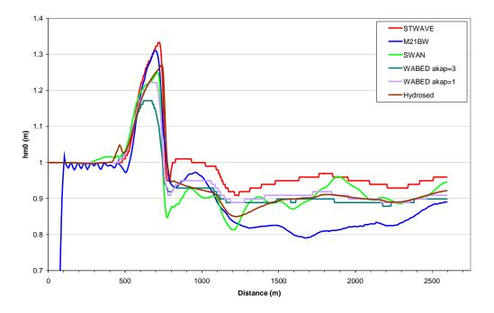
Figure 3.87 Wave Height Comparison for the 1500 m Cross Shore Line (9 s)
