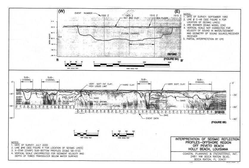
Figure 12. High-resolution seismic profiles across the southern part of the Pevoto channel showing the subsurface geologic framework of the fluvial sedimentary bodies and stratigraphic characteristics of the overburden. Upper seismic profile is from investigations conducted by the U.S. Geological Survey in the 1980's and lower profile is from CPE (2002) approximately across the same location. Location of profile is shown in figure 9.
