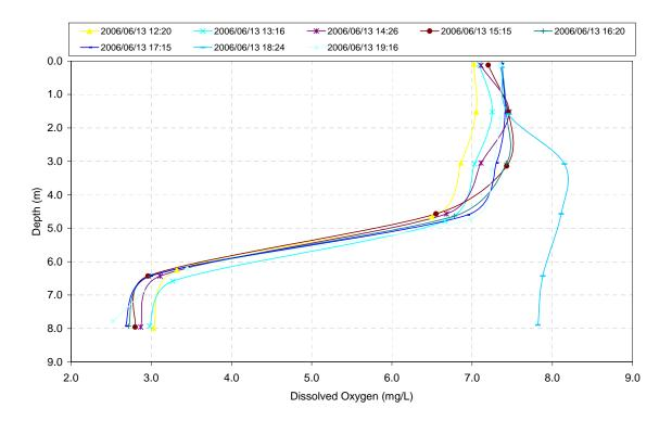
Figure 3.32 Site 7 Dissolved Oxygen Results Throughout Water Column
