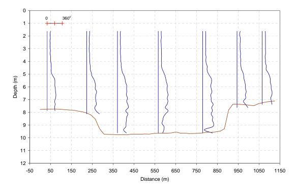
Figure B.2.6 Direction Profiles for North-South Transect Line (File no. 183610)
