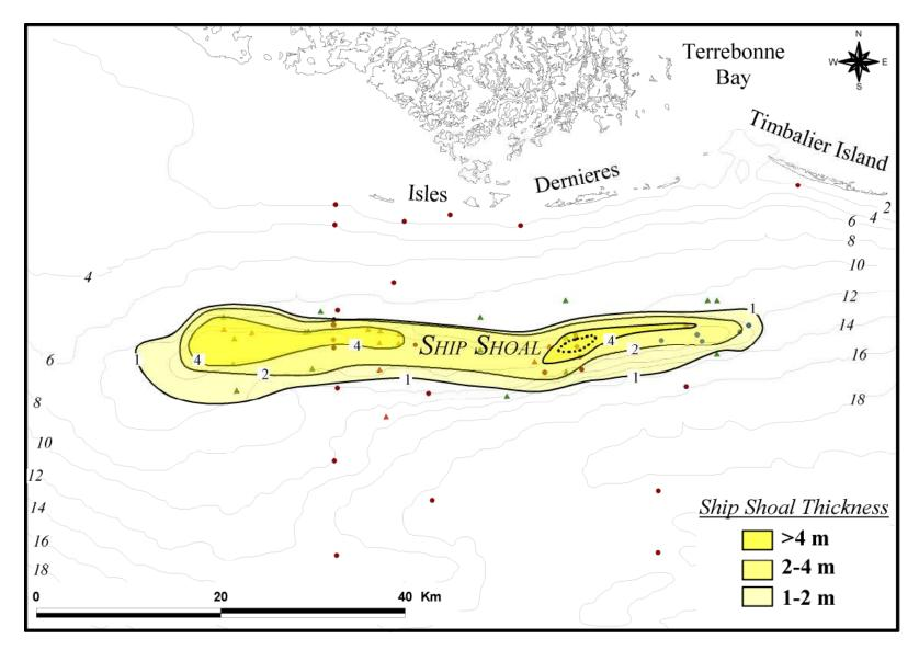
Figure 27. Isopach map of the Ship Shoal offshore sandy deposit with bathymetry (from Kulp et al., 2005).
