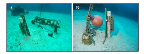
Figure 3.6.4. YSI and Seabird units partially buried in sand at the (A) EFGB and (B) WFGB long-term monitoring sites in October 2008. Photographs from Hickerson (2008b).
