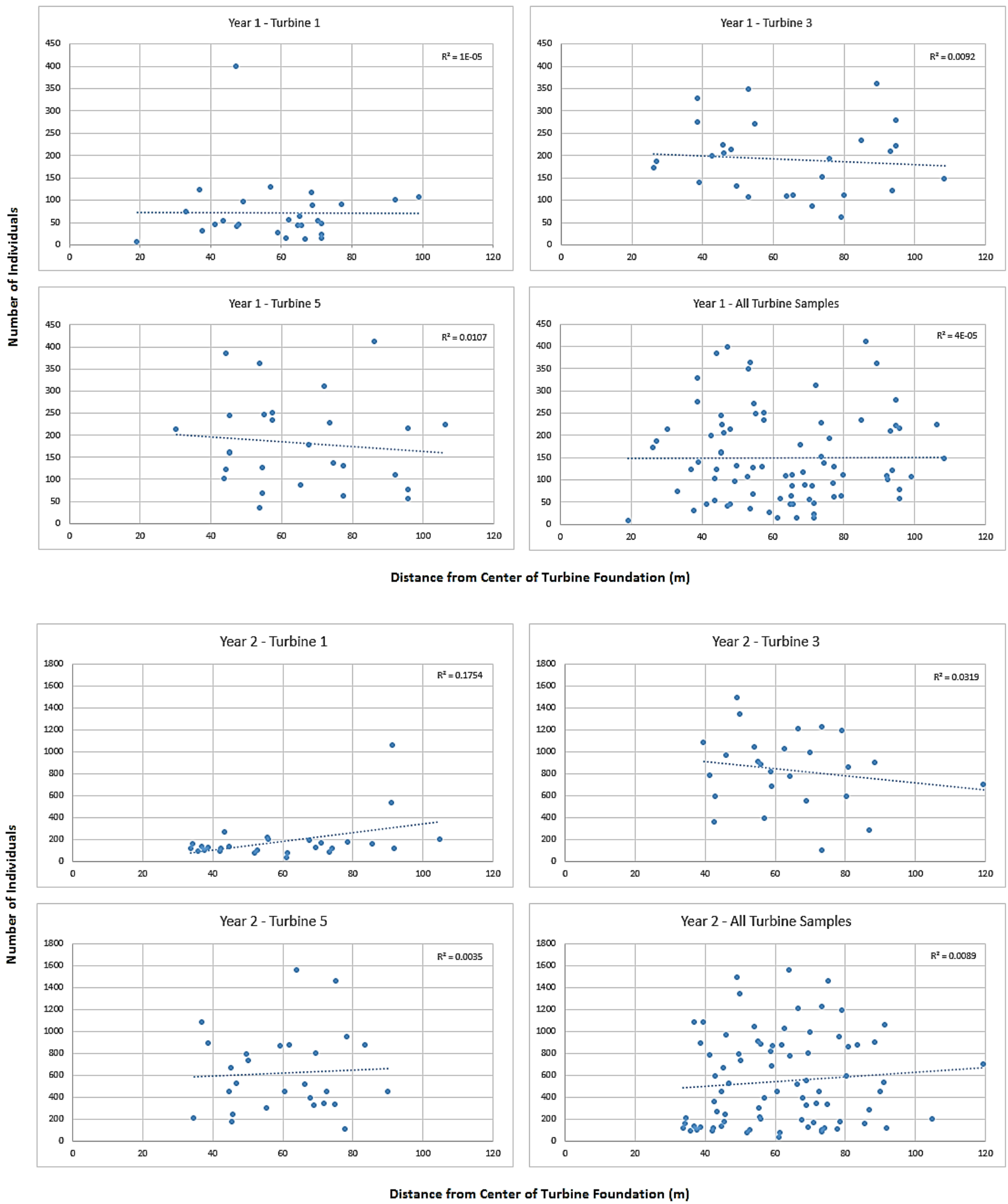
Figure 36. Number of individuals per vessel-based grab sample with distance from the center point under each turbine foundation structure for Year 1 and Year 2.
