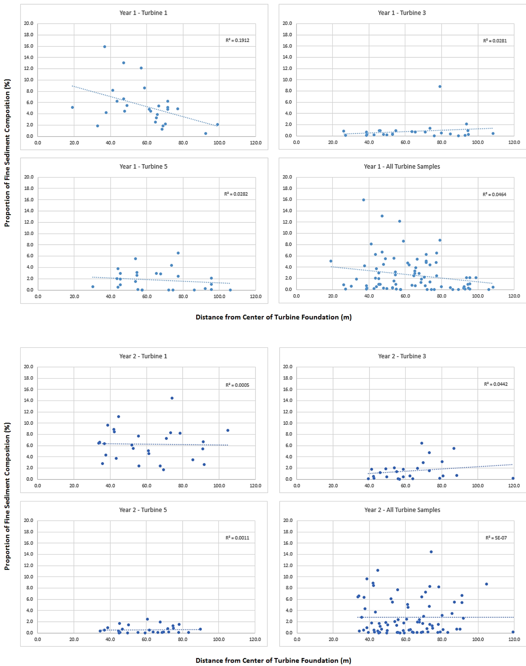
Figure 18. Proportion of fine sediment (particles <250 \mu\text{m} diameter) from vessel-based sediment samples with distance from the center point under each turbine foundation structure at BIWF for Year 1 and Year 2.
