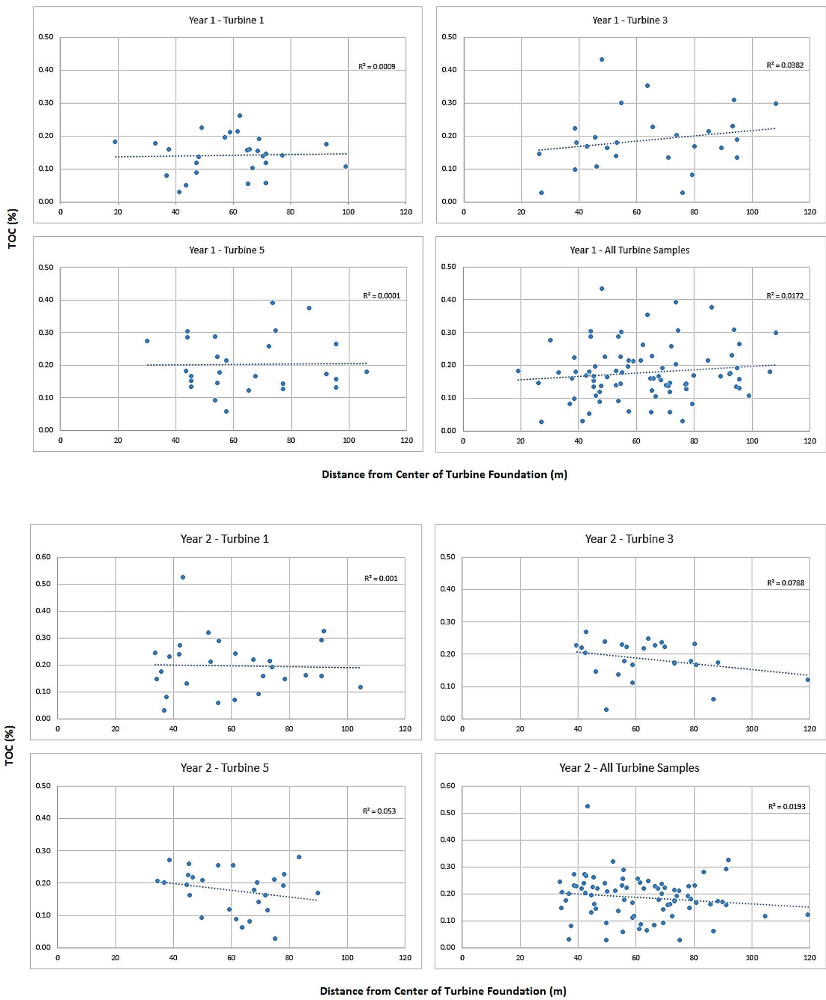
Figure 22. Levels of TOC in vessel-based sediment samples plotted against distance from the center point under each turbine foundation structure at BIWF for Year 1 and Year 2.
