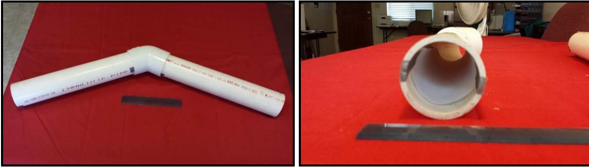
Figure 4. Scat tube (left) with 15-cm ruler for scale, and entrance to scat tube (right) with paper to collect Buena Vista Lake shrew scats.
