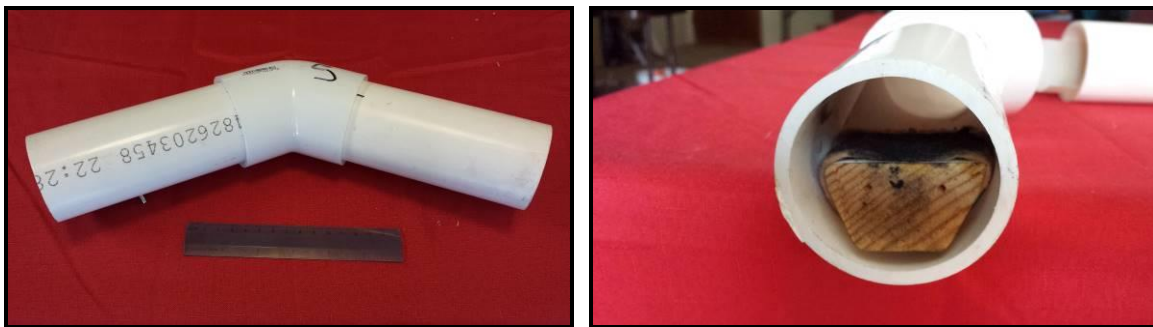
Figure 3. Track tube (left) with 15-cm ruler for scale, and wooden block with felt ink pad in entrance (right).
