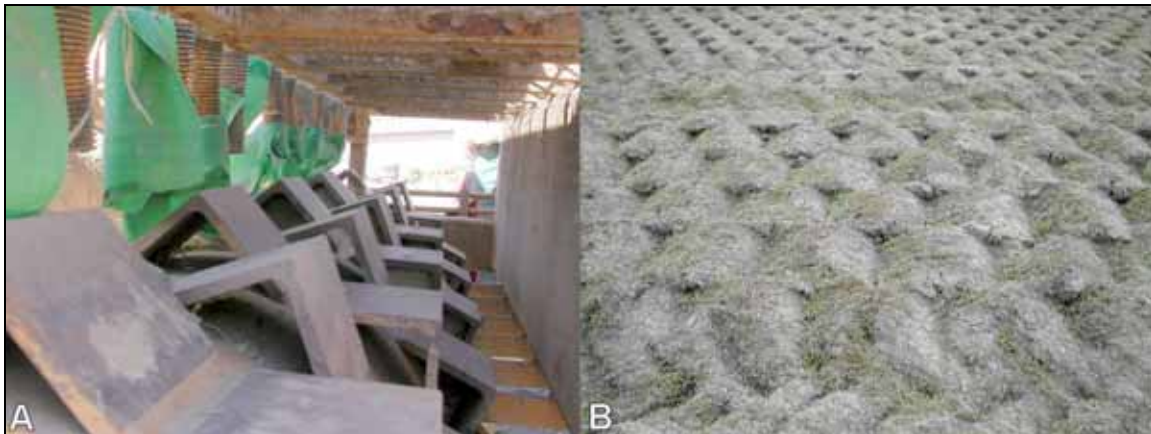
Figure 13. A. Close-up of the teeth on the LRDP imprinter. B. a series of imprints in the clay soil at the Tranquillity project site.
