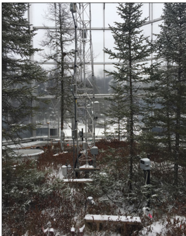
Fig. 16. Spruce and Peatland Responses Under Climatic and Environmental Change (SPRUCE) Project Site. Interior of a SPRUCE open-topped warming enclosure showing natural snow accumulation during a mid-winter precipitation event in Minnesota. [Image courtesy Oak Ridge National Laboratory]
