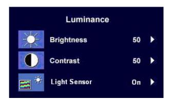
Press the  $\blacktriangleleft$  or  $\blacktriangleright$  keys to adjust the degree of **Brightness**.
