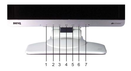
There are 7 keys for user's control including "Enter", "◀", "▶", "Exit", "Mode", "*iKey*" and a power switch. The following descriptions are the introduction of these keys & switch.
