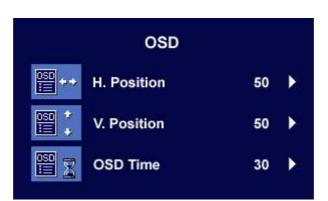
Press the ◀ or ▶ keys to adjust the **Horizontal Position** of the OSD. Press the **Exit** key to return to previous menu.
