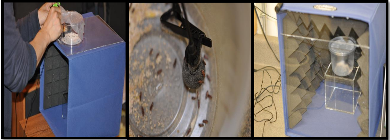
Figure. 4.5. An insulated box with a plexiglass served as the initial recording chamber, using a commercially available microphone and T. castaneum as a sample organism.
