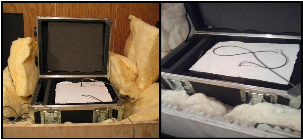
Figure. 4.4. Acoustic chamber used for dampening background sound while simultaneously recording two different FFT's, the background and the ambrosia beetle activity.
