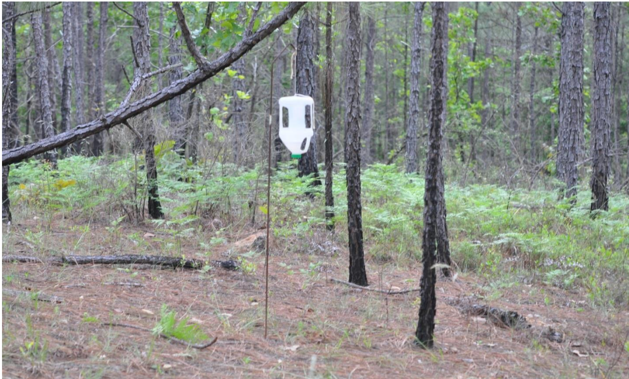
Figure 2.1. A Baker bottle trap design was used for testing the attractiveness of varying ratios of ethanol and methanol to ambrosia beetles.
