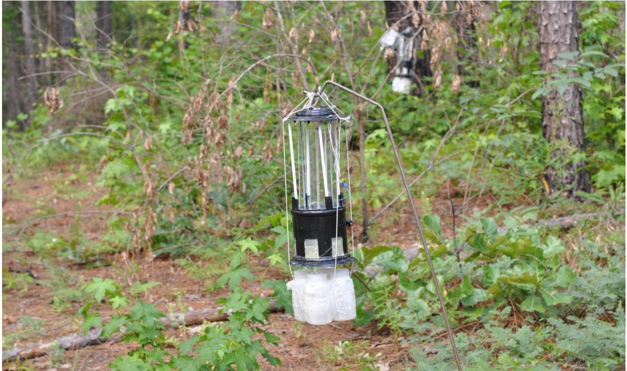
Figure 2.2. An improved bottle trap for testing the attractiveness of volatile cues and various light emitting diode (LED) wavelengths, including 395 nm (UV), 470 nm (blue), 525 nm (green),
