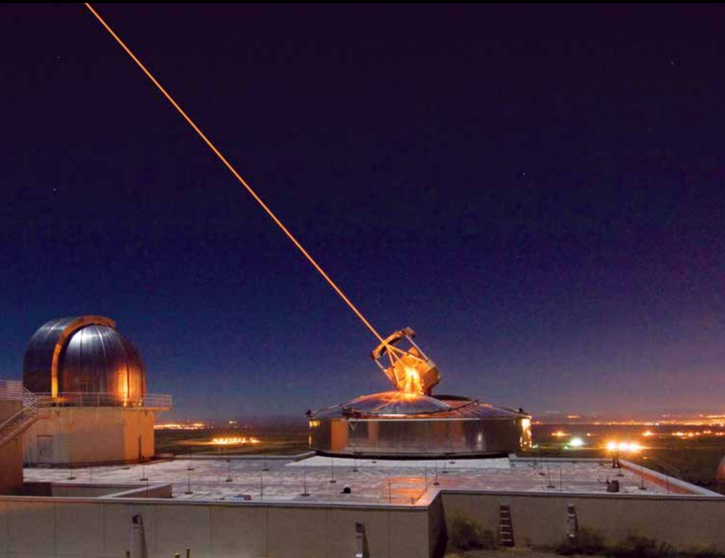
The Sodium Guidestar at the Air Force Research Laboratory Directed Energy Directorate's Starfire Optical Range. Researchers with AFRL use the Guidestar laser for real-time, high-fidelity tracking and imaging of satellites too faint for conventional adaptive optical imaging systems. The SOR's world-class adaptive optics telescope is the second largest telescope in the Department of Defense. (Courtesy photo)
