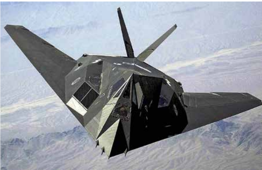
The F-117A NIGHTHAWK, the first operational stealth aircraft
