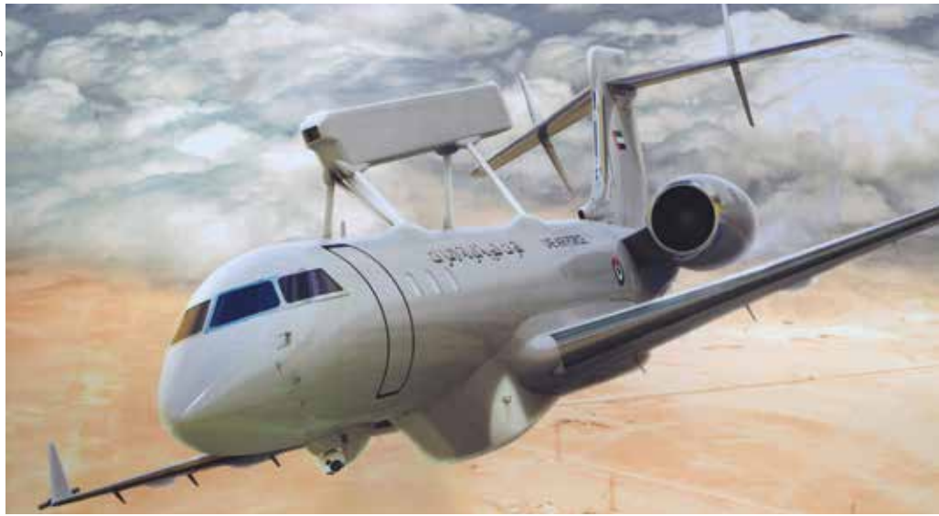
GLOBAL EYE AEW&C from Saab provides air, maritime and ground surveillance. It combines a new extended range radar with the ultra-long range GLOBAL 6000 jet aircraft from Bombardier.
