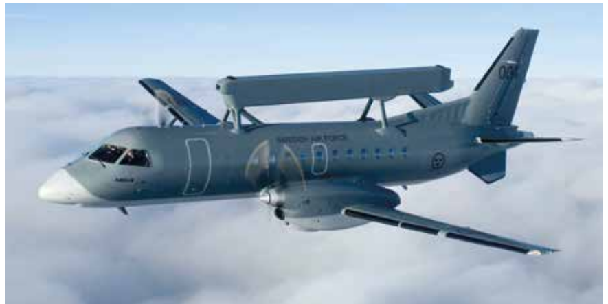
Saab's ERIEYE system, produced since 1996, was the first compact, 360-degree AESA radar system to be mounted on an aircraft.
