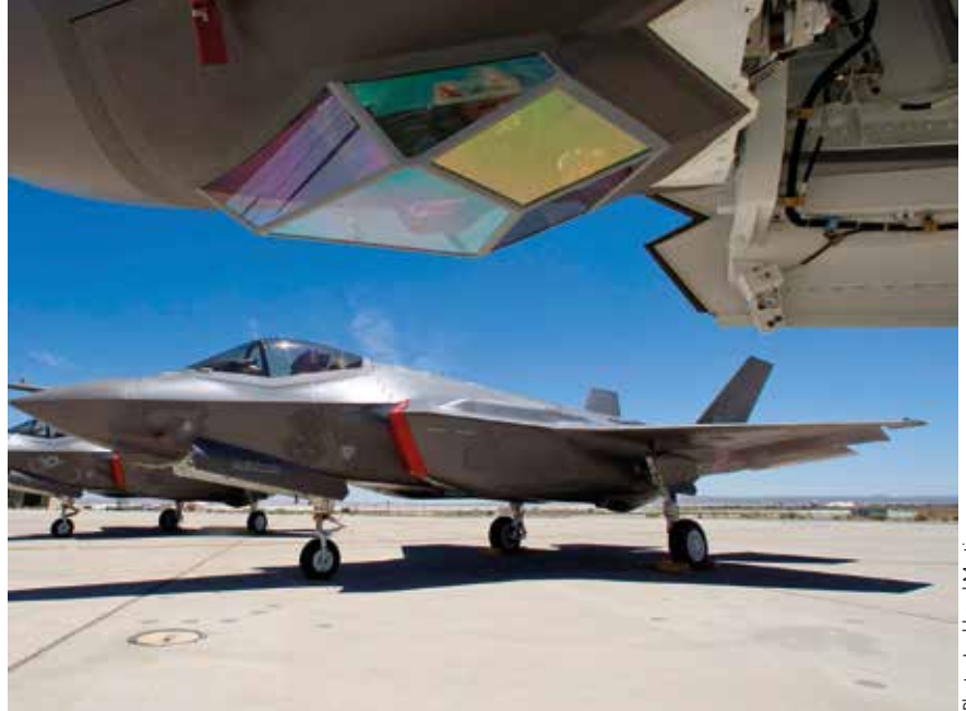
The sensors of the EOTS (Electro-Optical Targeting System) on the F-35
