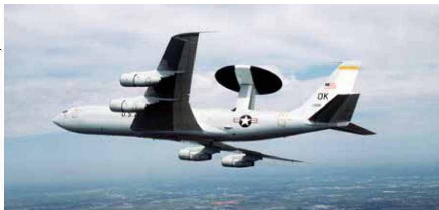
An E-3 SENTRY aircraft from Tinker Air Force Base, Oklahoma. The E-3 SENTRY is a modified Boeing 707/320 with a rotating radar dome that permits surveillance from the Earth's surface up into the stratosphere. The radar has a range of more than 200 miles.
