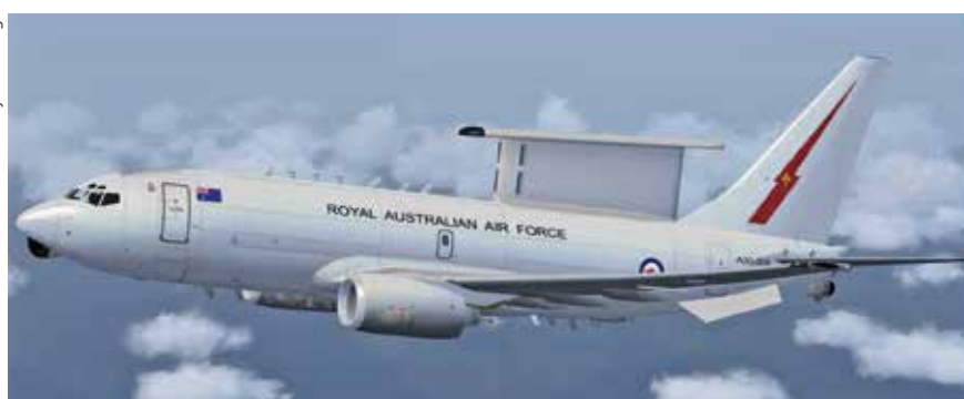
The E7A WEDGETAIL flown by the Royal Australian Air Force is a twin-engine airborne early warning and control aircraft based on a Boeing 737. It is lighter than the E-3 SENTRY and mounts a fixed, active electronically scanned array radar instead of a rotating one.
