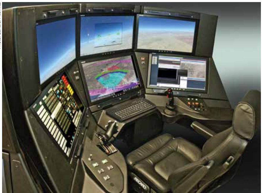
An example of an advanced workstation for RPA operators
