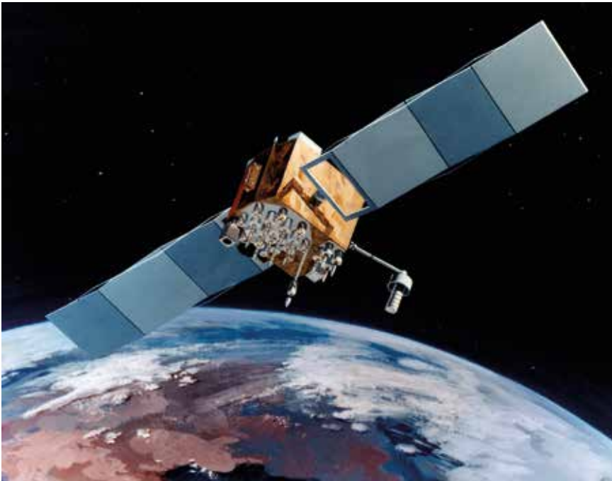
Navstar-2F satellites were among the first to transmit the new M-code GPS signal.
