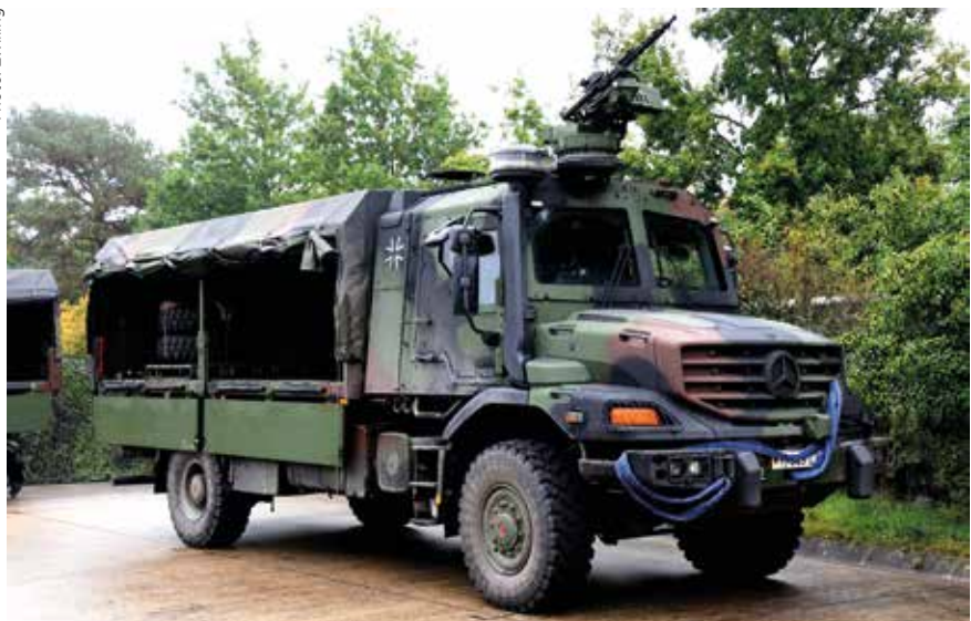
FLW remote-controlled weapon station on a ZETROS protected transport vehicle
