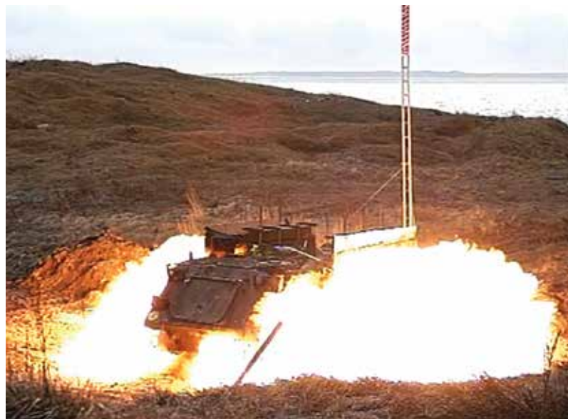
The Active Blast Countermeasure System undergoing tests
