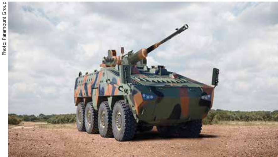
The 8x8 version of the MBOMBE armoured vehicle from the Paramount Group of South Africa was displayed in Kazakhstan in June mounting the Russian AU-220M BAIKAL unmanned turret system. This has a 57x347SR calibre cannon, originally used in the S-60 anti-aircraft system, that offers significant performance against both hard and soft targets.
