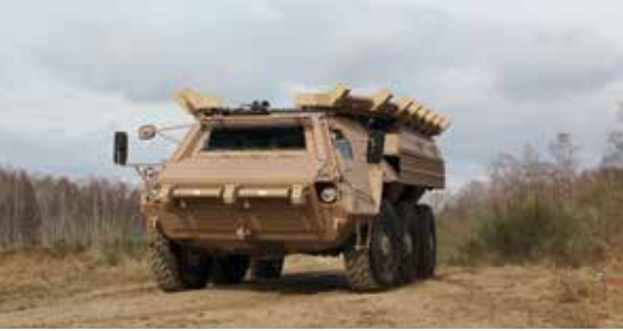
Active Defence System (ADS) from IBD Deisenroth/Rheinmetall on the FUCHS armoured transport vehicle
