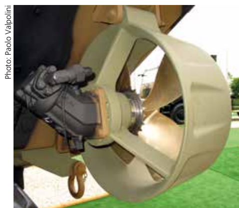
A close up of the Iveco DV ACV 1.1 prototype showing the serrated disk located on the propeller hub to clear it from possible entanglements
