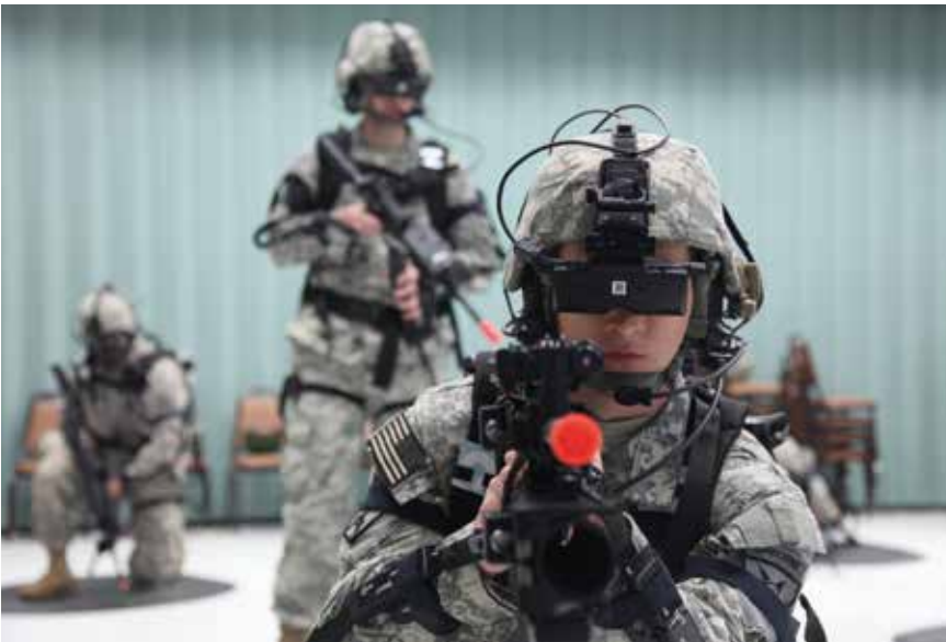
The Dismounted Soldier Training System (DSTS), a virtual reality trainer at Fort Leonard Wood. The DSTS translates soldiers' movements into a simulated training environment where soldiers can conduct foot patrols and clear buildings.
