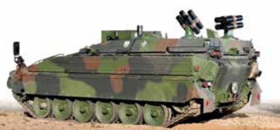
AvePS (Active Vehicle Protection System) is a launcher-based protection system, shown here on a MARDER AIFV.
