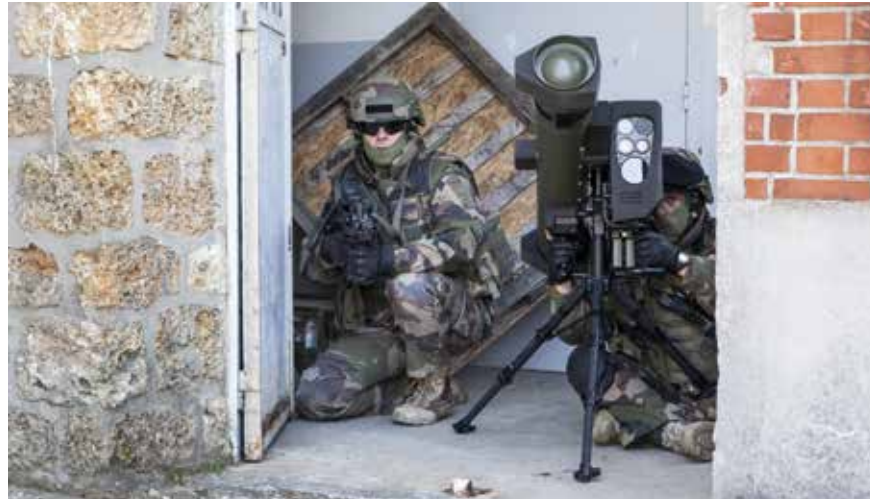
Like many modern antitank missile systems, the MBDA Missile Moyenne Portée (MMP) uses a soft-launch technique that allows a missile to be fired from inside buildings or bunkers. Once the missile has cleared the launch-tube and flown a safe distance from the launcher, the main motor then ignites.
