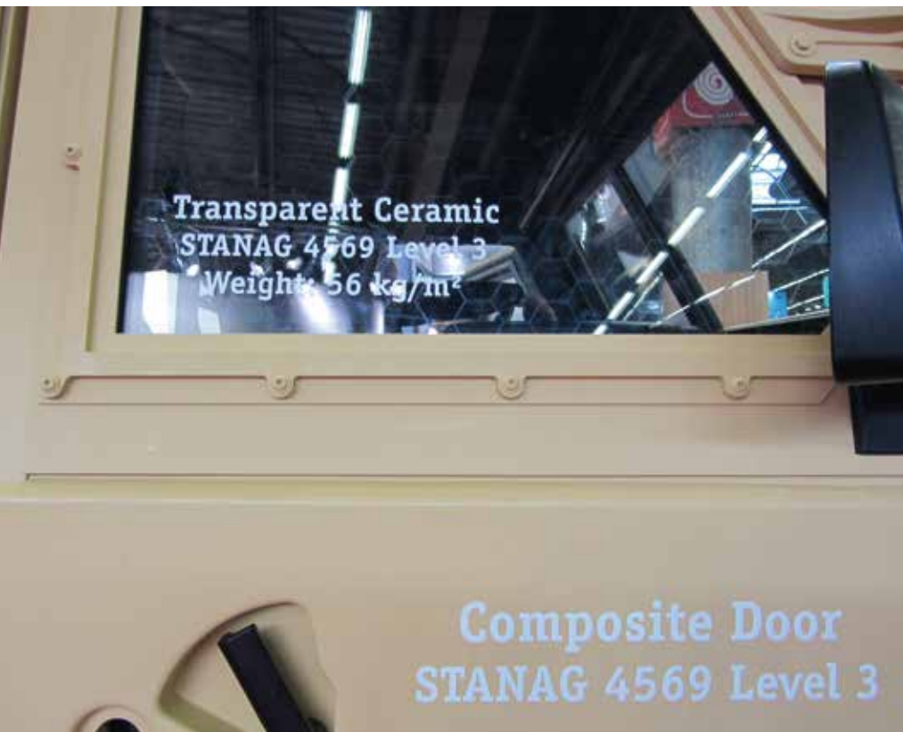
Level 3 transparent protection on a vehicle door
