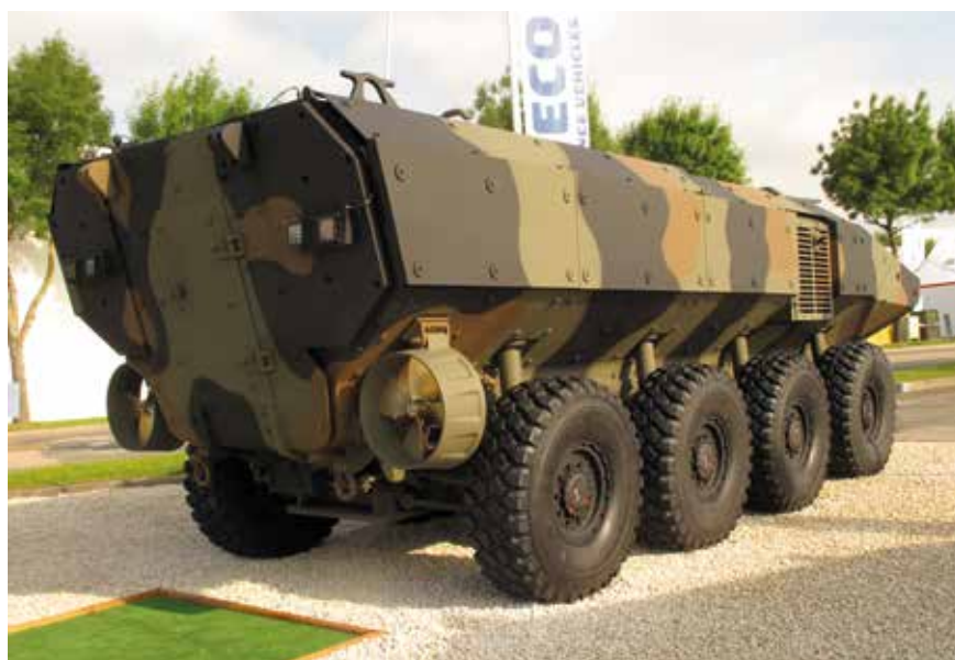
The BAE Systems/Iveco DV contender for the AVC programme is heavily based on the original Iveco DV SuperAV.
