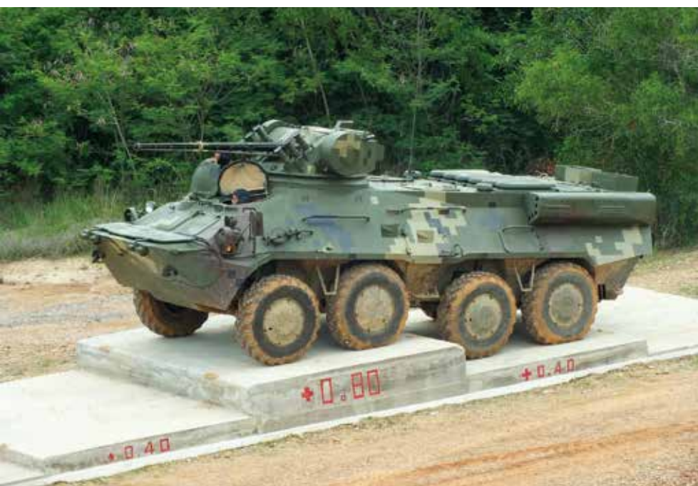
A KMDB BTR-3E1 of the Royal Thai Army (RTA), equipped with a SHKVAL Overhead Weapon Station (OWS). This mounts a 30 mm ZTM-1 cannon, 7.62 mm coax, 30 mm AG-17 AGL and two SKDB Luch BARYE anti-tank missiles. The SHKVAL is being offered as the turret solution for a new BMP-1 upgrade being proposed by Ukrainian industry.
