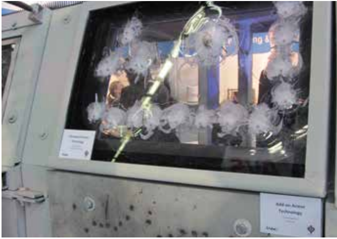
Transparent protection system after multiple engagements
