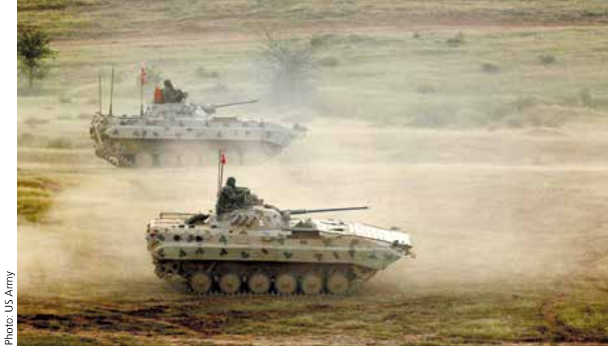
Indian Army BMP-2 vehicles on exercise. Uralvagonzavod produced 14,000 BMP-2 vehicles in the 1980s, with the vehicle also produced in the then Czechoslovakia, and still in production in India as the SARATH. The 2A42 30x165mm cannon of the BMP-2 is reaching its limits these days, opening the way for future potential BMP-2 turret upgrades.
