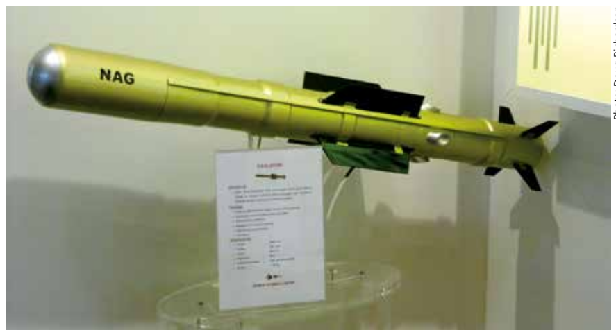
The basic version of India's NAG antitank missile is fitted with a nose-mounted imaging infrared seeker.
