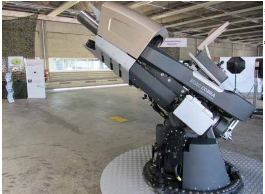
The electrical drive of the COBRA makes the system highly accurate, while ballistic computing enables MRSI firing (Multiple Rounds Simultaneous Impact).
