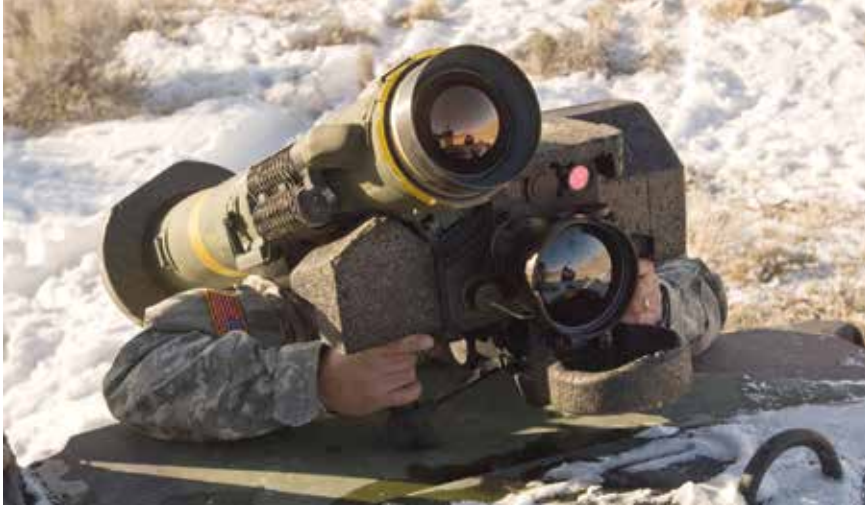
A ready-to-fire JAVELIN system consists of a sealed launch-tube attached to a Command Launch Unit (CLU) incorporating a daythermal sight.
