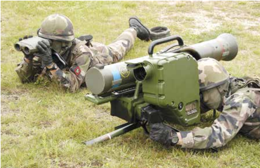
The MILAN ADT firing post was developed for the MILAN ER (Extended Response), a system developed by MBDA for use by armed forces that do not require a fire-and-forget antitank weapon.
