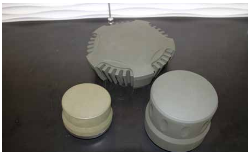
As this US Army photograph of various types of “smart” controlled-reception pattern antennas shows, these are small units that can easily be substituted for normal omnidirectional antennas.
