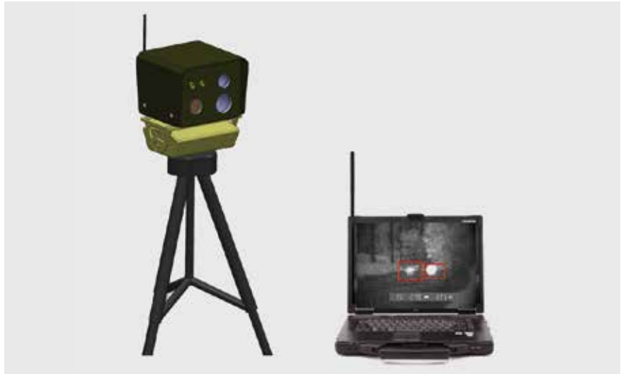
The artwork on the left shows the planned configuration of the Ukrainian Advanced Research Project Agency's sniper-detection system. The image on the monitor screen on the right shows how laser energy striking the lens of an enemy optical system produces a visible 'bloom'.
