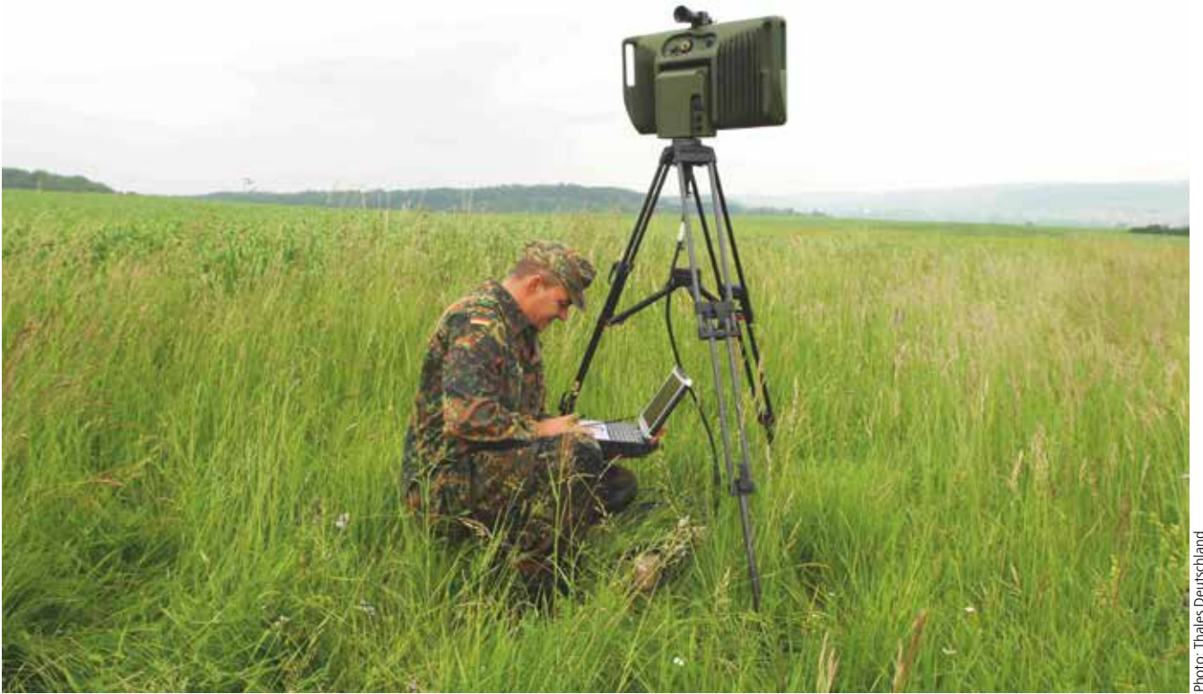
The GROUND OBSERVER 12 of Thales Deutschland can be manpacked by a single soldier, and has a setup time of less than two minutes.
