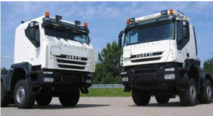
Comparing the size of transparent surfaces of unprotected (right) and protected (left) cabs of a logistics vehicle from Iveco
