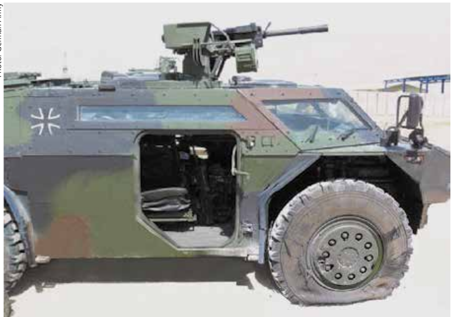
FENNEK scout vehicle after RPG 7 hit
