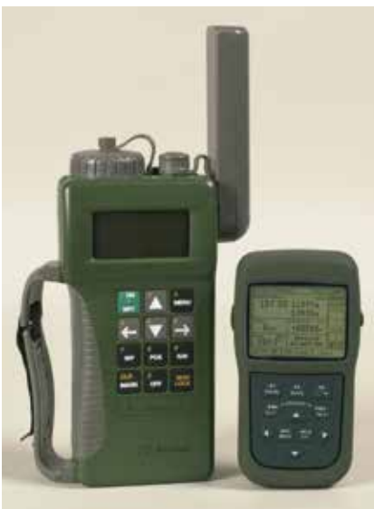
As with most types of electronic hardware, the size and weight of hand-held GPS receivers shrink from generation to generation. The ANIPSN-11 Precision Lightweight GPS Receiver (PLGR) seen on the left towers over the later ANIPSN-13 Defense Advanced Global Positioning System Receiver (DAGR).
