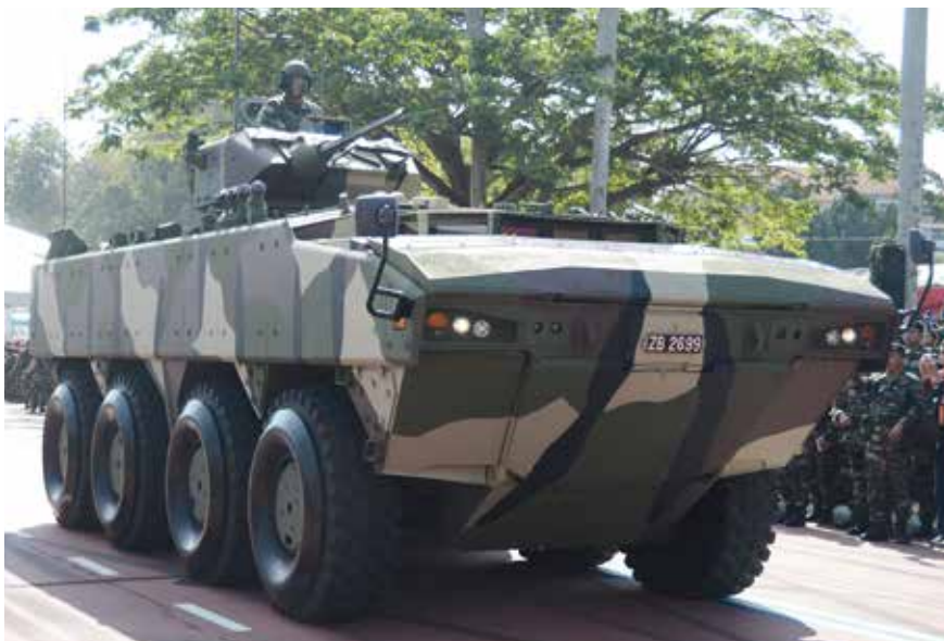
Malaysia is producing the AV8 (the first prototype is shown here); a development of the PARS 8x8 from FNSS.
