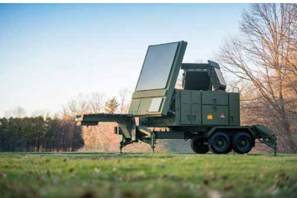
Raytheon's GaN-based PATRIOT AESA radar with a 360-degree capability
