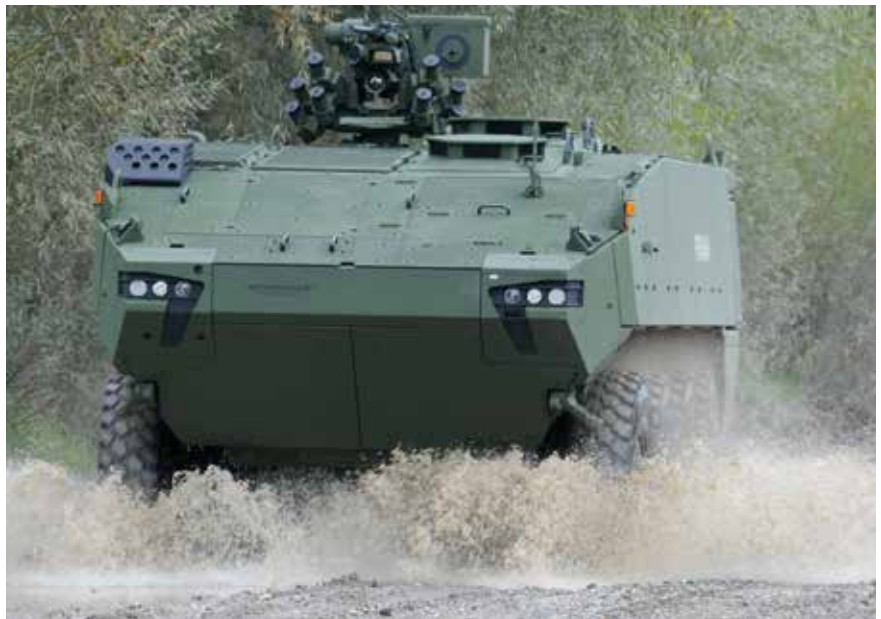
The infantry version of the PIRANHA V will get a remotely controlled weapon station.
