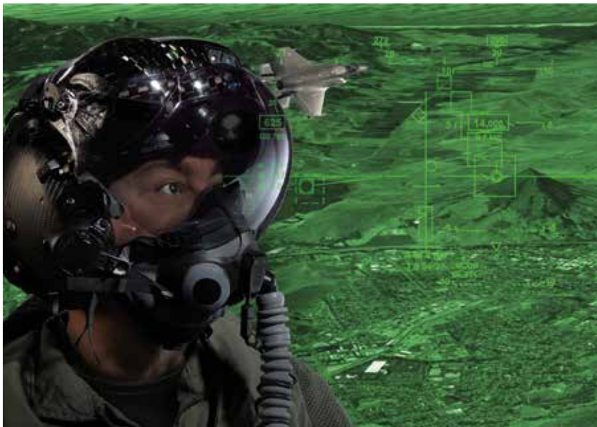
Use of this Rockwell Collins generation III Helmet Mounted Display System (HMDS) to present extensive symbology and other data to the pilot removes the need for the F-35 to have a Head-Up Display (HUD).
