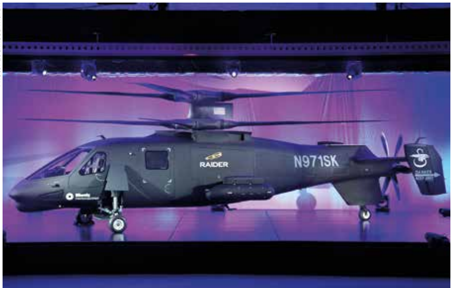
The Sikorsky S-97 RAIDER concept for a multi-mission helicopter first flew in 2015 and is considered a potential successor for USSOCOM’s MH-6 LITTLE BIRD. The SB-1 DEFIANT participating in the JMR-TD is based on the S-97, but heavier. Note the coaxial rotor system and pusher propeller.
