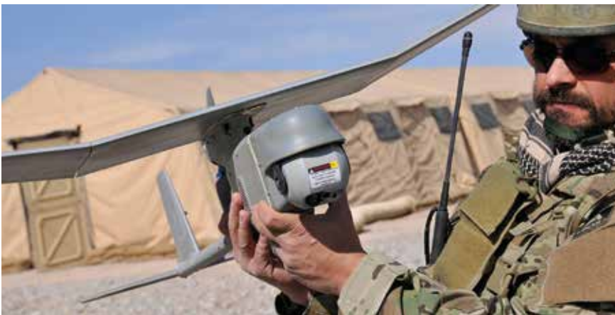
AeroVironment's RAVEN can be launched right from the hand of the soldier.
