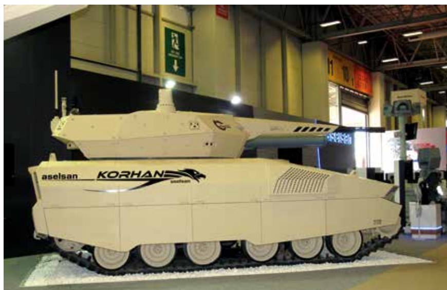
Aselsan exhibited the KORHAN turret armed with a 35 mm cannon, this calibre being apparently the one of choice for the future Turkish Army IFV.
