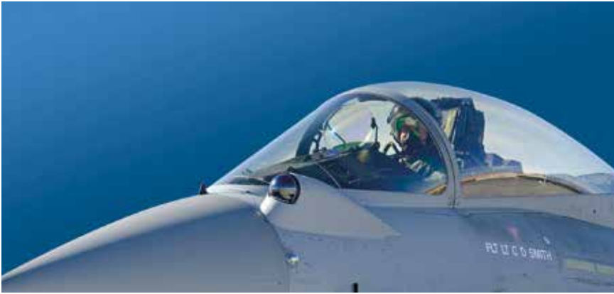
This air-to-air close-up of the Eurofighter TYPHOON shows the housing for the EUROFIST PIRATE EO system, and gives a good view of the BAE wide-angle HUD.
