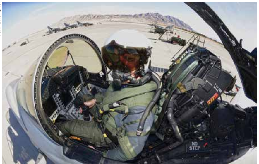
The multifunction displays in the Eurofighter TYPHOON cockpit are of the conventional pattern incorporating an array of push buttons.
