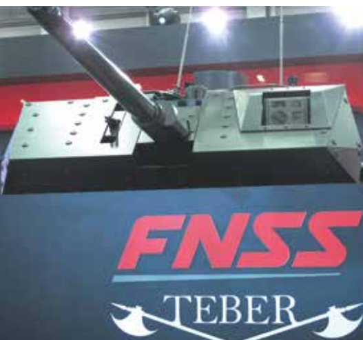
The prototype of the TEBER turret in the two-man version; armed with a 30 mm cannon, it can host also a bigger calibre weapon.
