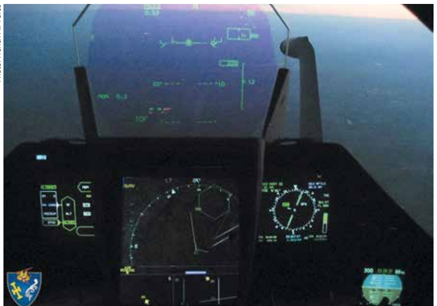
View of a RAFALE cockpit showing the symbology of the HUD and the infinity-collimated Head-Level Display
