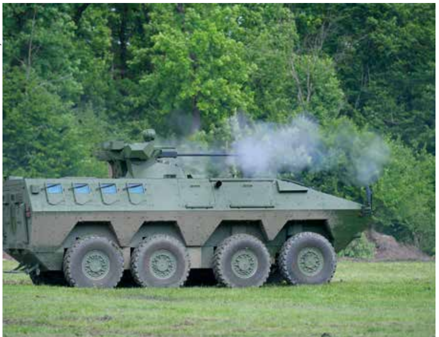
The LAZAR II and III Light Armoured Vehicles (LAV) are being acquired by the Serbian Army. Weapon options include a turret-mounted 30 mm cannon or a machine gun mounted in a Remote Control Weapon Station (RCWS). Serbia intends to purchase large numbers of LAZAR vehicles.
