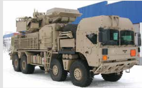
The modular layout of the PANTSIR-S1 ADMGS allows for its integration with different chassis of both Russian and foreign origin.
