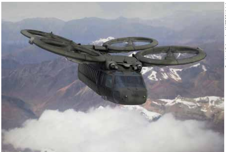
An artist’s conception of future army rotorcraft using ducted fans rather than conventional rotor systems
