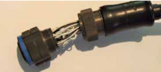
Mil c 38999 connector showing good harness practise of repair loops and a boot termination
