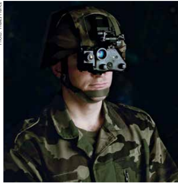
Thales France's MINI-DIIR is a clip-on attachment for the company's MINIE-D (Miniature Night Intensified Equipment - Display). The combination provides a fused thermal and I2 image.
