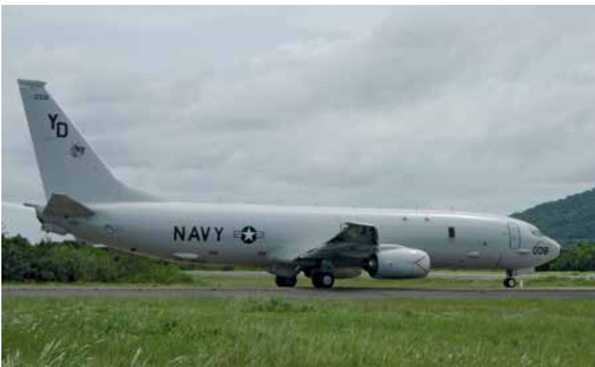
In the US the P8 POSEIDON replaced the P3 ORION. The POSEIDON is derived from the Boeing 737 NG airliner.
