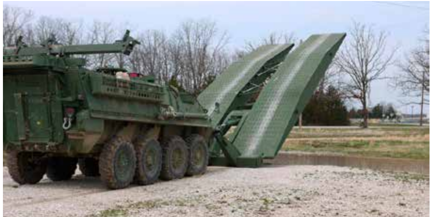
Pearson Engineering has developed an AVLB carried by the General Dynamics Land Systems 8x8 STRYKER M1132 Engineer Squad Vehicle (ESV).
