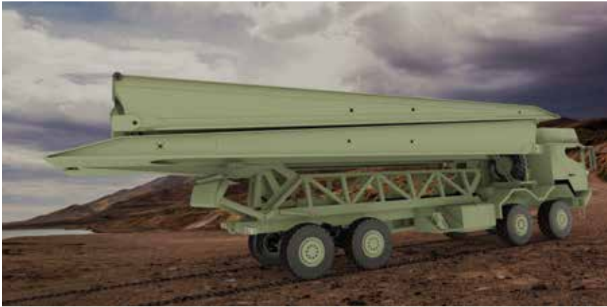
The MLC 80+ classification ANACONDA can support the latest and heaviest variants of the LEOPARD 2, M1A2 ABRAMS and CHALLENGER 2.
