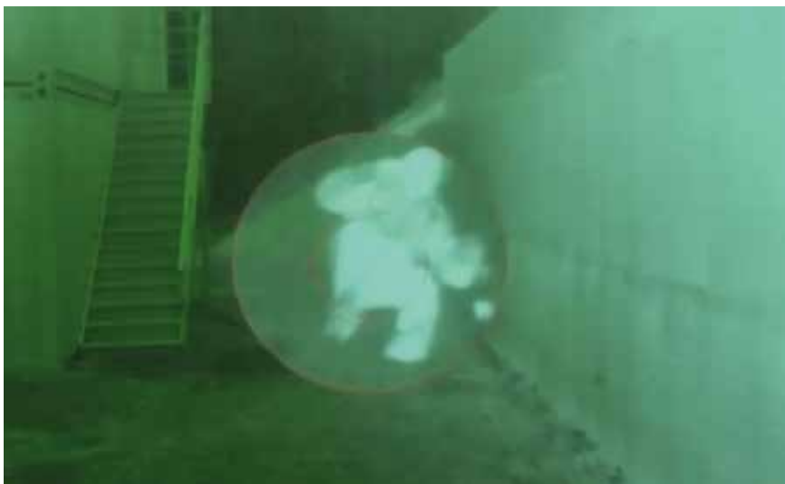
Imagery from the FWS-I weapon sight can be displayed as an overlay in the output of the ENVG III night-vision goggle.
