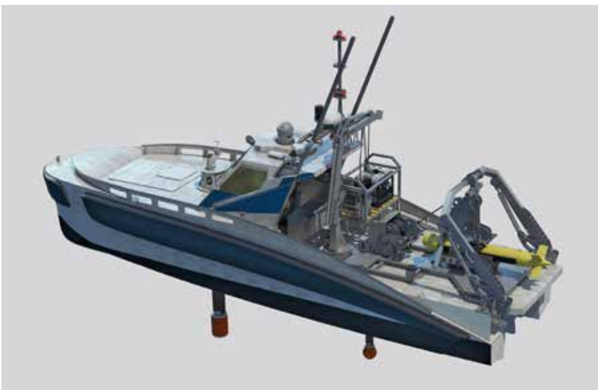
Israel's Elbit Systems has developed the SEAGULL USV. In addition to Mine Countermeasures, the USV can be used for anti-submarine warfare.
