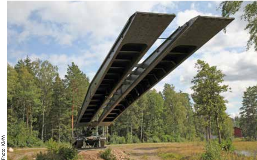
The LEGUAN AVLB is based on a LEOPARD 2 chassis.
