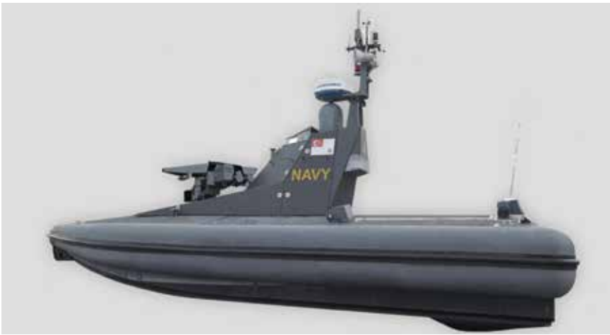
The PROTECTOR USV is an unmanned integrated naval combat system, based on a rigid hull inflatable boat. It has a complete sensor, navigation and weapon suite and can be remotely controlled from shore or from ships at sea.
