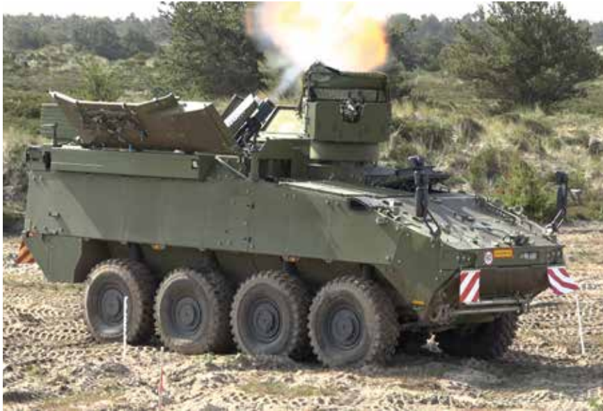
PIRANHA 5 with integrated CARDOM 10 during firing tests. The three crew members are well protected inside the vehicle while operating the mortar. The crew includes the commander and a driver.
