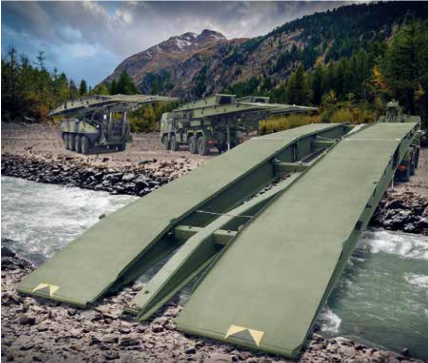
PYTHON is a lightweight, aluminium, dry-gap bridge offering a tactical 13m gap-crossing capability.
