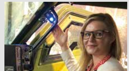
Installed map reading light in a protected vehicle
