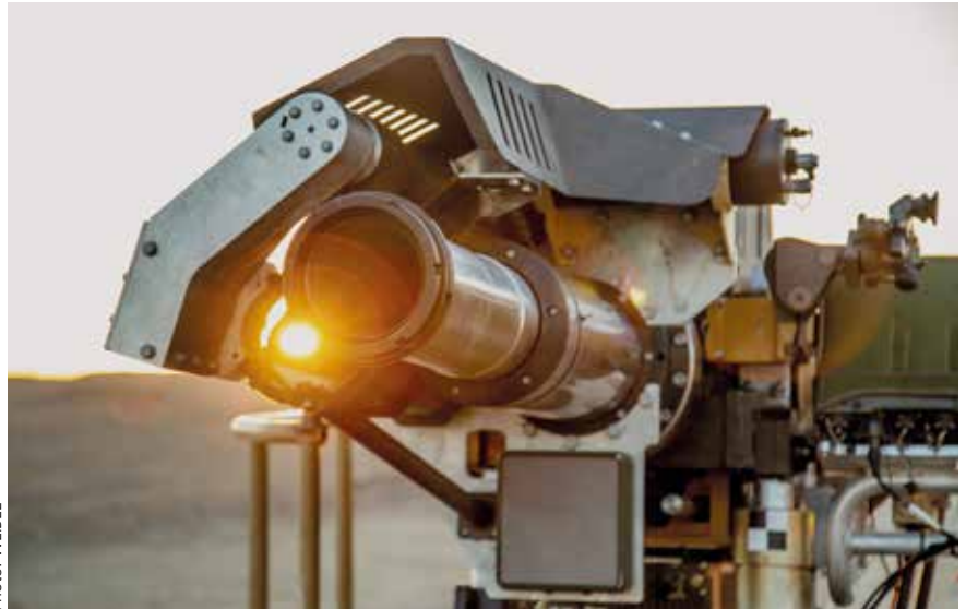
The CARDOM 10 prototype with the MVR-700SC positioned underneath the barrel
