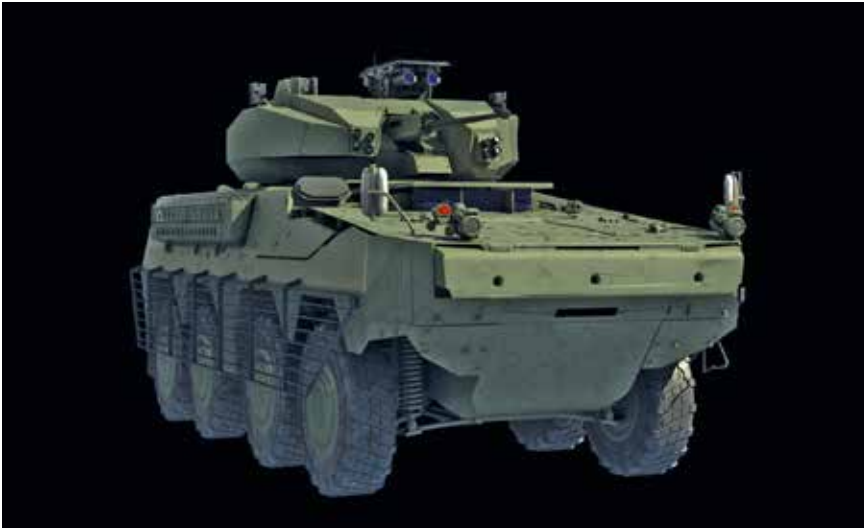
RAFAEL's SAMSON 30MM remote-controlled weapon station with SPIKE and the TROPHY active protection system
