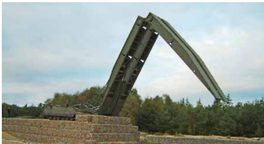
The TITAN AVLB in use with the British Army is based on a CHALLENGER 2 chassis.
