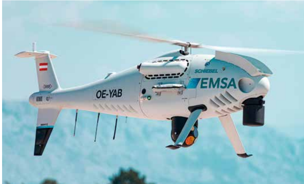
The CAMCOPTER® S-100 navigates automatically via pre-programmed GPS waypoints or can be operated directly with a pilot control unit.
