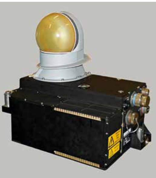
The Leonardo SKYWARD family of IRST for both combat manned aircraft and unmanned platforms
