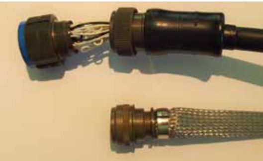
Mil c 38999 connector with repair loops and boot termination (above) together with a stainless steel braid termination to a back shell (below)
