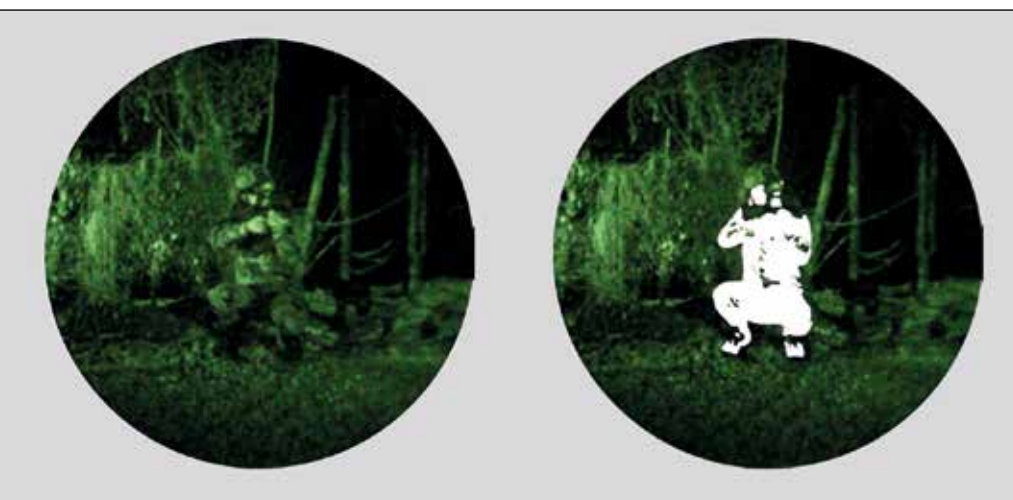
A decamouflage mode allows the MINI-DIIR to highlight potential targets.
