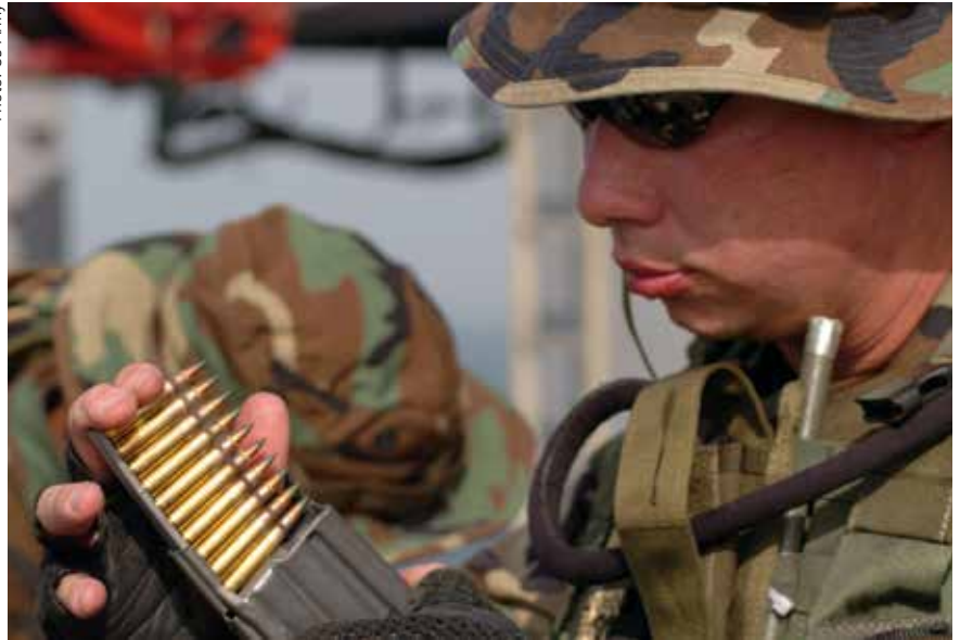
Using a stripper clip to load M885 5.56mm ammunition into an M-16 magazine
