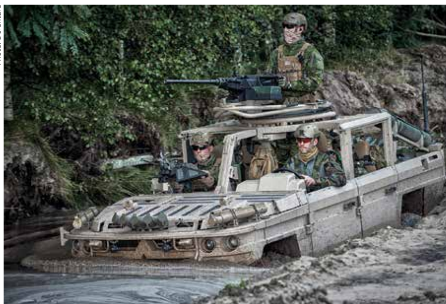
The ATTIVECTOR has a deep fording capability of up to 840mm.
