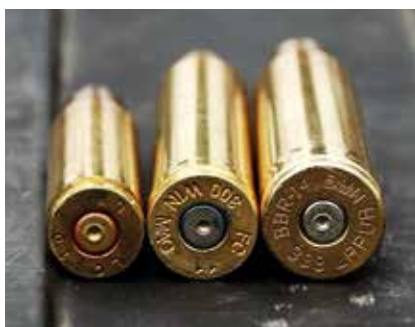
From left to right, the 7.62mm NATO, .300 Winchester Magnum, and .338 Lapua Magnum rounds before a 2016 evaluation to inform Marine Corps acquisition leaders about future Marine sniper weapon system requirements. Marine Corps snipers conducted the test using different rifles at distances ranging from 900 to 1,500 metres to target.
