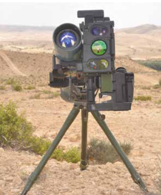
Head-on view of the RAFAEL SPIKE MR with missile on the left and optical package and gunners sight on the right
