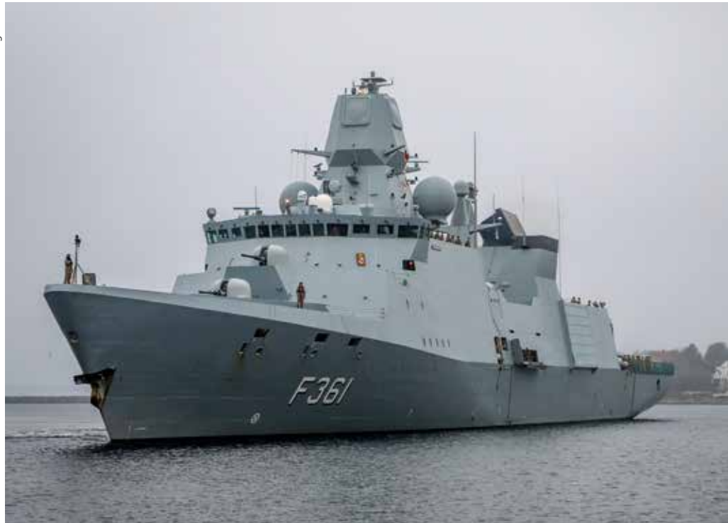
From 2012, three 6000 tonne AAW frigates of the IVER HUITFELD class were introduced.
