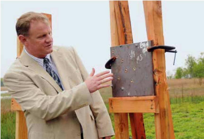
Comparison of the effectiveness of the Army's 5.56mm M855A1 Enhanced Performance Round fired from an M4 Carbine against a 3/8 inch mild steel plate, versus the performance of a 7.62mm M80 round fired from an M14, during a test fire event at Aberdeen Proving Ground, May 4, 2011. The M855A1 round penetrated the plate at 300 metres; the M80 (which was replaced by the upgraded M80A1 in 2014, did not.
