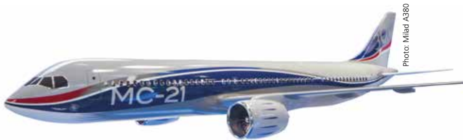
The Irkut MC-21 is a single-aisle twinjet airliner, developed by the Yakovlev Design Bureau and produced by UAC. Its name translates as "mainline aircraft of the 21st century".
