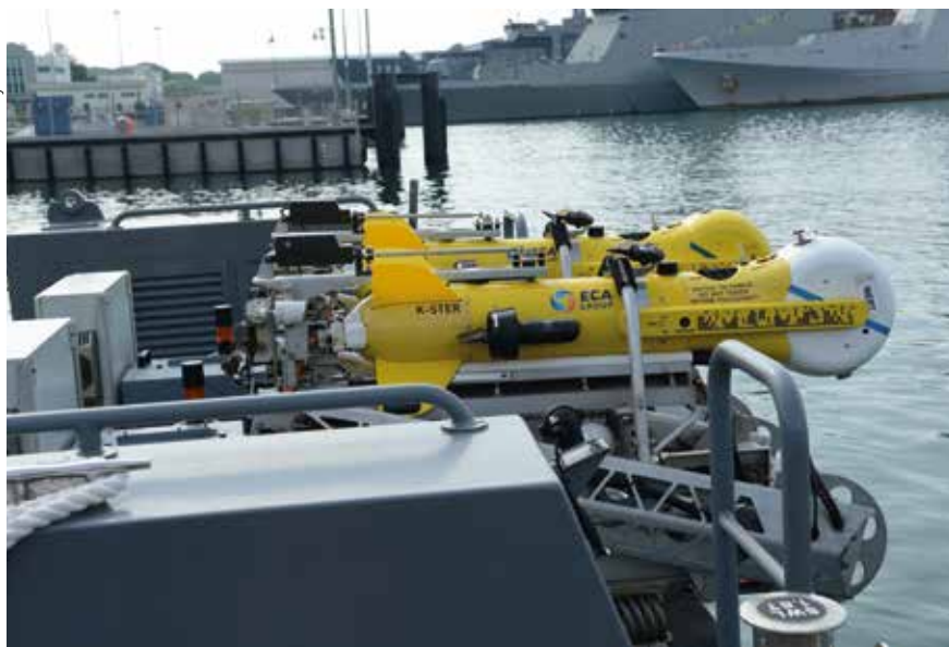
One of the RSN's VENUS 16 USVs with two Expendable Mine Disposal Systems onboard
