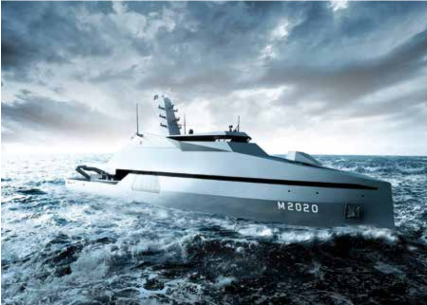
Abeking & Rasmussen can offer the APEX PROTECTOR MCMV with a non-magnetic steel hull.
