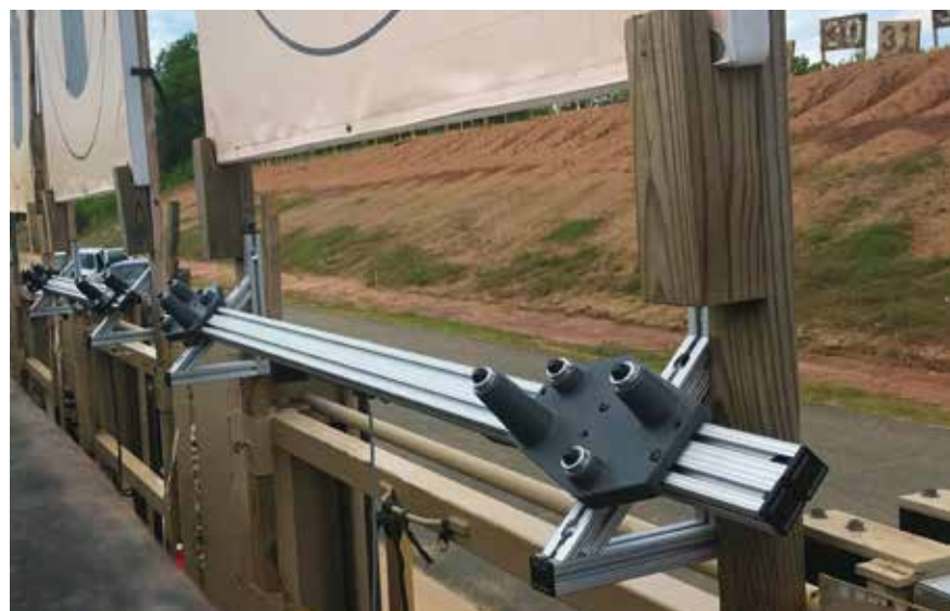
Meggitt's LOMAH (Location of Miss and Hit) system gives instant feedback at the student station; shooters receive immediate results.
