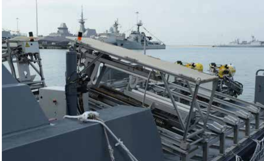
The racks to store the ECA K-STER Inspection and EMDS ROVs onboard a VENUS 16 USV
