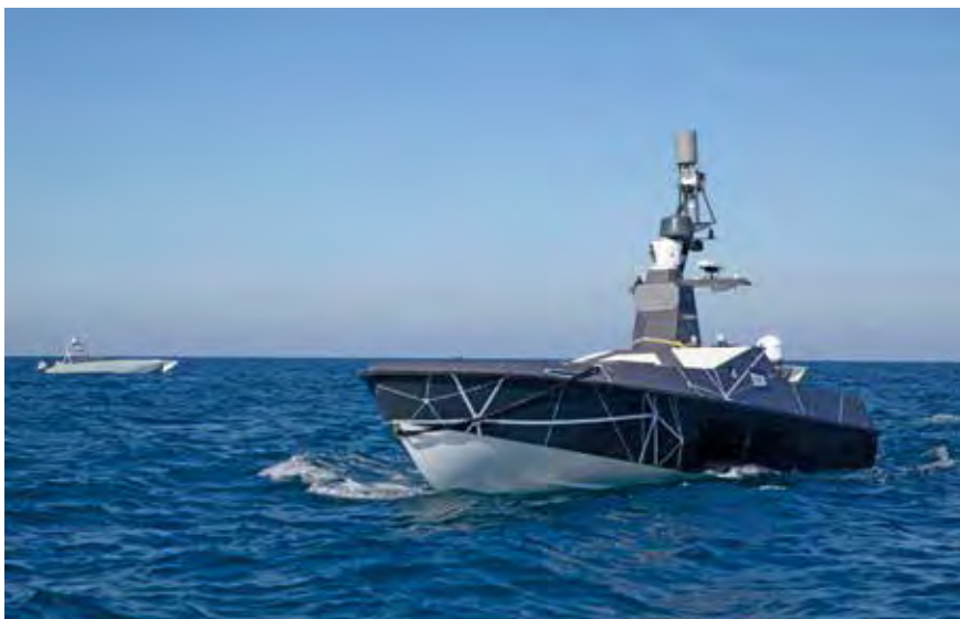
The Royal Navy's MAST-13 USV (foreground) pictured during an international exercise. The later MADFOX USV is derived from this design.
