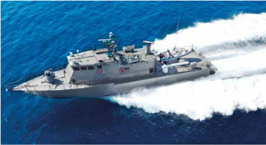
The SHALDAG Mk 5 is the largest of the well-established SHALDAG series of fast patrol boats.
