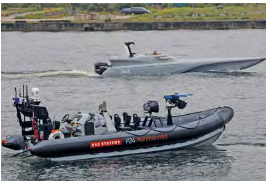
The Royal Navy's NavyX experimentation unit is now trialling an autonomous PACIFIC 24 rigid inflatable boat to understand how these might be used by future Type 26 and Type 31 frigates.
