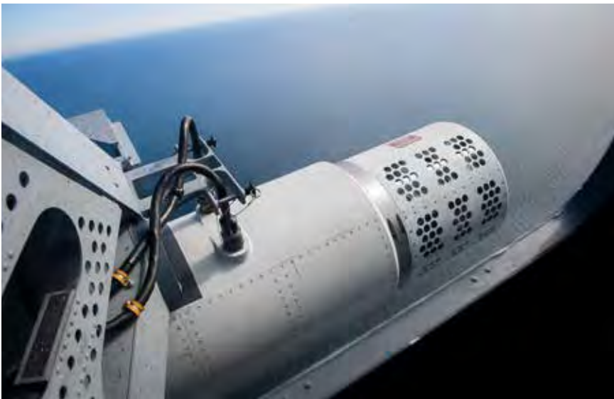
The ALMDS pod, which collects laser data for initial and requisition mine sweeping missions, attached to an MH-60S SEA HAWK helicopter
