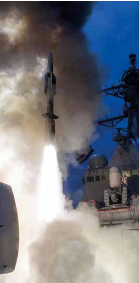
The guided-missile destroyer JOHN PAUL JONES (DDG-53) launches a Standard Missile (SM) 6 during a live-fire test of the ship's AEGIS weapons system. The multi-role missile's capabilities include the provision of defence against hypersonic weapons and ballistic missiles in their terminal phases.
