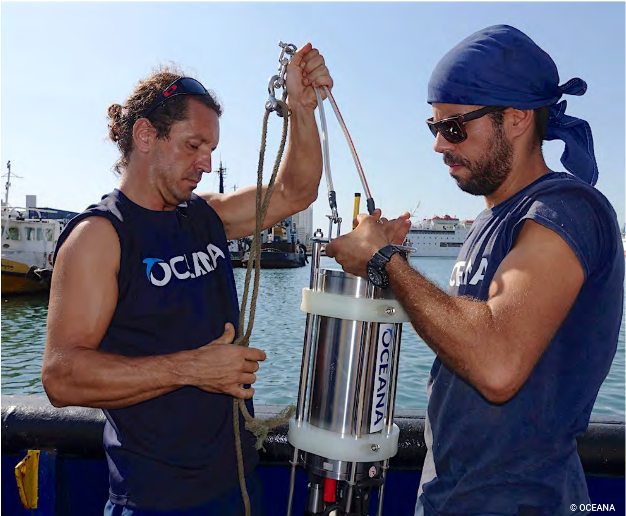
Figure 20. CTD sensors for water column analysis
