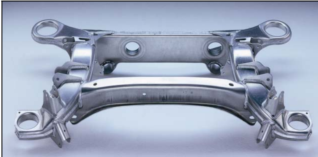
Rear axle subframe of the Mercedes S class Source: Hydro Aluminium Rolled Products
