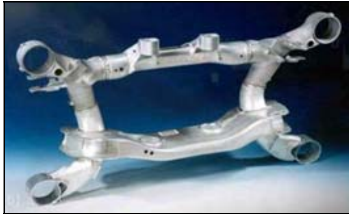
Aluminium rear axle subframe of the BMW 7 series Source: Hydro Aluminium Rolled Products
