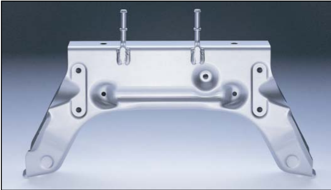
Front axle subframe of the Volkswagen “3 litre” Lupo Source: Hydro Aluminium Rolled Products
