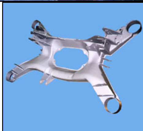
Aluminium rear axle subframe prototype consisting of a sheet stamping and a single casting (below, bottom view) Source: Hydro Aluminium Rolled Products
