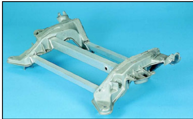
Rear axle subframe made from straight extrusions and thixo-cast components, produced for the Alfa Romeo Spider Source: Constellium
