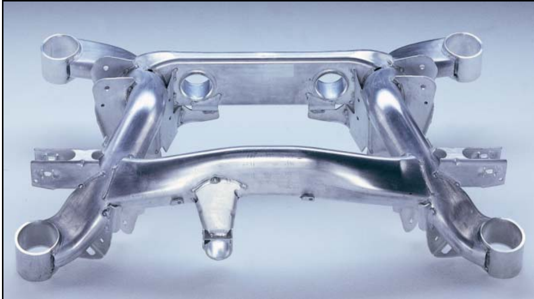
Rear axle subframe for BMW 5 series models Source: Hydro Aluminium Rolled Products
