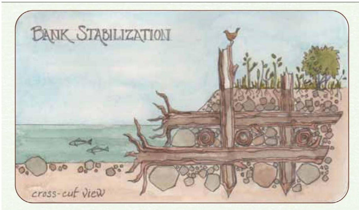
FIGURE 13. BANK STABILIZATION EXAMPLE GRAPHIC
