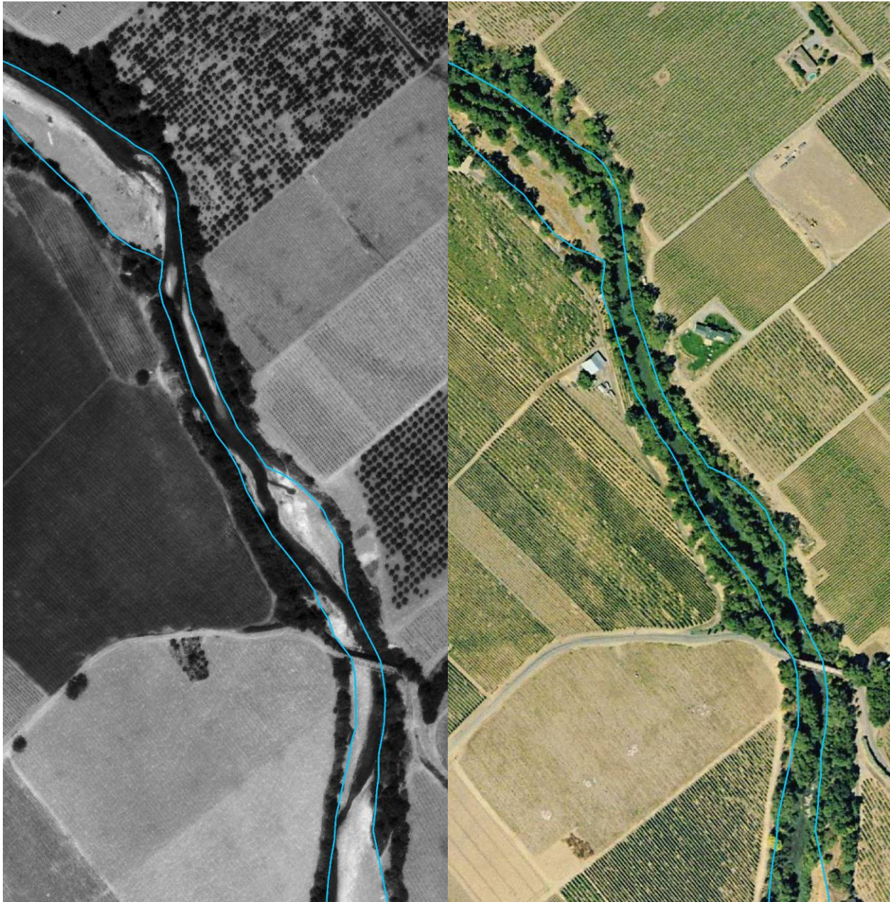
Figure 2: Example of vegetative narrowing of channel corridor near Lambert Bridge (RM 6.6). Lambert Bridge is seen at lower right of each frame. Dry Creek flow is from top to bottom. Left frame is from 1976, right frame is from 2004. Light blue line is estimated limit of active fluvial features in 1976.
