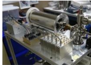
L10 with inner magnetic shield installed.
