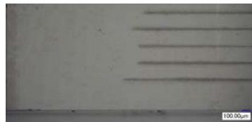
Fig. 2: Structural damage close to the output face of SLT SHG device left by 5 series of experiments.
