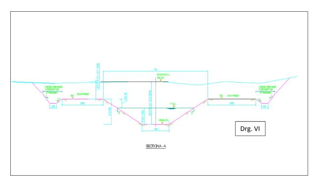
**Cross Section of Earthen Canal**
