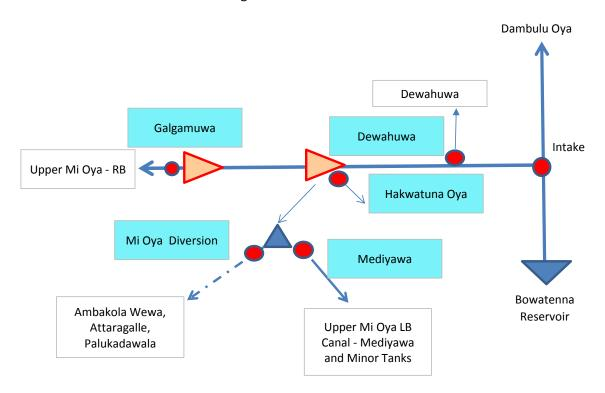
Figure 4-2 Main diversion points in NWP canal project
