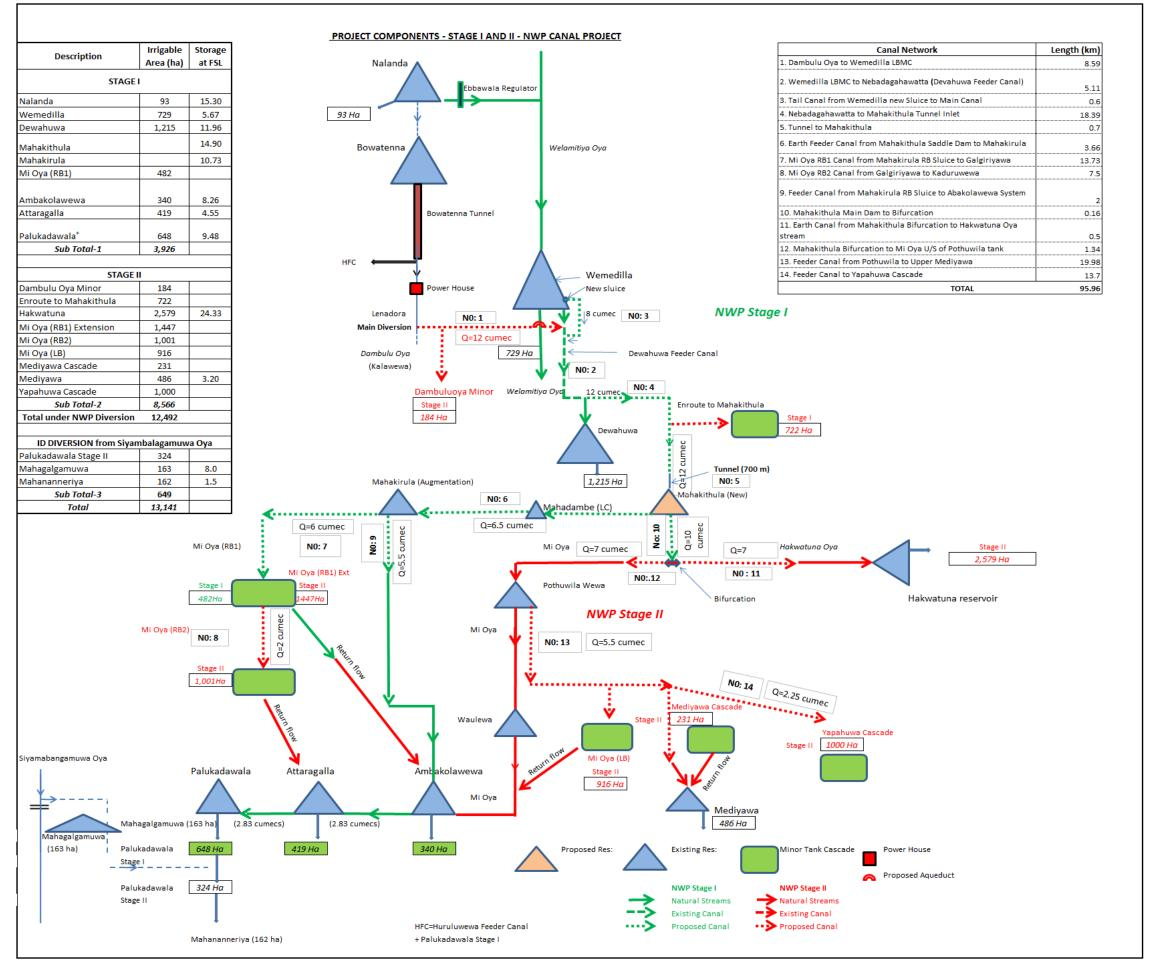
Figure 1-2 Project components - stage I and II
