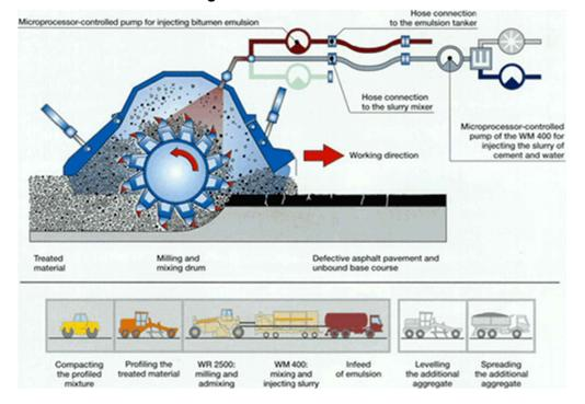
Figure 3: Schematic of FDR
