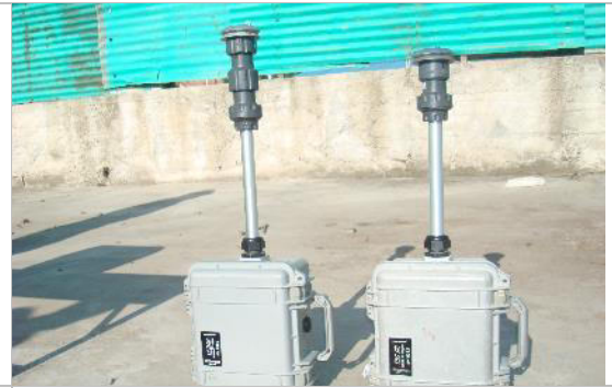
Low Volume Sampler and Weather Station at A4
